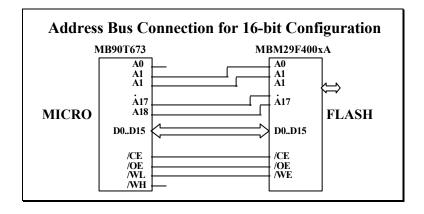
The important thing is, that the address line A1 of the controller is connected to A0 of the flash memory. The controller would need its A0 line only to address single bytes in an external memory, but since we configured our system to be 16-bit wide, the smallest unit the microcontroller can read is a 16-bit word. Note, that also the controller has to be configured such that it knows that the flash memory area is 16-bit wide.
