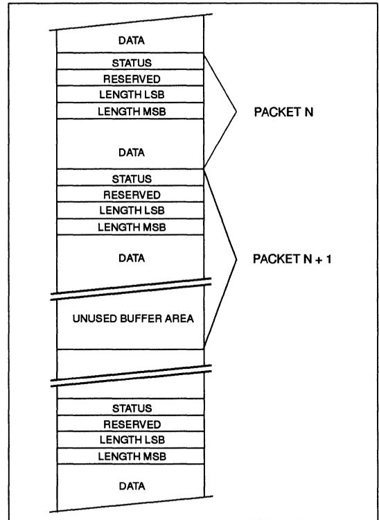
Figure 9. Receive Buffer Detail
