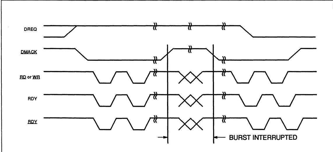
Burst can be interrupted by negating DMACK. Burst will resume when DMACK is reasserted.
