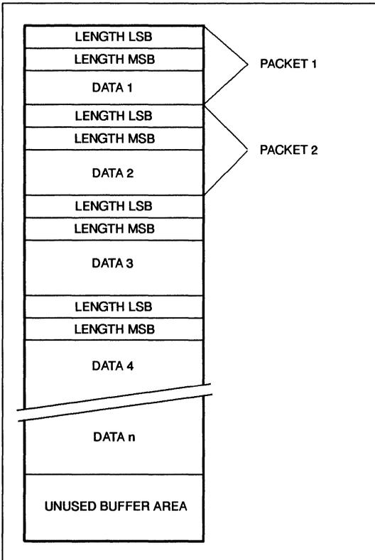
Figure 8. Transmit Buffer Detail
