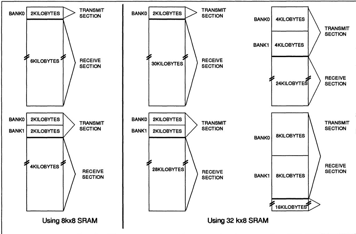
Figure 7. Transmit Buffer Configurations
