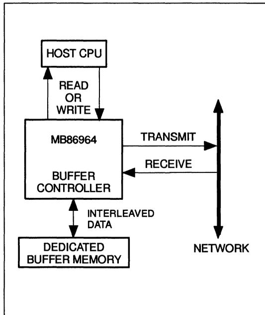
Figure 6. Simultaneous Access to Buffer Memory
