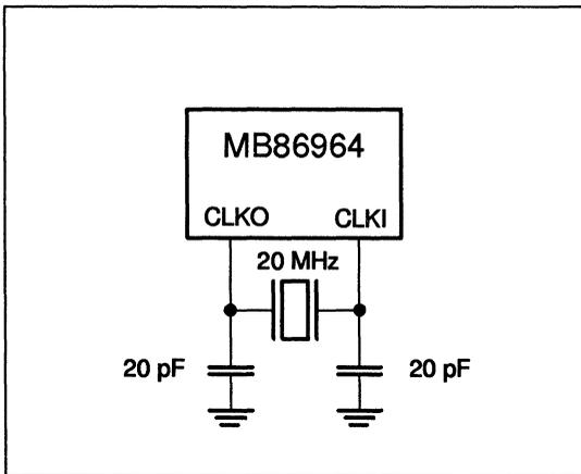
Figure 4. Crystal Oscillator Connection
