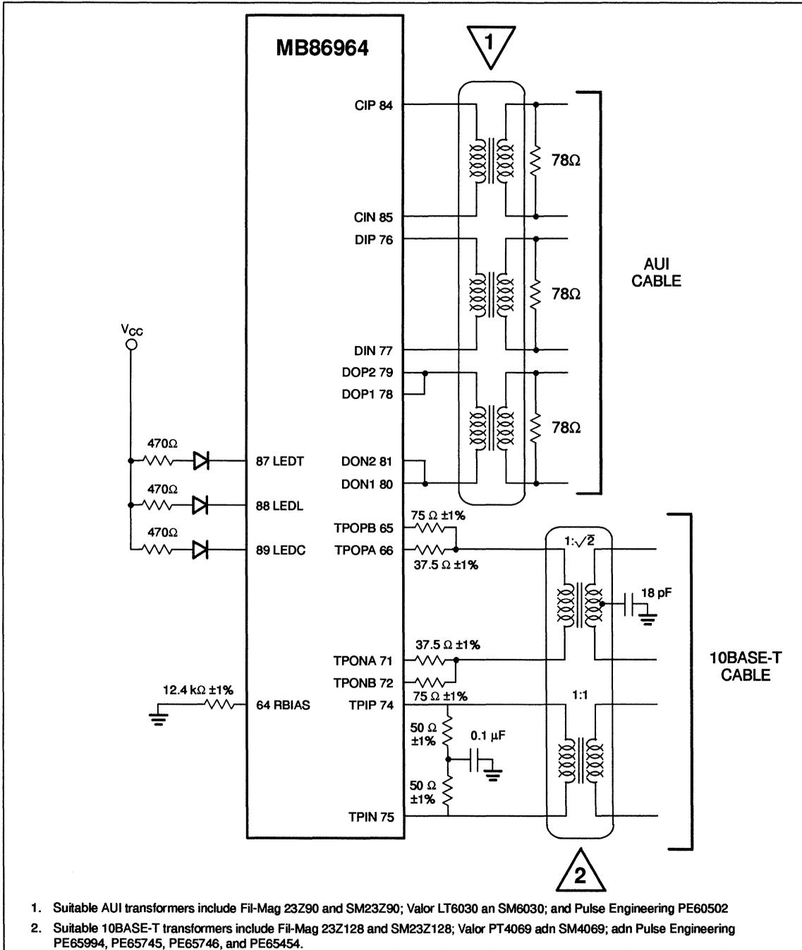
Figure 11. Typical TP Port and AUI Port Connections
