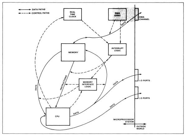
Fig. 2-12. Logical Functions of the 3854 DMA Device
