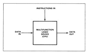
Fig. 2-1. Multifunction Logic Device
