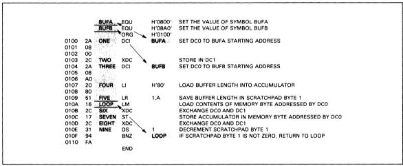
Fig. 4-2. Label Fields (Shaded) in a Source Program
