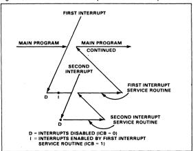
Fig. 8-2. Two Levels of Interrupt
