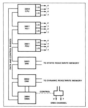
Fig. 2-5. F8 Microprocessor System Configurations
