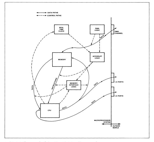
Fig. 2-4. Logical Components, Data Paths and Control Paths in any Microprocessor System
