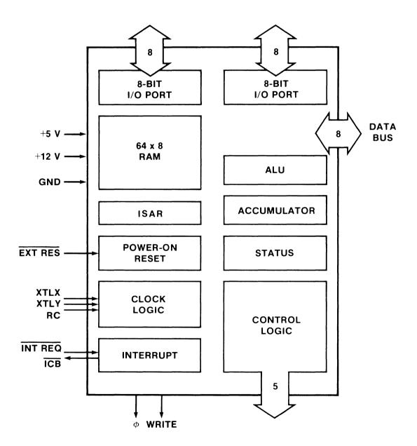
Figure D-1 F3850 Central Processing Unit (CPU)
