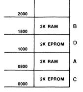
D) Switches E. H and A set. Jumper connections: E1 to E3, E2 open, E4 to E7, E5 to E6.
