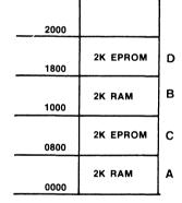
E) Switches E, H and A set. Jumper connections: E1 to E2, E3 open, E4 to E7, E5 to E6.
