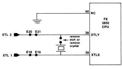
(b) Jumper connections for use with non-standard frequency or clock reference
