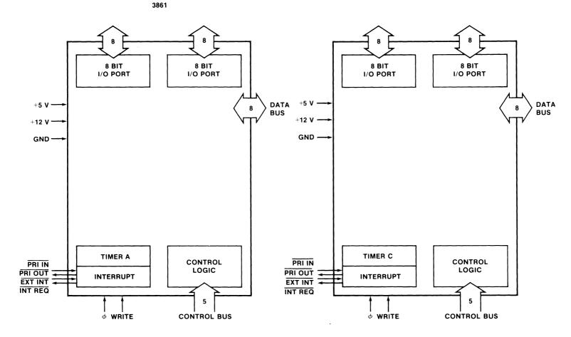
Figure D-4 F3861 Peripheral I/O Device (PIO)
