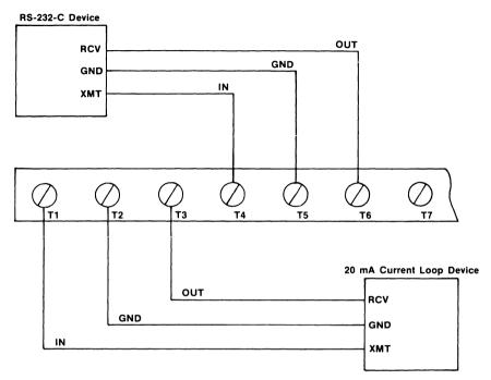
Figure 2-1 Connecting an External Terminal to the PEP System
