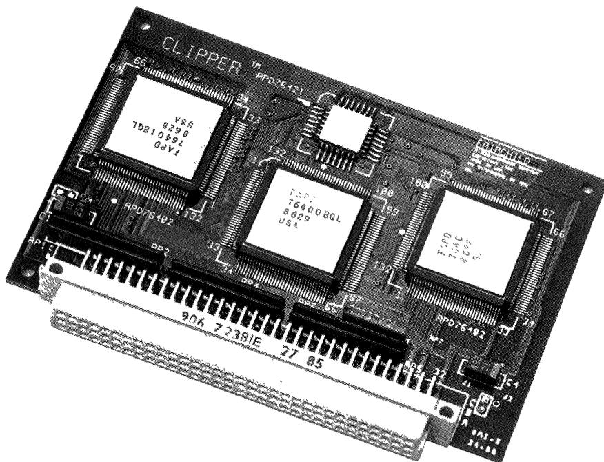
This document provides a comprehensive description of the CLIPPER 32-bit microprocessor module including a functional description, signal description, timing waveforms, module dimensions with connector pinout, and AC/DC parametric values. The CLIPPER module, as shown in the photograph above, contains three CMOS VLSI chips and clock circuitry implemented on a small multilayer printed circuit board.
