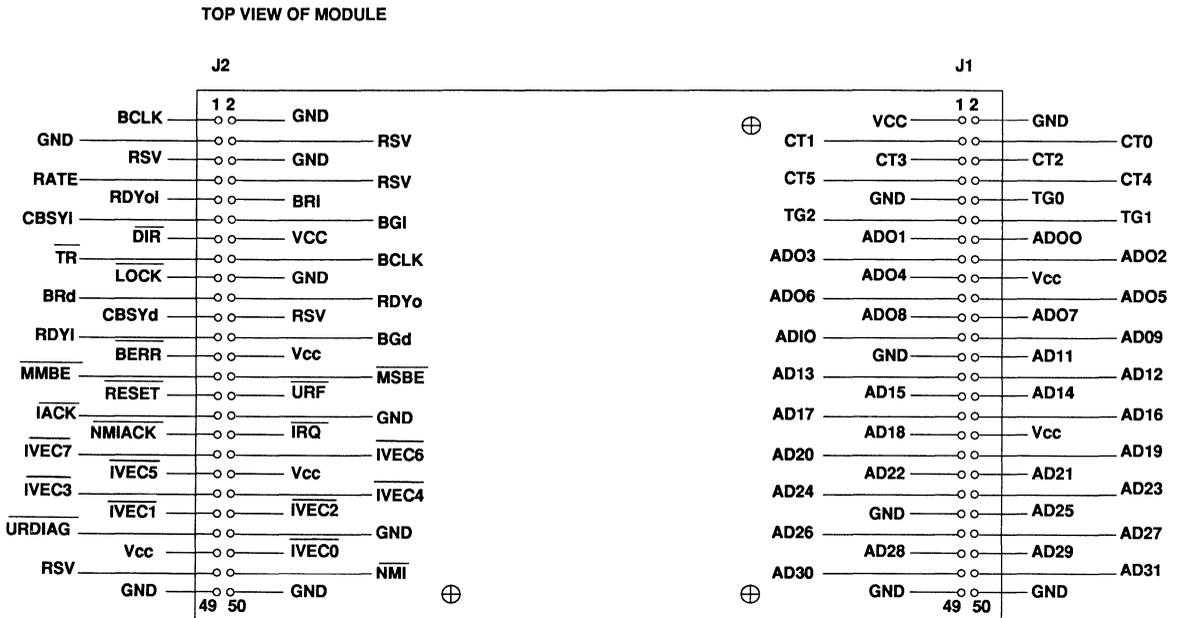
NOTE: PIN J3-8 SHOULD BE TIED TO BCLK (PIN J2-1) TO ENSURE COMPATIBILITY WITH FUTURE ENHANCED VERSIONS OF THE CLIPPER MODULE.
