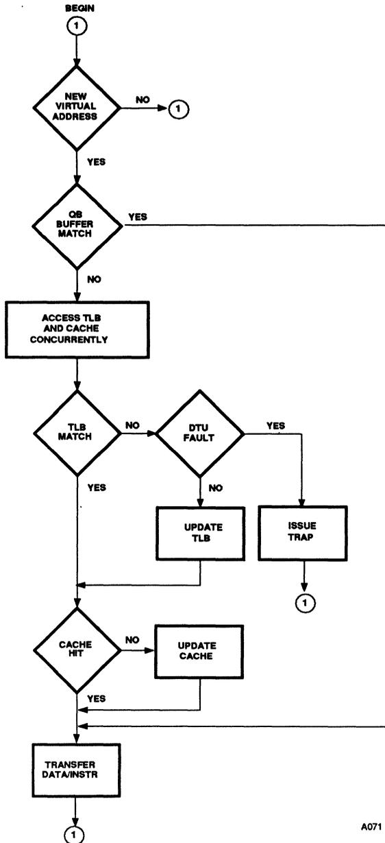
CAMMU operation begins when the CPU asserts a virtual address on the CPU-CAMMU address/data bus. The task of the CAMMU is to translate the CPU virtual address (bits <31:12>) into a real address and to use the translated real address to find the data.
