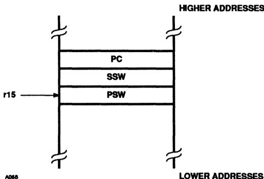
INTRAP uses V to obtain the new PC value and  $V + 4$  to obtain the associated SSW value. The new SSW value is transferred to the SSW, overwriting the previous contents of SSW except for the previous mode flag (P), which is retained in order to indicate the mode of the interrupted program. INTRAP then exits, and control is passed to the trap or interrupt service routine.
