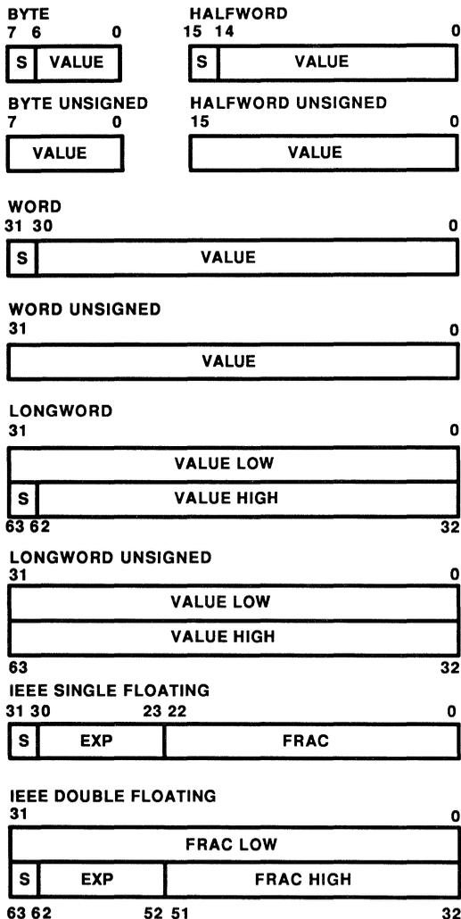
The rules for the storage and alignment of memory data types are illustrated in *Figure 7* and summarized below:
