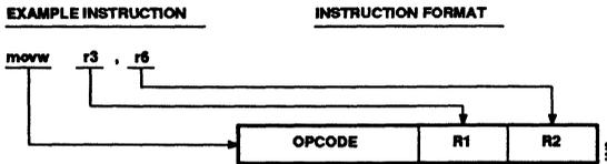
The opcode specifies the interpretation of the R1 and R2 fields. Usually the R1 field contains the source operand register number, and R2 contains the destination operand register number. For example, in the `movsw` instruction, the R1 field contains the number of the single-precision floating-point register containing the source operand, and the R2 field contains the number of the general register in which to store the result.
