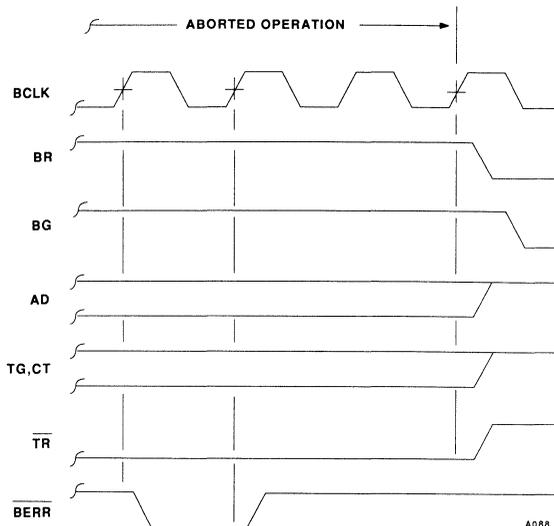
assertion of  $\overline{\text{BERR}}$ . The CPU should use the interrupt request to vector to a routine designed to resolve the bus error condition.
