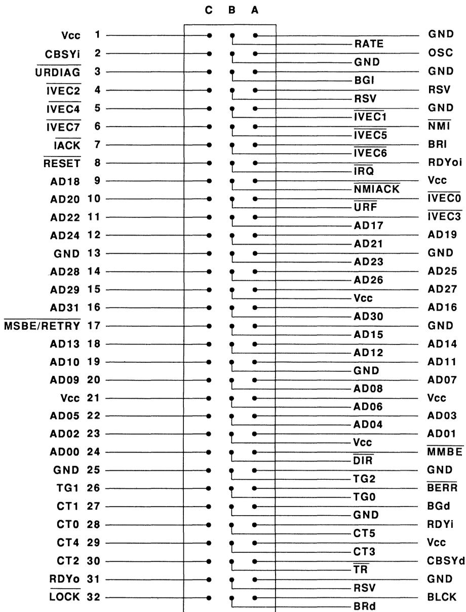
**NOTE:** Pin B31 (RSV) should be tied to pin A32 (BCLK) to ensure compatibility with future enhanced versions of the CLIPPER Module.
