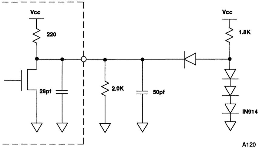
Figure 65 BLCK Output Test Load
