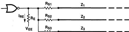
**c. Using Multiple Output Element for Load Sharing**
