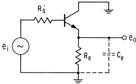
Fig. 1(a) Conventional AC Circuit of an Emitter Follower
