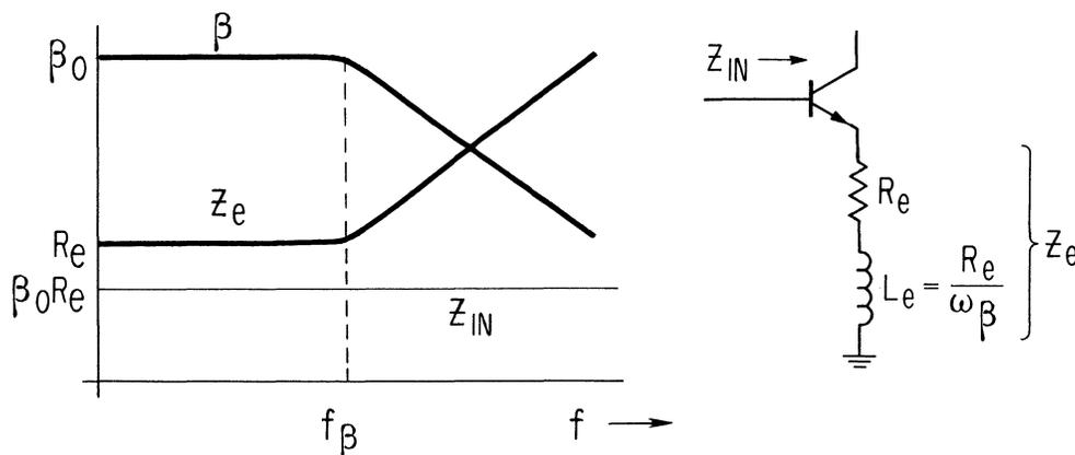
Fig. 3 Emitter Inductance,  $L_e$ , Can Compensate for Falling  $f_\beta$  as Frequency Increases
