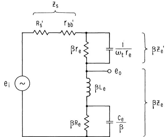
Fig. 6(b) Equivalent Circuit
