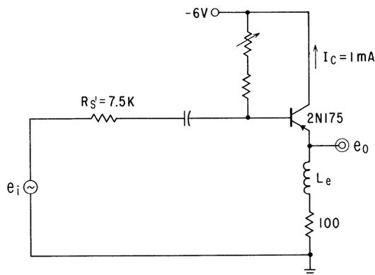
Fig. 4(a) A Circuit Demonstrating the Compensating Method
