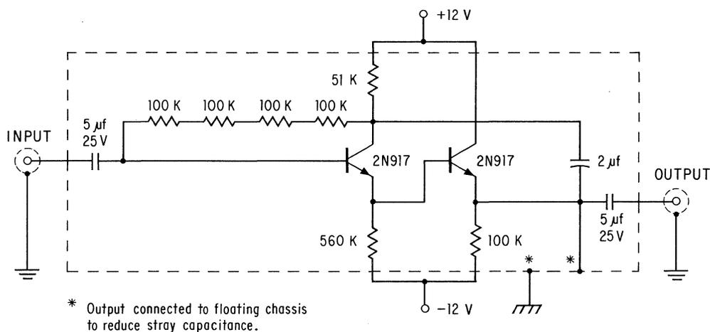
Fig. 5 Wideband High Input Impedance Amplifier.
