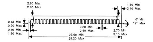
**NOTE:** Dimensions for the QFP package are in millimeters.
