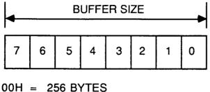
01H = 512 BYTES 03H = 1K BYTES 07H = 2K BYTES 0FH = 4K BYTES 1FH = 8K BYTES 3FH = 16K BYTES 7FH = 32K BYTES FFH = 64K BYTES
