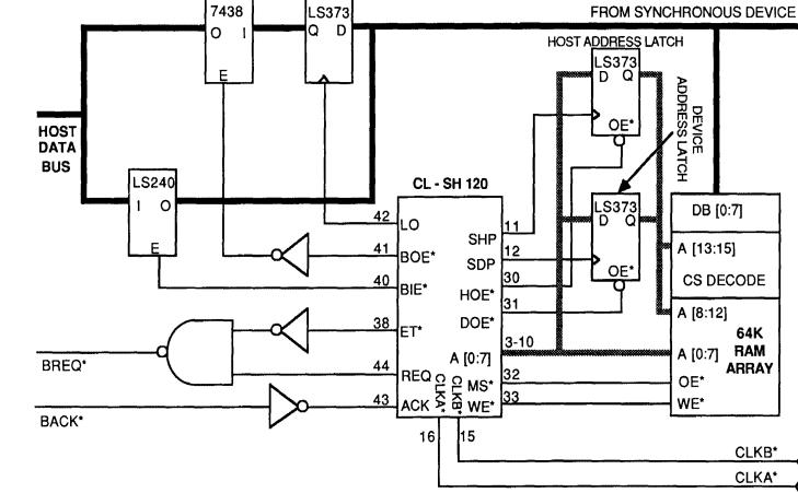
Figure 4.3 Maximum Addressing Mode (Not available in 40-pin P-DIP parts)
