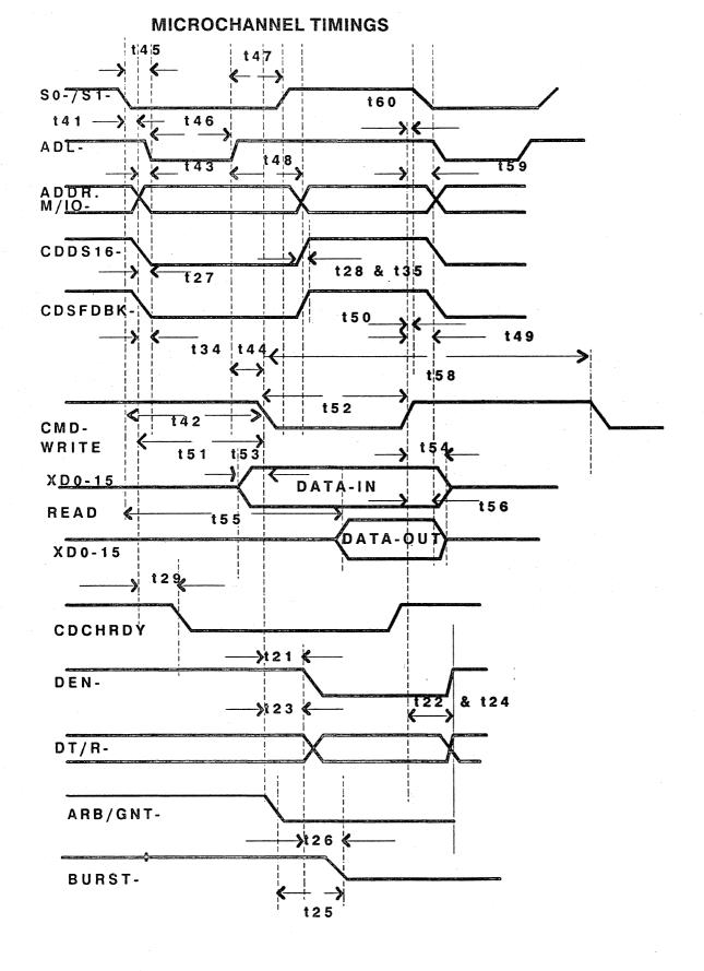
MICROCHANNEL TIMINGS: (ta=0 DEG C TO 70 DEG C VCC=5v +/-5%, CI=35pf for all outputs except microchannel interface pins, PREMPT-,BURST-,ARB00 thru ARB03 which are rated at 240pf max and CDCHRDY,CDSFDBK-,CDDS16- at 85pf)
