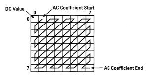
Figure 1-4 Zigzag Reordering of the 8x8 DCT Coefficients
