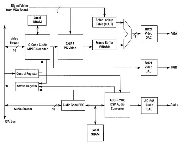
Figure 9-2 Block Diagram of CL450 Development Board
