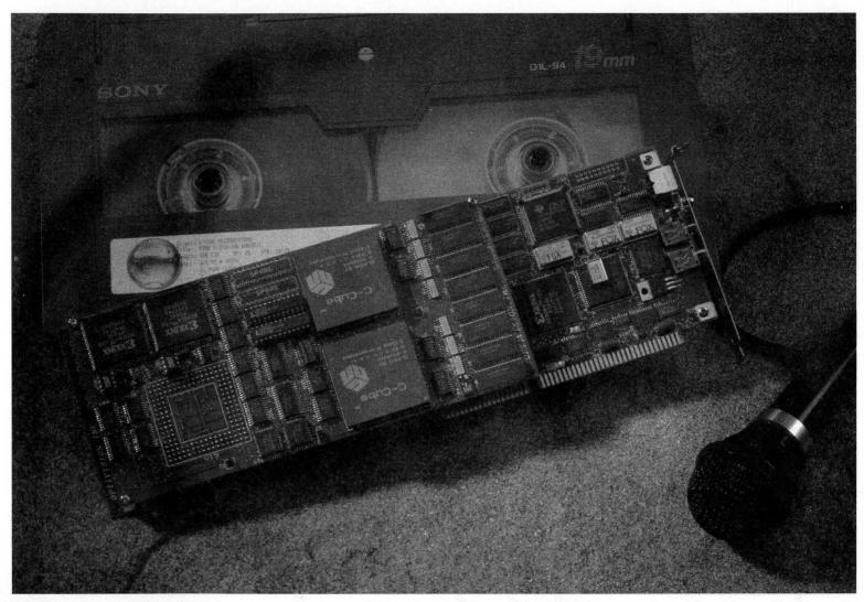
The CLM4500 uses two VideoRISC Processors to compress digital video into SIF-resolution MPEG bitstreams in real time. The product pictured above is the OPTIVideo™ board from OPTIVISION, Inc.
