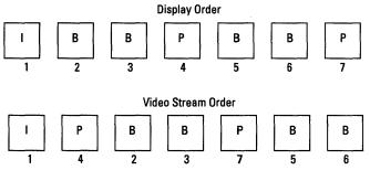
Figure 2-8 Video Stream versus Display Ordering
