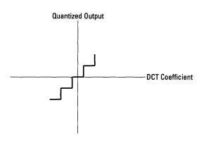
Figure 1-2 Quantizer Stepping (Uniform Quantization)
