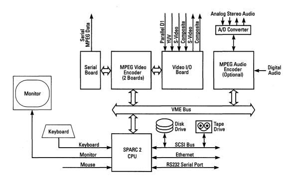
Figure 7-1 VideoRISC Encoder Development System Block Diagram
