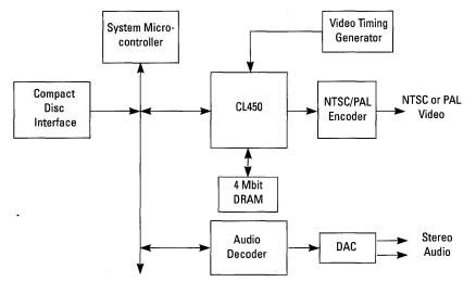
Figure 8-2 Typical CL450 System Application
