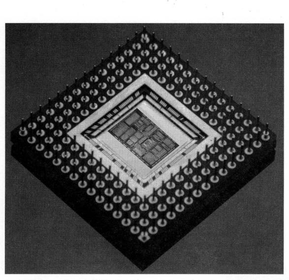
The CL560 is the successor to the CL550, which was the world's first JPEG processor when it was introduced in 1990. Both products are high-performance single-chip JPEG processors that encode and decode gray-scale and color images at video rates.
