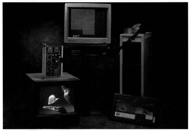
The MPEG Encoder Development Station uses the CLM4600 to encode video and audio sequences into MPEG 1 syntax in real time.
