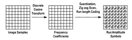
Figure 2-9 Transform Coding Operations
