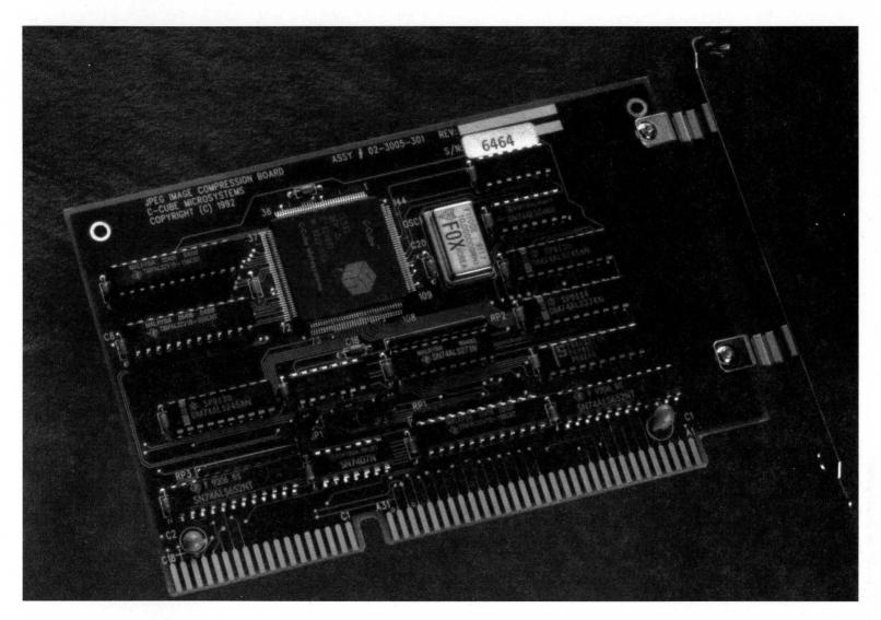
C-Cube's JPEG Still-Image Board is an ISA-bus card that compresses and decompresses graphic images using the CL550 JPEG Processor.
