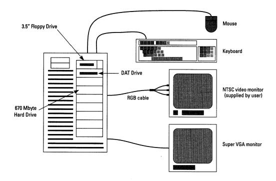
Figure 10-1 Video Lab Components
