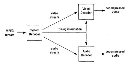
Figure 2-1 General MPEG Decoding System
