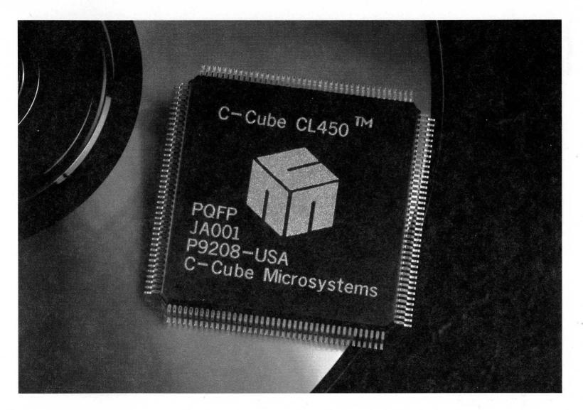
The CL450 MPEG Video Decoder provides full-motion video capability for cost-sensitive electronics products.
