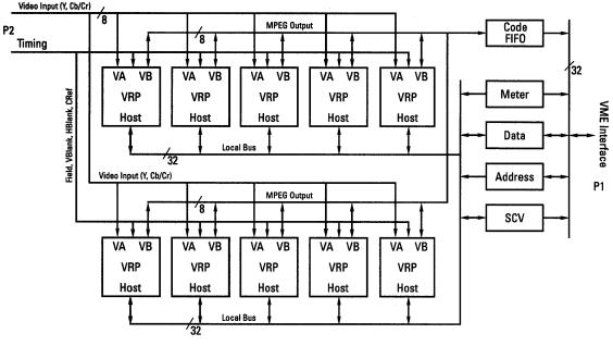
Figure 6-1 CLM460x-Based Video Encoding System
