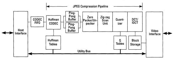
Figure 3-2 CL560 Block Diagram
