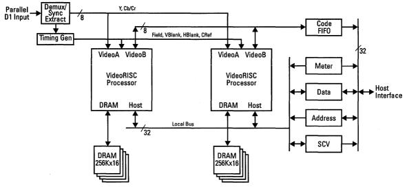
Figure 5-1 CLM4500-Based Video Encoding System
