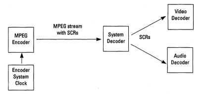
Figure 2-10 SCR Flow in MPEG System
