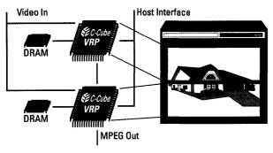
Figure 6-2 Scaled Image Processing
