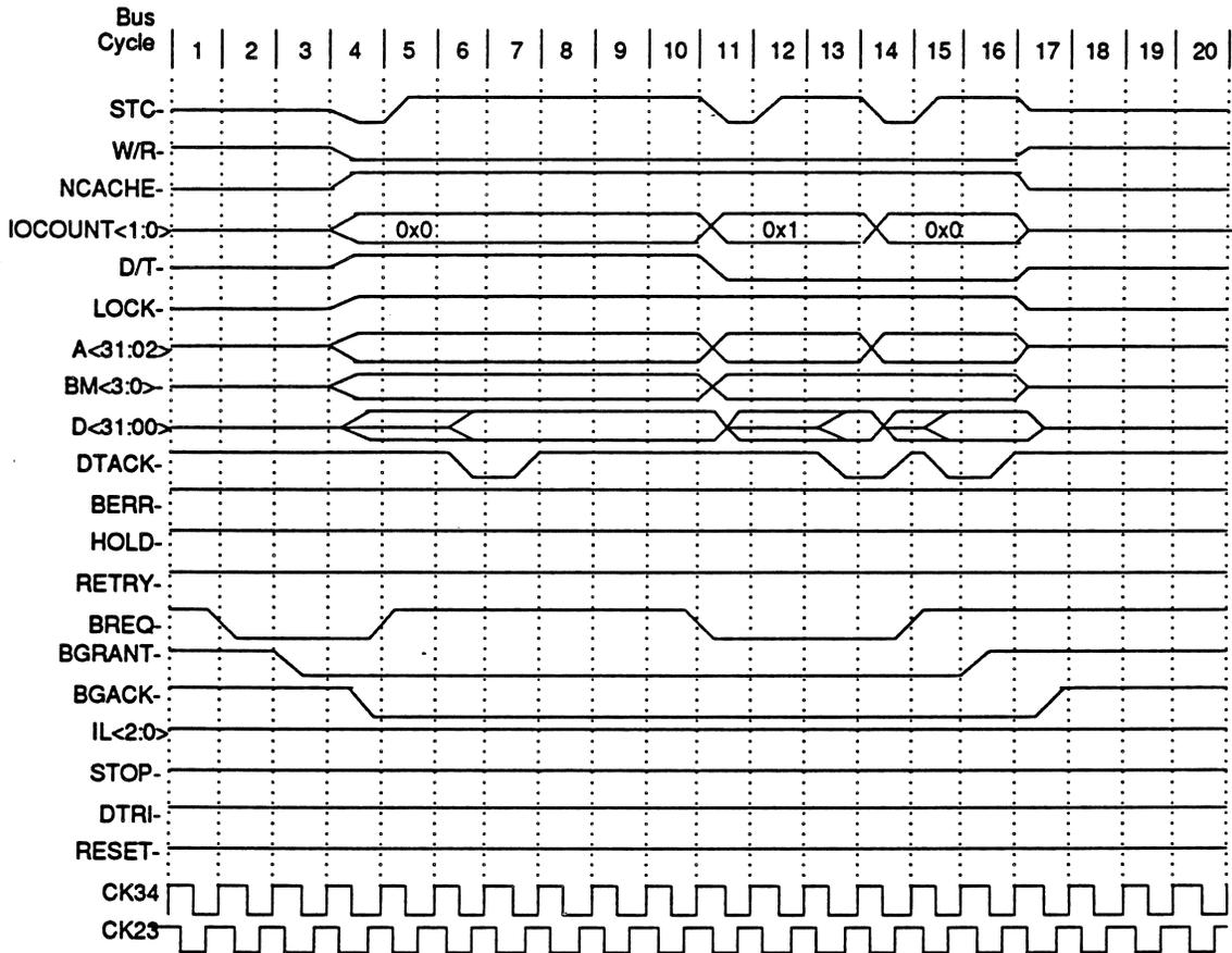
Figure 5-2. ATT2100 Read Bus Cycles with Bus Arbitration
