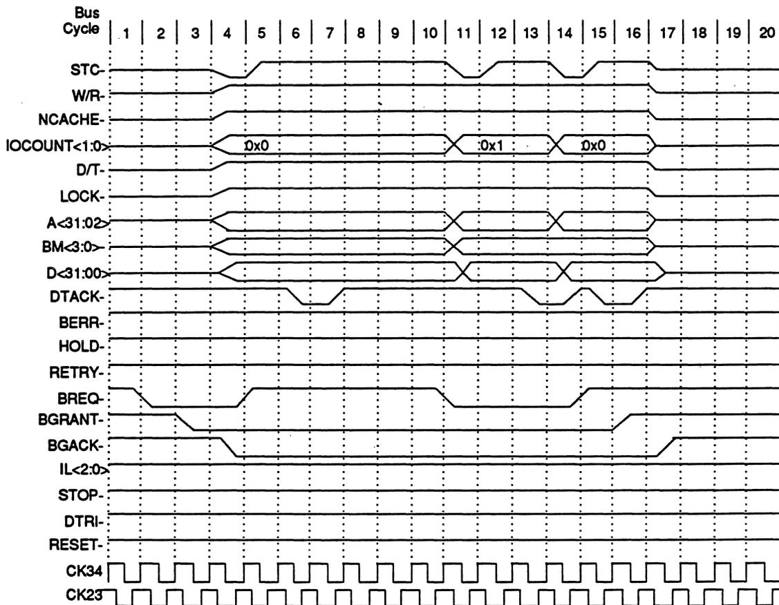
Figure 5-3. ATT2100 Write Bus Cycles with Bus Arbitration
