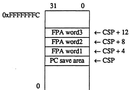
Figure 2-4. Floating-point Accumulator
