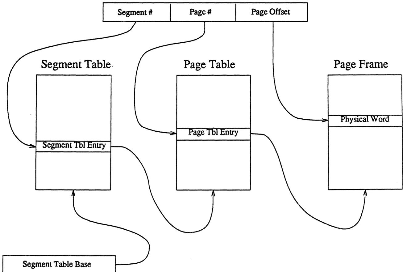
Figure 6-7. Paged Segment Address Mapping
