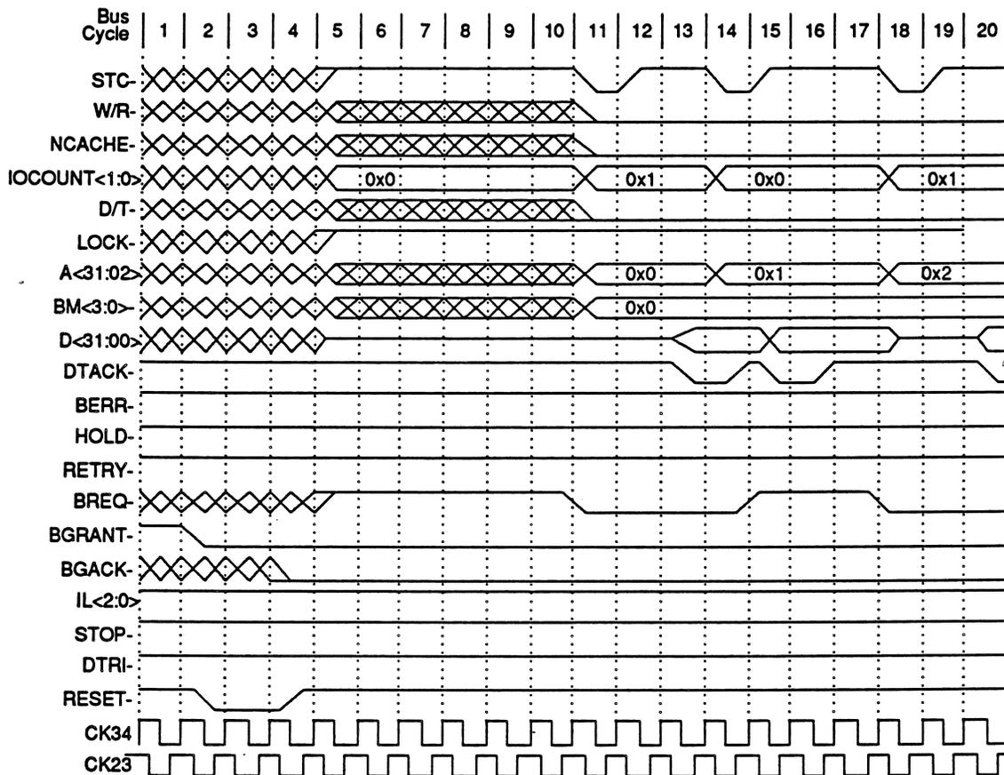
Figure 5-1. Reset with Bus Grant Asserted
