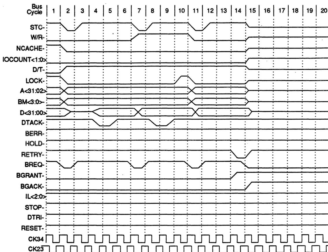
Figure 5-4. Interlocked Bus Transfer without and with Retry
