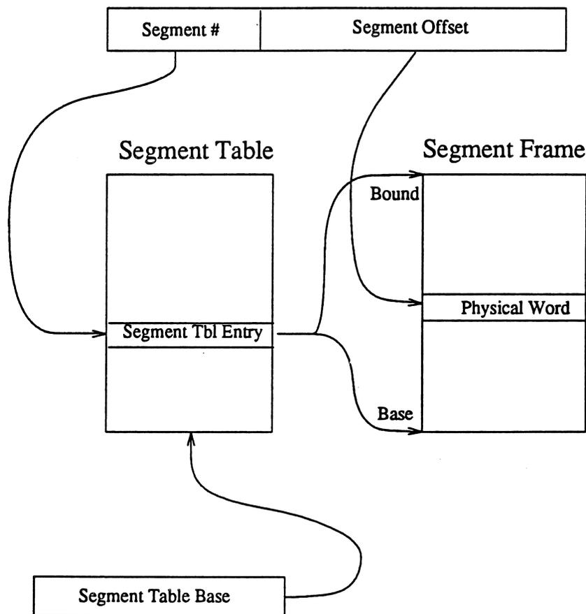
Figure 6-8. Non-paged Segment Address Mapping
