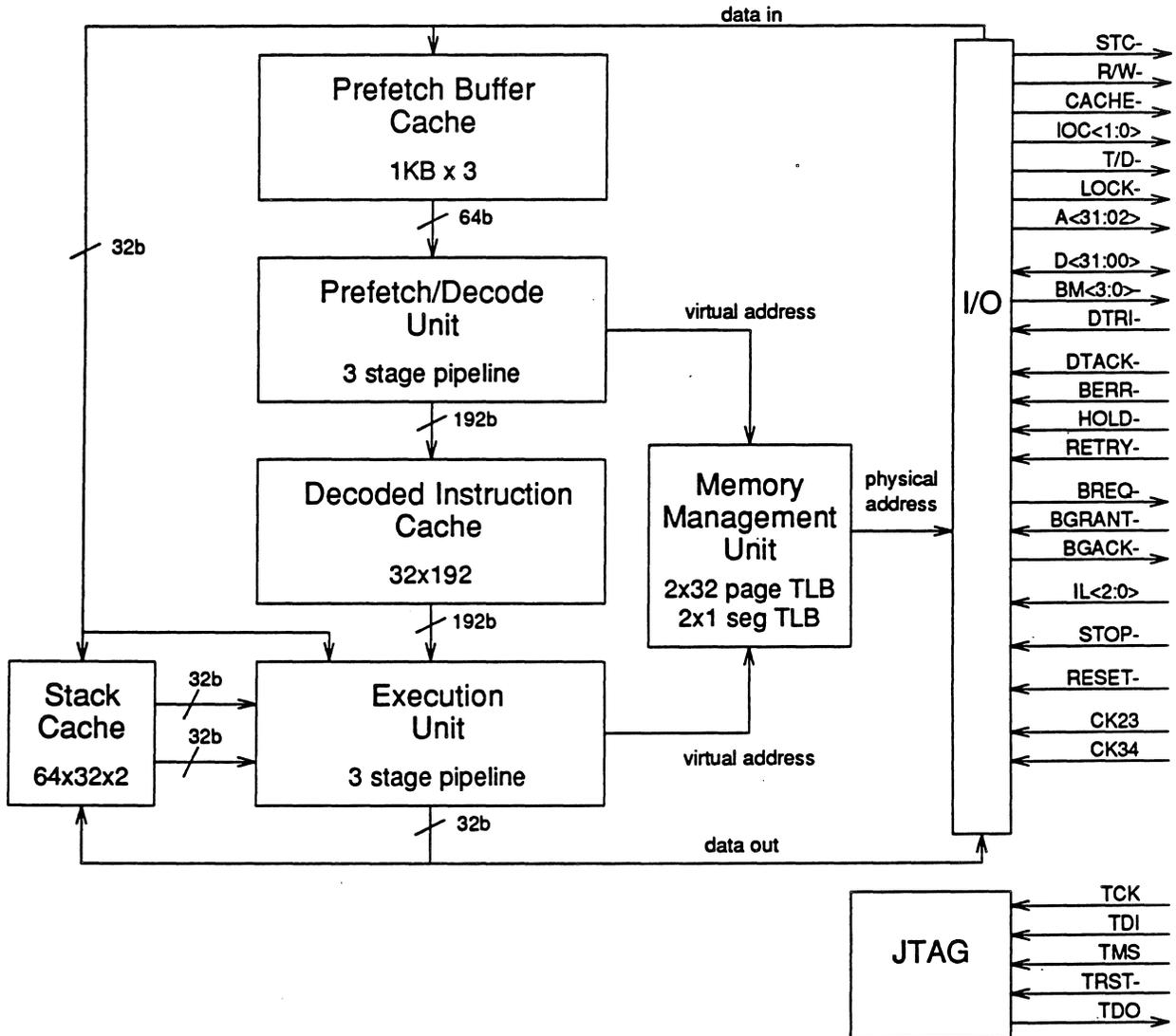
Figure 1-1. ATT2100 Functional Block Diagram
