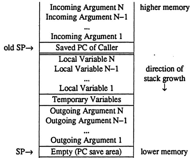
Figure 2-14. Typical Stack-frame
