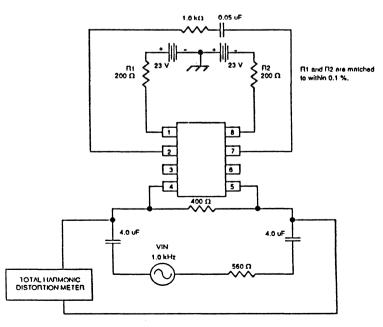
Figure 4. Distortion, Test Circuit
