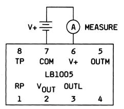
Figure 1. Test Circuit (Power Supply Current)
