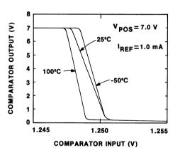
Figure 6. Typical Comparator DC Transfer Characteristics vs Temperature
