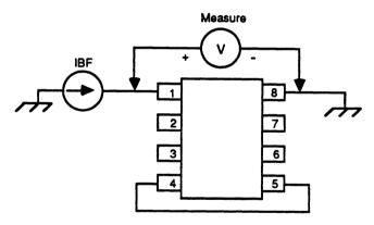
Figure 6. Battery Feed Total Voltage, Test Circuit
