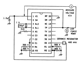
Figure 9. Voltage (TP-to-VS), Dial
