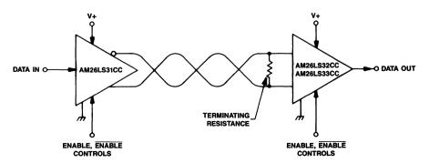
Figure 13. AM26LS32CC, AM26LS33CC Quad Line Receiver Application Diagram
