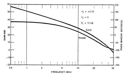
Figure 15. Open-Loop Gain and Phase vs. Frequency
