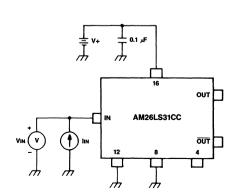
Figure 2. Input Clamp Voltage
