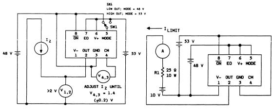
Figure 8. Output Current Threshold Test
