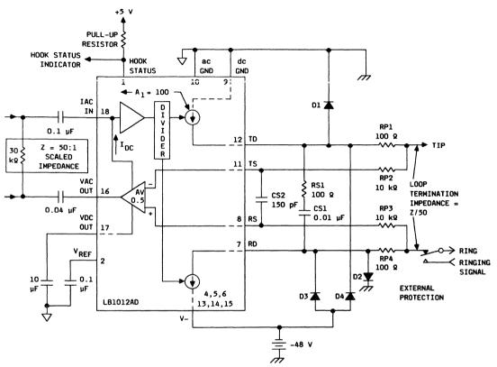
Figure 22. LB1012AD Battery Feed Application Diagram
