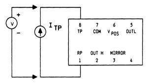
Figure 10. Clamp Voltage (ITP)
