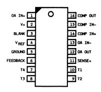
Figure 2. 16-Pin Plastic DIP
