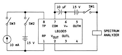
Figure 6. Test Circuit (Output Frequency and Modulation Rate)
