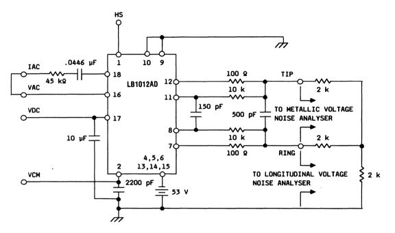
Figure 20(c). LB1012AD Noise Test Circuit
