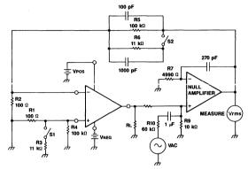
Figure 1. Open Loop Gain Test Circuit
