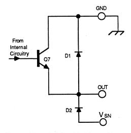
Figure 2. LS1098AAF Simplified Output Diagram
