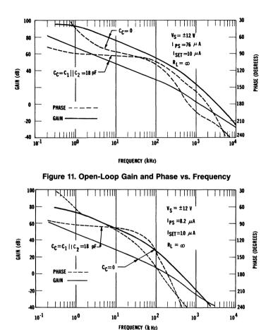
Figure 12. Open-Loop Gain and Phase vs. Frequency
