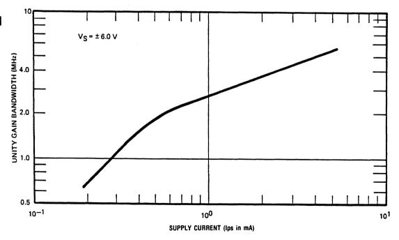
Figure 15. Supply Current/Unity Bandwidth Characteristic
