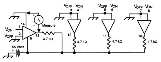
Figure 6. Output-On Voltage Test Circuit
