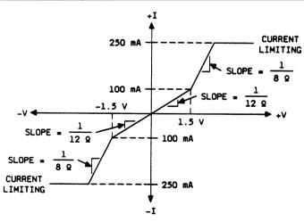
Figure 1. LH1061AB Typical ON Characteristics
