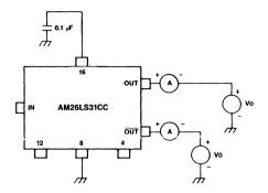
Figure 5. Output Current (Power OFF)
