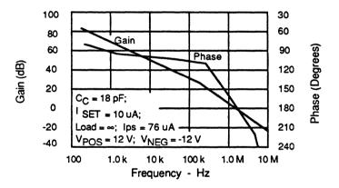
Figure 11. Open Loop Gain and Phase vs Frequency
