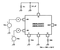
Figure 2. Differential Input Threshold Voltage
