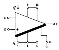
Figure 11. Low Current Output No Offset Null Internal Compensation
