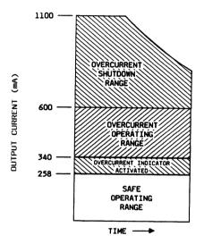
Figure 1 is an output diagram of a typical LB1019AB at room temperature as a function of load current.
