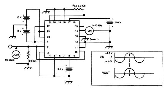
Figure 13. Crosstalk Test Circuit
