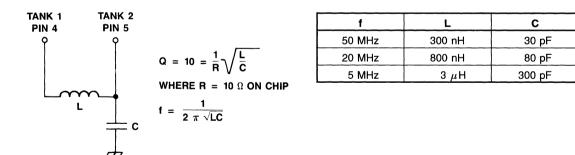
Figure 7. External Connections for Oscillation
