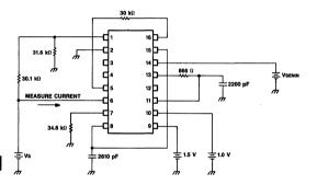
Figure 1. Power Supply Current Test Circuit
