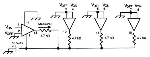
Figure 5. Fail-Safe Output Leakage Current Test Circuit
