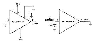
Figure 6. Logic Input Current, On
