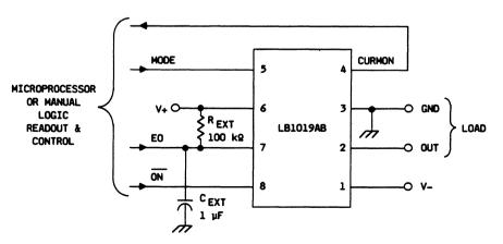
Figure 10. Typical Application Diagram for LB1019AB
