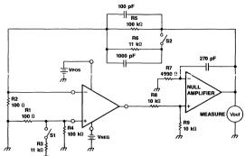
Figure 2. Input Offset Voltage (Vio), Input Bias Current (IB), and Input Offset Current (Io) Test Circuit
