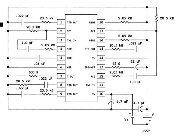
Figure 21. LB1021AD Test Circuit
