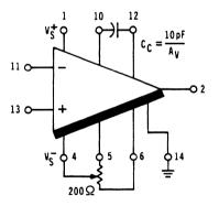
Figure 14. High Current Output Offset Null External Compensation
