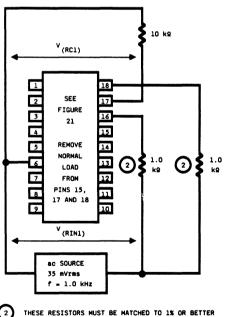
Figure 29. LB1021AD Test Circuit
