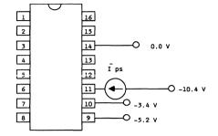
Figure 2. Power-Supply Current (+ Ips) Test Circuit
