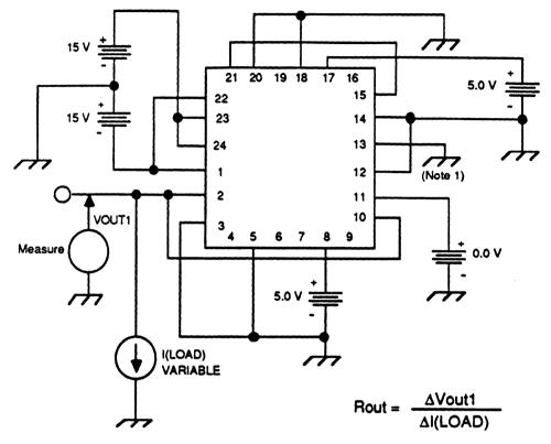
Figure 7. Output Resistance Test Circuit
