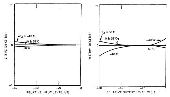
Figure 10. Temperature Stability of the Compressor
