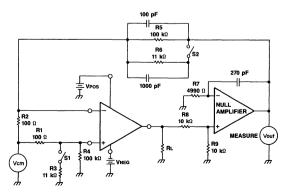
Figure 5. Common Mode Voltage Range and Common-Mode Rejection Ratio Test Circuit
