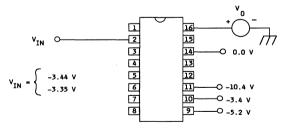
\*REPEAT FOR INPUTS/OUTPUTS 2-4, CONNECT A 0.1µfd CAPACITOR FROM EACH OF THE LEADS 1,3,6,8, AND 10 TO GROUND
