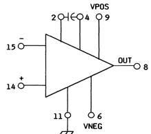
Figure 5. Internal Bias Setting External Feedback Compensation
