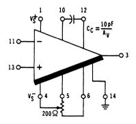
Figure 13. Low Current Output Offset Null External Compensation
