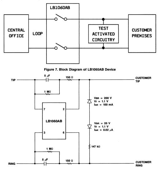
Figure 8. Typical Application Diagram for LB1060AB in Maintenance Termination Unit (MTU)
