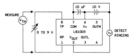
Figure 3. Test Circuit (Input Threshold Voltage)
