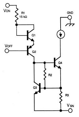
Figure 1. LS1098AAF Simplified Input Diagram
