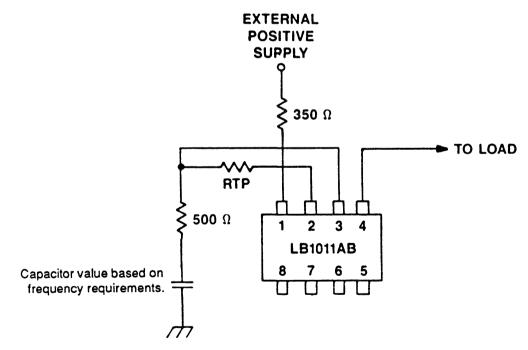
Figure 14. Battery Feed Application (Unbalanced Configuration)
