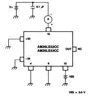
Figure 8. Power Supply Current
