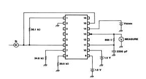
Figure 3. Sense Amplifier Output Voltage Test Circuit
