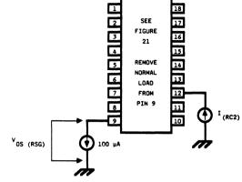
Figure 27. LB1021AD Test Circuit
