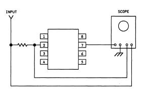
Figure 2. Hold Current and Breakover Voltage Tests
