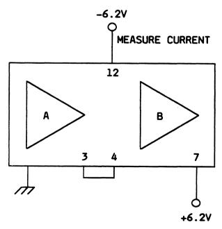
Figure 4. Test Circuit, Power-Supply Current
