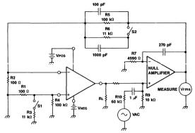
Figure 1. Open Loop Gain Test Circuit
