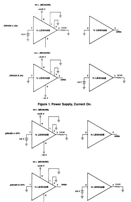
Figure 2. Power Supply, Current Off
