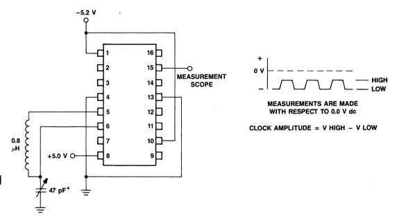
\* Capacitor should be adjusted so the resonant frequency of the tank circuit (including lead length, etc.) is nominally 20 MHz. Figure 3. Clock Level High and Low; Clock Amplitude
