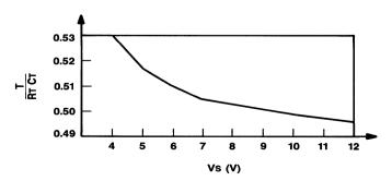
Figure 6. Ratio of Ramp Generator Period (T) to RT CT Time Constant vs. Supply Voltage
