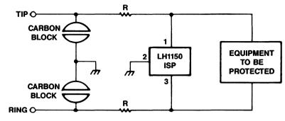
Figure 2. Application Diagram
