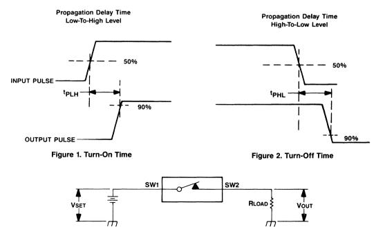
Figure 3. Test Method for Switching Time and Switch Offset Voltage
