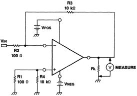
Figure 4. Output Voltage Swing Test Circuit
