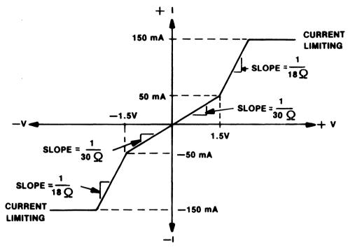
**Figure 1. Typical ON Characteristics**
