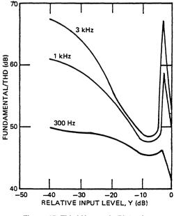
Figure 15. Third Harmonic Distortion of the Compressor
