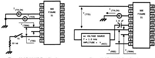
Figure 36. LB1021AD Test Circuit
