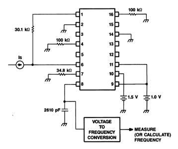
Figure 5. Ramp Generator Frequency Test Circuit
