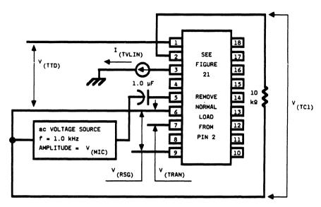
Figure 38. LB1021AD Test Circuit
