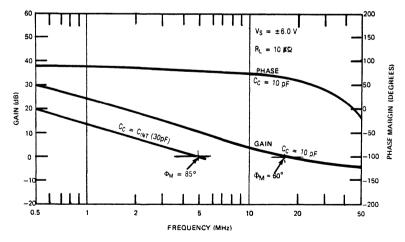
Figure 17. Open-Loop Gain and Phase vs. Frequency
