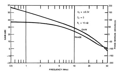
Figure 16. Open-Loop Gain and Phase vs. Frequency
