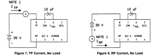
Note 1: Current is measured between 30 ms and 40 ms after ringing has been detected ("OUT H" sources current when ringing has been detected).
