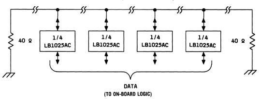
Figure 7. LB1025AC Quad Bus Transceiver Application Diagram
