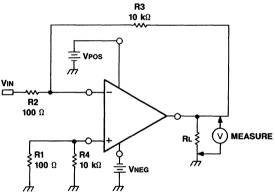
Figure 4. Output Voltage Swing Test Circuit
