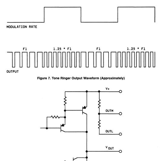
Figure 8. Simplified Tone Ringer Output Diagram
