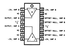
Power-supply connections are common for two amplifiers. If offset null is not desired for either amplifier, leads 10, 11, 13, and 14 must be connected to lead 12.
