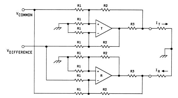
Figure 7 shows connections to achieve a transconductance configuration for telephone line drive applications.
