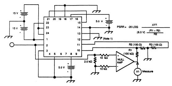
Figure 12. Power Supply Rejection Ratio Test Circuit
