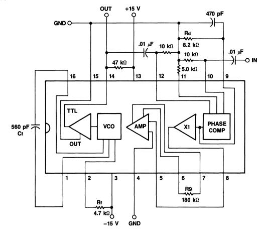
Figure 5. 200 kHz Synchronizer Application
