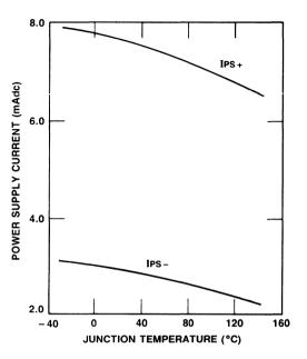
Figure 12. Typical Power Supply Current vs. Temperature
