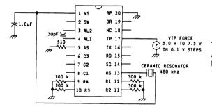
The voltage on TP is ramped until the signal on either AL1 or AL2 (with respect to RP) exceeds 1.0 volts. Ring Detect is defined as the condition where voltage exceeds 1.0 volts on AL1 or AL2.
