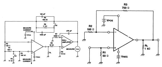
Figure 7. Power Supply Quiescent Current Test Circuit
