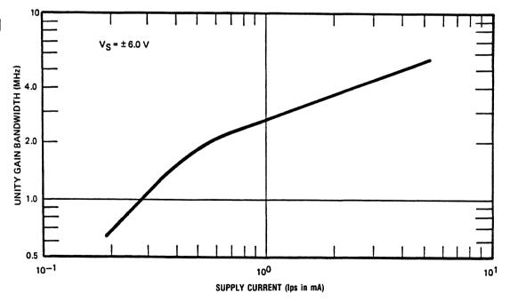
Figure 14. Supply Current/Unity Bandwidth Characteristic
