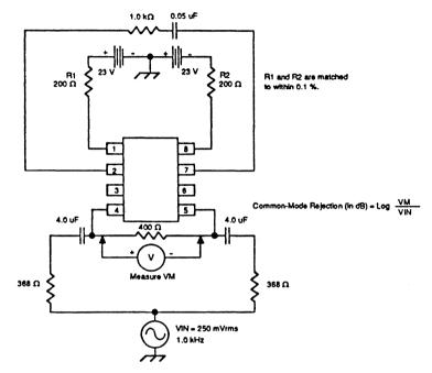
Figure 3. Common-Mode Rejection, Test Circuit
