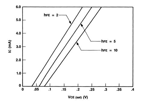
Current vs. Saturation Voltage (PNP)
