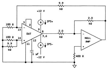
Figure 8. Power-Supply Current Test Circuit
