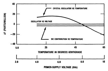
Figure 6. Frequency Deviation from Nominal 512 kHz
