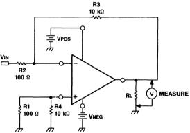
Figure 4. Output Voltage Swing Test Circuit
