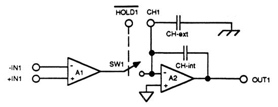
Figure 14. Simplified Functional Operation
