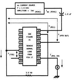
Figure 31. LB1021AD Test Circuit
