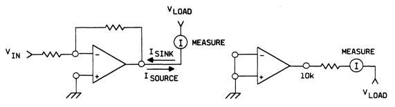
Figure 3. Test Circuit, Output Current
