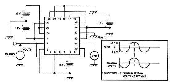
Figure 5. Full-Power Bandwidth Test Circuit
