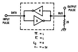
Figure 1. Driver Test Circuit
