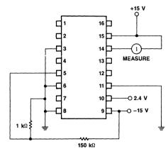
Figure 4. Logic Supply Current (I14)
