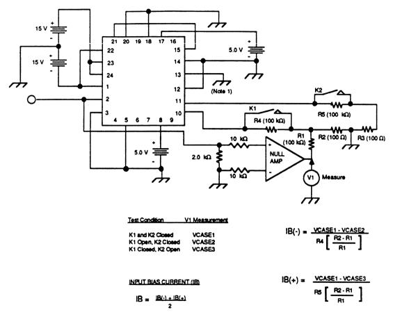
Figure 9. Input Bias Current Test Circuit
