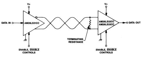
Figure 14. AM26LS31CC Quad Line Driver Application Diagram
