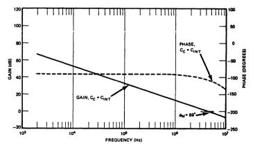
Figure 10. Gain and Phase vs. Frequency
