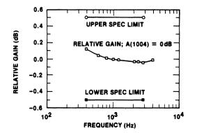
Figure 18(a). LB1012AA/AD Typical Gain vs Frequency Response
