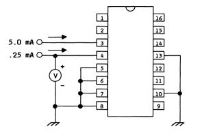
Figure 4. Saturation Voltage (VBE) Test Circuit
