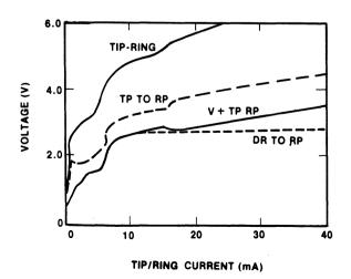
Figure 2. Typical V-I Characteristics (Speech Mode)
