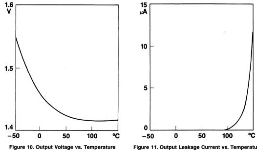
Figure 11. Output Leakage Current vs. Temperature
