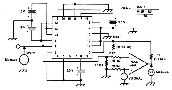
Figure 3. Open Loop Gain Test Circuit
