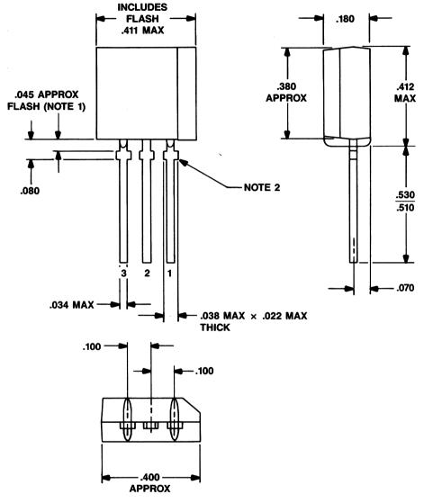
Note 1. Flash permissable in this area along with lead length not to exceed the .038" max. wide X .022" max thickness of the leads. Note 2. Burrs in trim are not to exceed overall lead thickness of .023".
