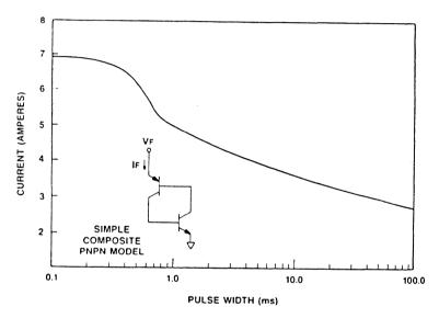
Figure 11. Maximum Applied Forward Surge Limits (PNPN Composite Device)
