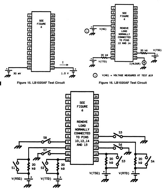
Figure 17. LB1020AF Test Circuit
