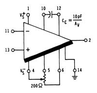
Figure 13. High Current Output Offset Null External Compensation
