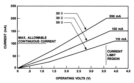
Figure 3. Output I/V Characteristics for Various Ron @ 25°C
