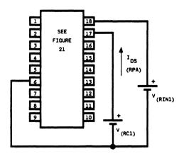
Figure 25. LB1021AD Test Circuit
