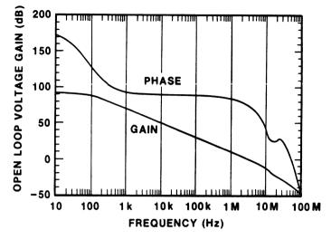
Figure 5. LB1108AD Open-Loop Frequency and Phase Response
