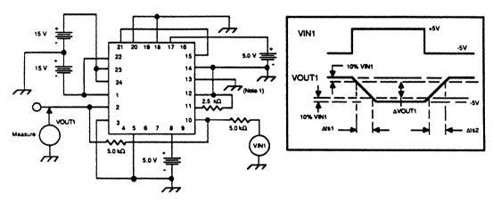
Figure 6. Slew Rate Test Circuit
