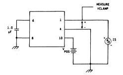
Figure 7. Clamp Voltage
