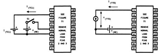
Figure 34. LB1021AD Test Circuit
