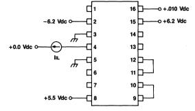
Figure 4. Logic Supply Current (IPSL)
