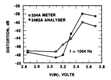
Figure 21(a). Typical Distortion vs Input Characteristics
