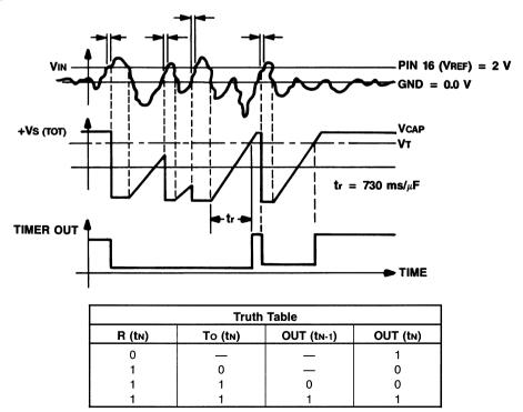
Figure 8. Timing Diagram and Truth Table
