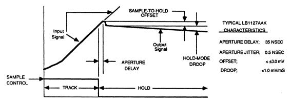
Figure 15. Several Sample-Hold Characteristics
