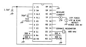
ITP (for this test) is defined as the current in Pin 17 just prior to Ring Detect. Lower the voltage applied to pin 17 to a value which is 250 mV less than the TP Ring Detect voltage value (which was measured in Figure 4).
