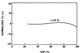
Figure 13. Temperature vs. Input Offset Voltage (Normalized) at Various Supply Voltages
