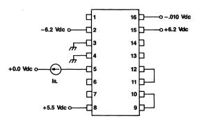
Figure 6. Input Forward Current, V(4) = 0
