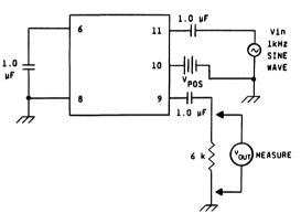
Figure 2. Expander, Input Gain Ratio
