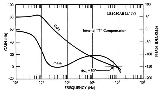
Figure 10. Typical Gain and Phase vs. Frequency
