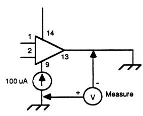
Figure 10. Forward Voltage, Output Diode D2 Test Circuit
