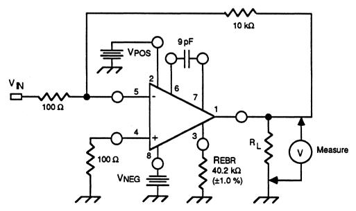
Figure 4. Output Voltage Swing Test Circuit
