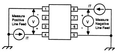
Figure 7. Line/Supply Voltage, Test Circuit
