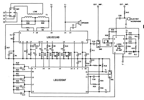
Figure 42. Typical Speakerphone Line-Coupled Application
