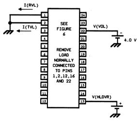
Figure 13. LB1020AF Test Circuit
