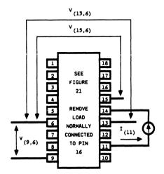
Figure 22. LB1021AD Test Circuit
