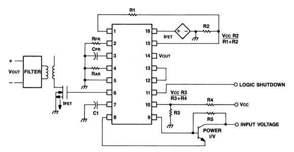
Figure 8. LB1132AC Switched-Mode PWM Application Diagram
