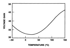
Figure 18. Typical Voltage Gain vs. Temperature
