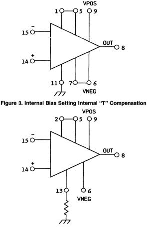
Figure 4. External Bias Setting Internal Feedback Compensation
