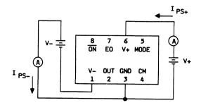
Figure 3. Power-Supply Current
