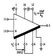
Figure 12. Low Current Output Offset Null External Compensation
