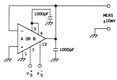
Figure 6. Test Circuit, Open Loop Voltage Gain Test Circuit
