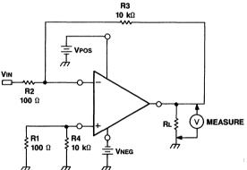
Figure 4. Output Voltage Swing Test Circuit
