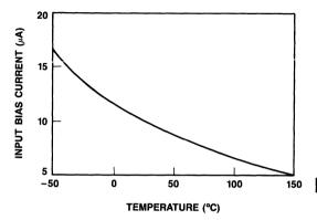
Figure 12. Typical Input Bias Current vs. Temperature
