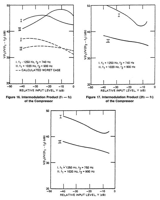
Figure 18. Intermodulation Product (2f1 — f2) of the Compressor
