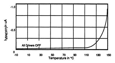
Figure 14. Typical Supply Current (IVSN(OFF)) vs Temperature
