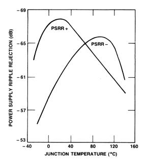
Figure 11. Typical Power Supply Ripple Rejection vs. Temperature
