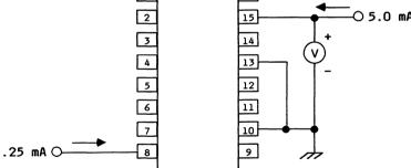
Figure 3. Saturation Voltage (VCE) Test Circuit
