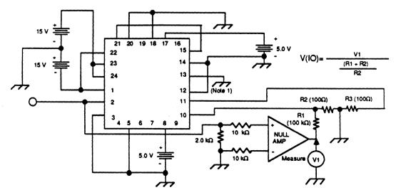
Figure 8. Input Offset Voltage Test Circuit
