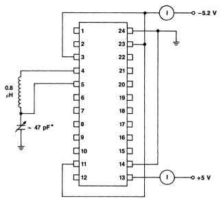
\* Capacitor should be adjusted so the resonant frequency of the tank circuit (including lead length, etc.) is nominally 20 MHz.
