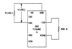
Figure 13. Test Circuit
