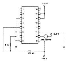
Figure 5. Strobe Leakage Current (I10)
