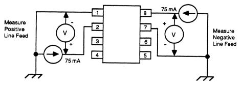
Figure 9. Supply/Cross Coupling Voltage, Test Circuit
