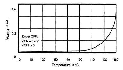
Figure 17. Typical Driver Von Input Current ( $I_{VON(L)}$ ) vs Temperature
