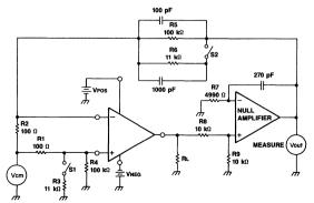
Figure 5. Common Mode Voltage Range and Common-Mode Rejection Ratio Test Circuit
