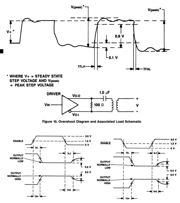
Figure 11. ENABLE and Output Waveforms
