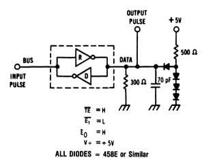
Figure 3. Receiver Test Circuit
