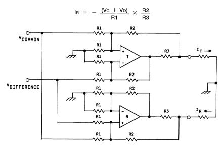
Figure 6. Simplified Line Feed Operation (Power-Supply Connections Not Shown)
