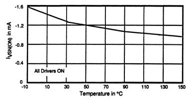
Figure 13. Typical Supply Current (Ivsn(on)) vs Temperature
