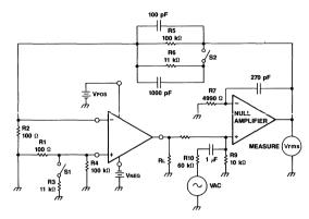
Figure 1. Open Loop Gain Test Circuit
