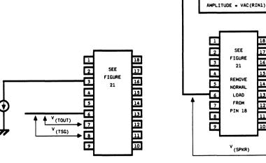
Figure 32. LB1021AD Test Circuit
