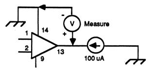
Figure 9. Forward Voltage, Output Diode D1 Test Circuit
