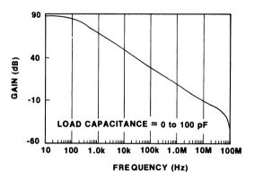
Figure 5. Op-Amp Open-Loop Gain
