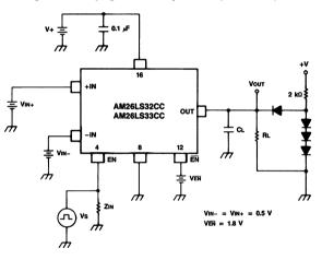
Figure 10. Propagation Delay Times (tplz, tprz, tpzl, tpzh)
