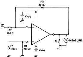
Figure 4. Output Voltage Swing Test Circuit
