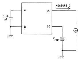
Figure 3. Microphone Bias Current
