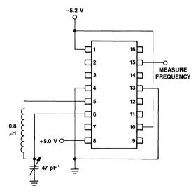
\* Capacitor should be adjusted so the resonant frequency of the tank circuit (including lead length, etc.) is nominally 20 MHz.
