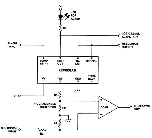
Figure 13. Regulation Control General Application Diagram
