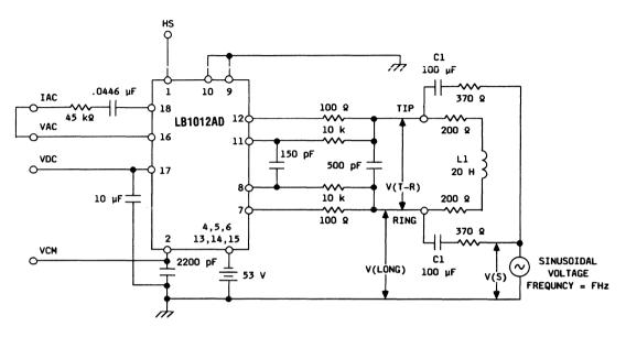
Figure 19(b). Longitudinal Balance Test Circuit
