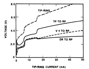
Figure 1. Typical V-I Characteristics (Dial Mode)
