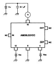
Figure 3. Power Supply Current, No Load & Disabled (Ven  $\leq$  0.8 V)
