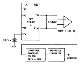
Figure 15. Test Circuit
