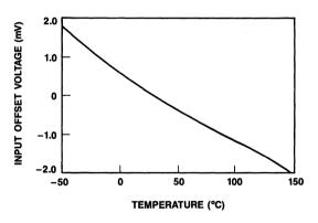
Figure 17. Typical Darlington Input Offset Voltage vs. Temperature
