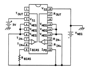
Figure 6. LB1108AD Op-Amp (Ground Return Connections)
