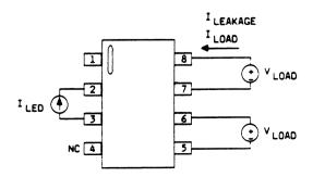
Figure 3. Test Circuit for Leakage and Limit Current
