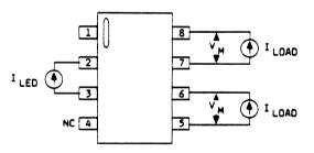
Figure 2. Test Circuit for Ron, ON Voltage and Breakdown Voltage
