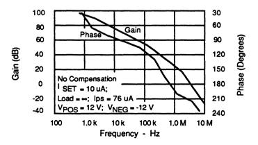
Figure 12. Open Loop Gain and Phase vs Frequency
