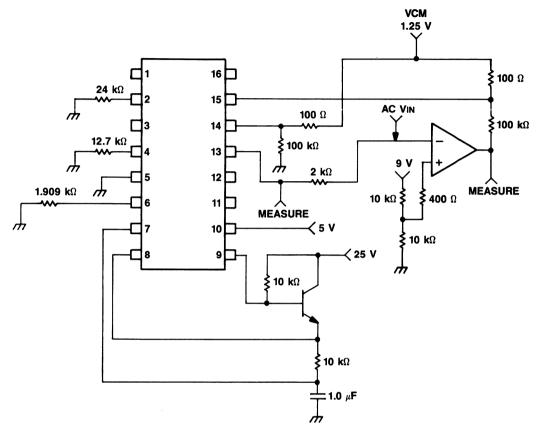
Figure 6. Open Loop Voltage Gain @ 10 kHz
