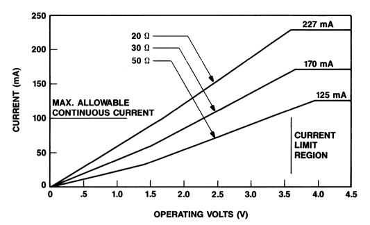
Figure 4. Output I/V Characteristics for Various Ron @ 0°C
