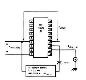
Figure 30. LB1021AD Test Circuit
