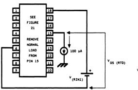
Figure 26. LB1021AD Test Circuit
