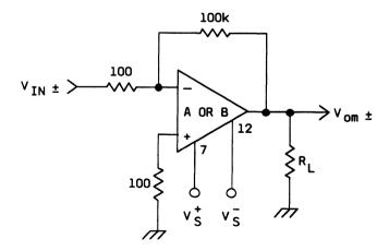
Figure 2. Test Circuit, Output Voltage Swing
