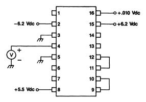
Figure 5. Input Forward Current, V(s) = 0
