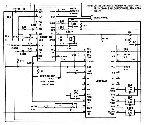
Figure 41. Typical Speakerphone Basic Application
