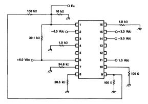
Figure 4. Input Offset Voltage Test Circuit
