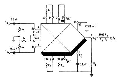
Figure 4. Internal Reference with Internal Resistor
