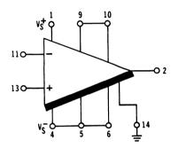
Figure 11. High Current Output No Offset Null Internal Compensation
