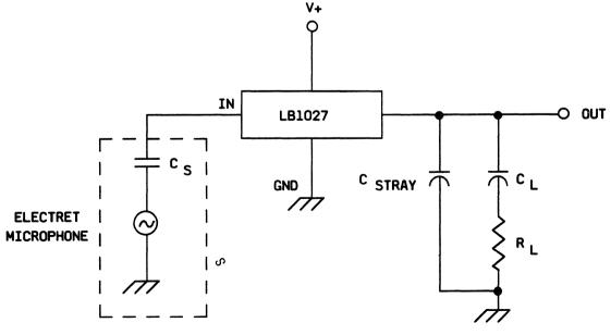
Figure 1. LB1027 Electret Preamplifier Application Diagram
