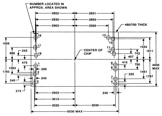
Note: Bonding pad numbers are for reference only. Bonding pads are 240 microns square, except where dimensioned otherwise.
