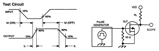
Figure 1. Switching Waveforms and Simplified Test Circuit
