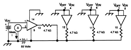
Figure 8. VOFF Input Current Test Circuit
