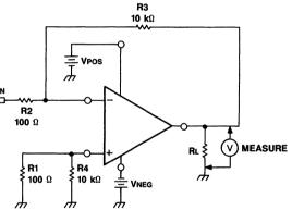
Figure 4. Output Voltage Swing Test Circuit
