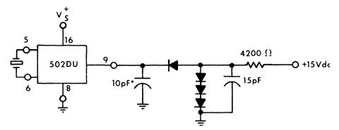
\*Includes probe, trigger circuit, and fixture capacitance. All diodes shall be 458E or equivalent.
