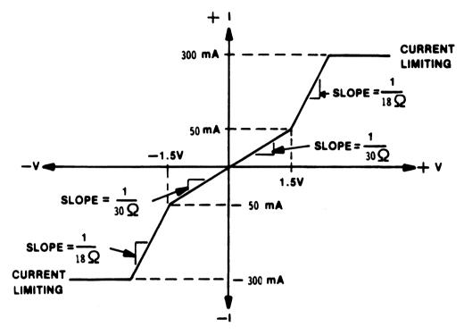
**Figure 1. Typical ON Characteristics**
