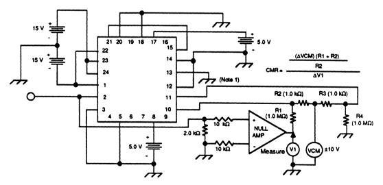
Figure 4. Common Mode Rejection Test Circuit
