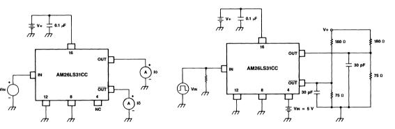
Figure 6. Output Current (Short Circuit)
