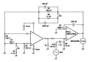
Figure 1. Open Loop Gain Test Circuit
