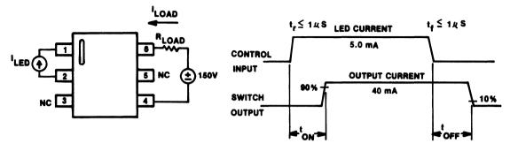
Figure 2. ton/toFF Test Circuit and Waveform
