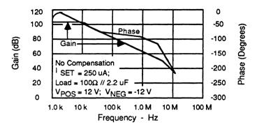
Figure 10. Open Loop Gain and Phase vs Frequency
