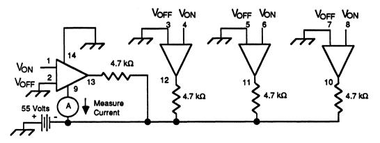
Figure 3. Supply Current Test Circuit
