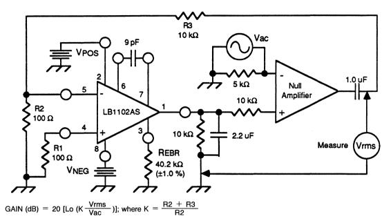
Figure 3. Open Loop Voltage Gain Test Circuit
