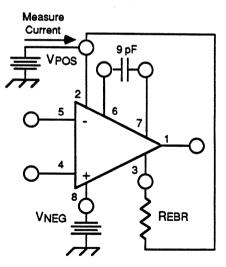
Figure 2. Power Supply Leakage Current
