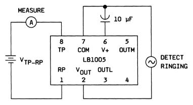
Figure 2. Test Circuit (TP and RP Currents, No Load)
