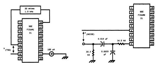
Figure 39. LB1021AD Test Circuit
