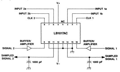
Figure 20. LB1017AC High-Speed Dual Analog Switch Sampling Application
