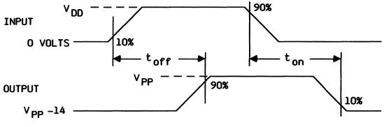
Figure 1. Switching Waveforms
