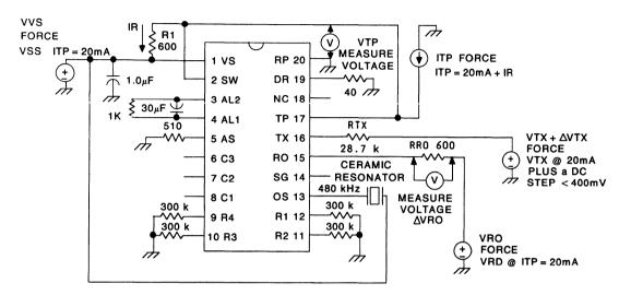
DETERMINE THE VALUE OF IR AND RECORD VRO VOLTAGE: Force 20 mA into RP (Pin 17) with TX (Pin 16) open and R1 disconnected. Measure VVS voltage (Pin 1), VTP voltage (Pin 17) and VRO voltage (Figure 18). Then, IR (mA) = [(VTP - VSS)/600] times 1000.
