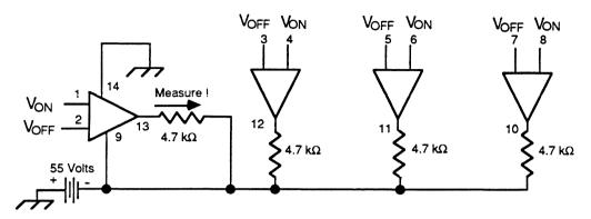
Figure 4. Fail-Safe Output Leakage Current Test Circuit
