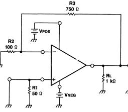
Figure 7. Power Supply Quiescent Current Test Circuit
