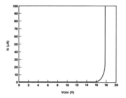
Current vs. Breakdown Voltage (PNP 1X)
