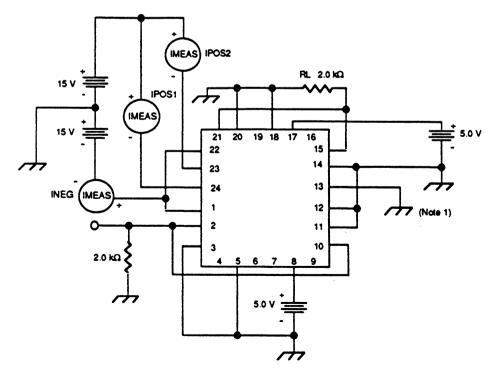
Figure 11. Power Supply Current Test Circuit
