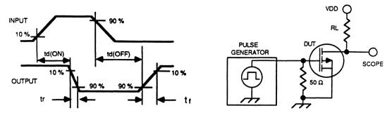
Figure 1. Switching Waveforms and Simplified Test Circuit
