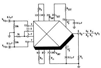
Figure 6. Internal Reference with External Resistor to the Positive Power-Supply
