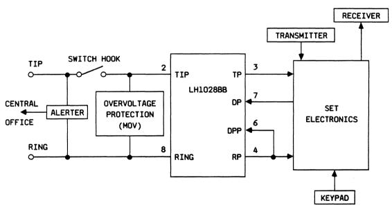
Figure 7. Typical Telephone Set Configuration
