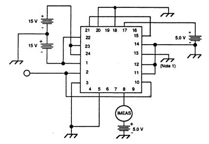
Figure 10. Logic Input Current Test Circuit
