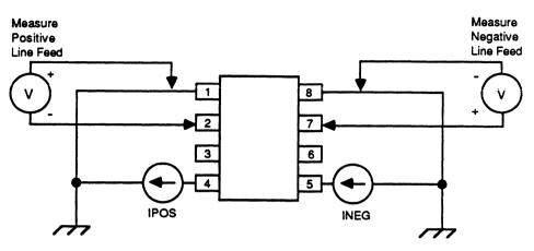
Figure 5. Base-to-Emitter Voltage, Test Circuit
