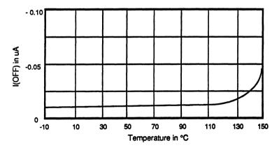
Figure 20. Typical Driver Output-Off Current (I(OFF)) vs Temperature
