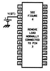
Figure 12. LB1020AF Test Circuit
