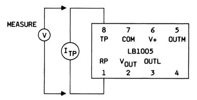
Figure 5. Test Circuit (Clamp Voltage)
