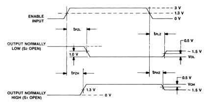
Notes: S1 and S2 of Load Circuit are Closed Except as Noted Above, and V ENABLE = 1.8 V Pulse Generator: Rate  $\leq$  1.0 MHz, Z0 = 50  $\Omega$ , tr  $\leq$  15 ns, tf  $\leq$  6 ns
