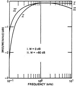
Figure 13. Frequency Response of the Expandor
