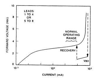
Figure 12. Typical Voltage vs Current (PNPN Composite Device)
