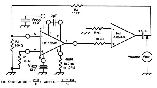
Figure 6. Input Offset Voltage
