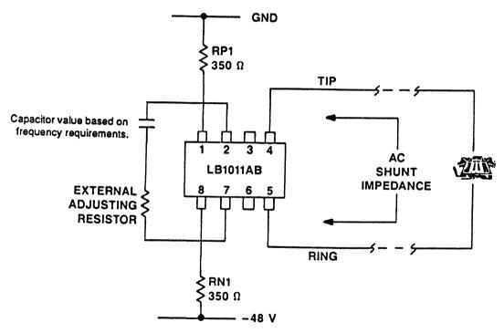
Figure 13. Battery Feed Application (Balanced Configuration)
