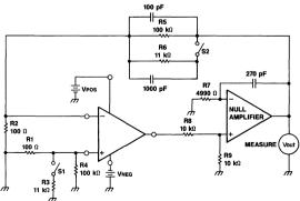
Figure 6. Power Supply Rejection Ratio Test Circuit
