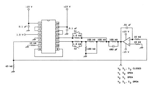
Figure 1. Input Offset Voltage (Vio), Input Bias Current (IIB), and Input Offset Current (IIO) Test Circuit
