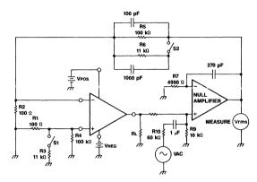
Figure 1. Open Loop Gain Test Circuit
