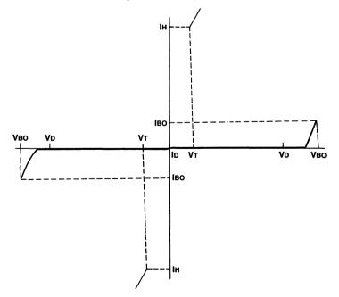
Figure 1. Typical Electrical Characteristics
