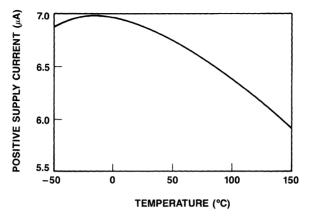
Figure 8. Typical Positive Supply Current vs. Temperature
