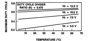
Figure 8. Maximum Duty Cycle as a Function of Temperature for Various Supply Voltages
