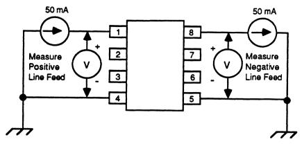
Figure 1. DC Voltage Drop, Test Circuit
