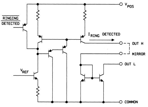
Figure 12. Simplified Output Diagram
