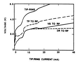
Figure 2. Typical V-1 Characteristics (Speech Mode)
