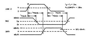
Figure 6. TE to Driver and Receiver Timing Waveform
