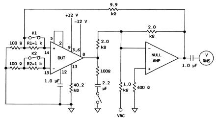
Figure 7. Input Offset Voltage (VIO), Input Bias Current (IIB), Input Offset Current (IIO) and Power-Supply Rejection Ratio (PSRR) Test Circuit
