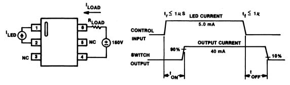
Figure 6. ton/toFF Test Circuit and Waveform
