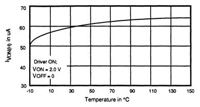
Figure 16. Typical Driver Von Input Current (I<sub>VON(H)</sub>) vs Temperature
