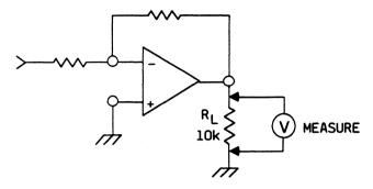
Figure 1. Test Circuit, Output Voltage Swing
