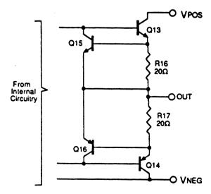
Figure 1. Sample-And-Hold Op-Amp Outputs (Simplified)
