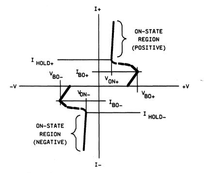
Figure 1. Symbology for Test Characteristics (Not to Scale)
