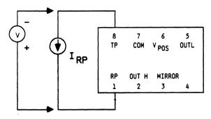
Figure 11. Clamp Voltage (IRP)
