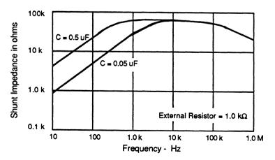
Figure 10. Typical Shunt Impedance vs Frequency
