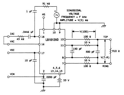
Figure 18(b). Frequency Response Test Circuit
