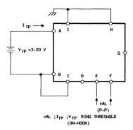
Figure 7. ON Hook dc Test Circuit
