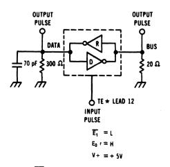
Figure 5. TE to Driver and Receiver Test Circuit
