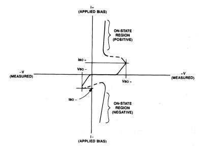
Figure 1. Symbology For Test Characteristics
