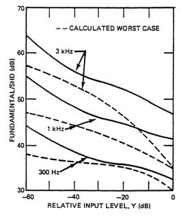
Figure 14. Second Harmonic Distortion of the Compressor
