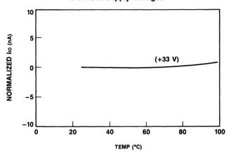
Figure 14. Temperature vs. Input Offset Current (Normalized) at Various Supply Voltages
