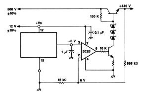
Figure 11. High-Voltage Application Using the LB1081CC 6 V Reference
