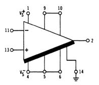
Figure 12. High Current Output No Offset Null Internal Compensation
