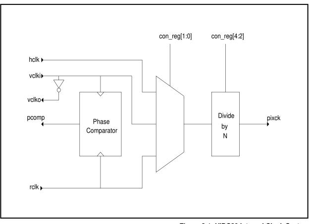
Figure 2-1: VIDC20 Internal Clock System
