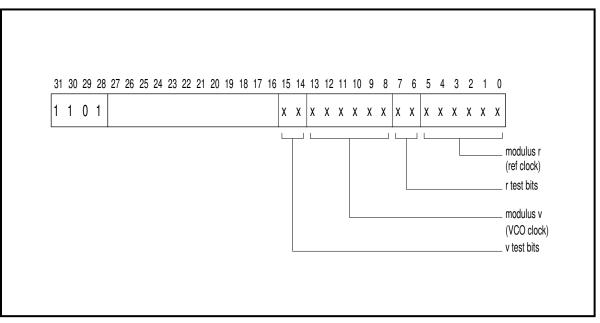
Figure 3-3: Frequency Synthesizer Register
