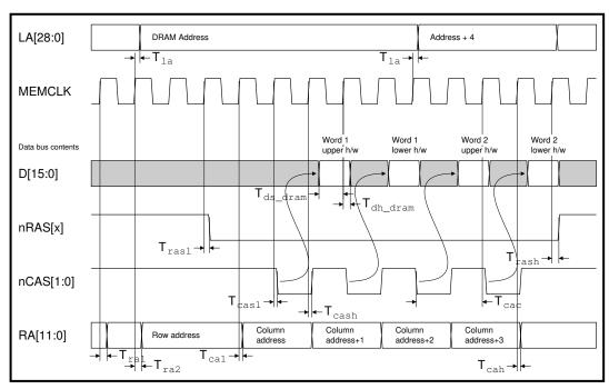
Figure 17-12: EDO DRAM read timing (16-bit mode)
