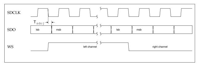
Figure 15-2: Serial sound output — Japanese format
