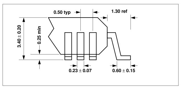
Figure 23-2: Side view of ARM7500FE chip
