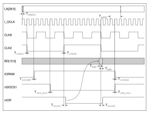
Figure 18-4: 'Sync' 8MHz I/O read cycle timing
