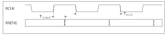
Figure 14-2: Timing relationship between ECLK and ED in LCD grayscale mode
