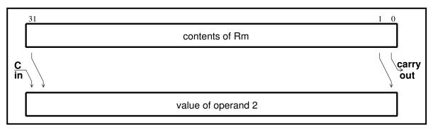
Figure 5-10: Rotate right extended
