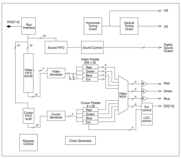
Figure 11-1: Video and sound macrocell block diagram
