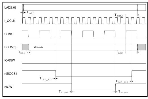
Figure 18-5: 'Fast' 8MHz Simple I/O write cycle timing
