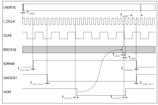
Figure 18-3: 'Slow' 8MHz Simple I/O read cycle timing
