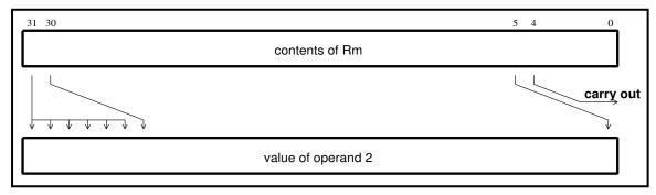
Figure 5-8: Arithmetic shift right
