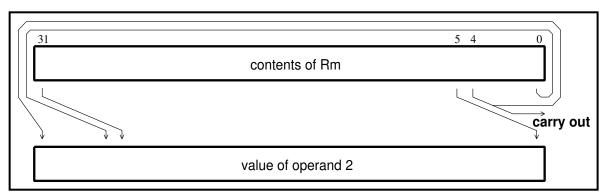
Figure 5-9: Rotate right
