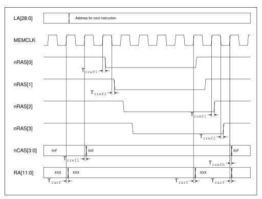
Figure 17-14: Refresh cycle timing
