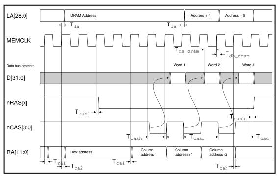
Figure 17-8: EDO DRAM read timing (32-bit mode)
