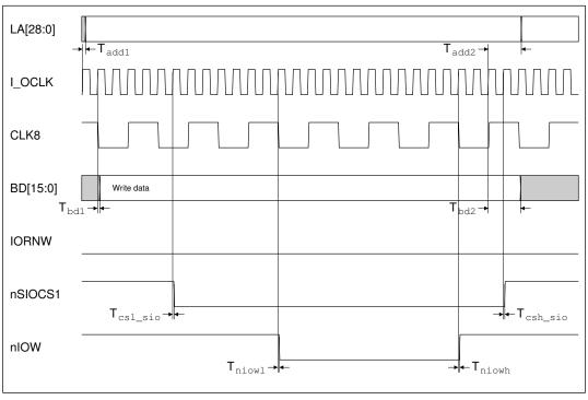
Figure 18-7: 'Slow' 8MHz Simple I/O write cycle timing
