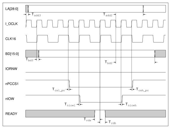
Figure 18-14: 16 MHz Type C write I/O cycle
