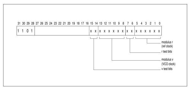
Figure E-2: Frequency Synthesizer Register
