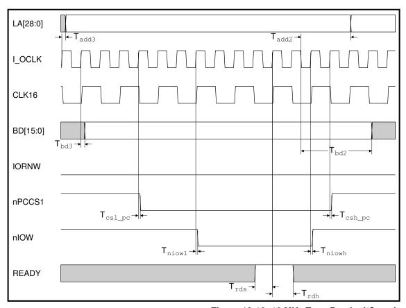
Figure 18-16: 16 MHz Type B write I/O cycle
