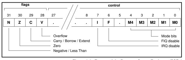
Figure 4-4: Format of the Program Status Registers (PSRs)
