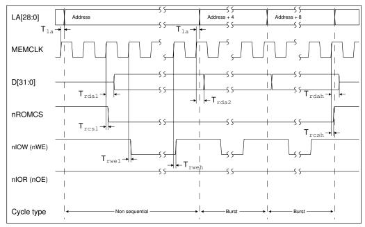
Figure 17-4: ROM write access with burst mode — (32-bit)
