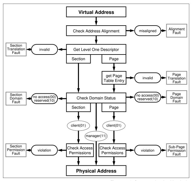
Figure 7-10: Sequence for checking faults
