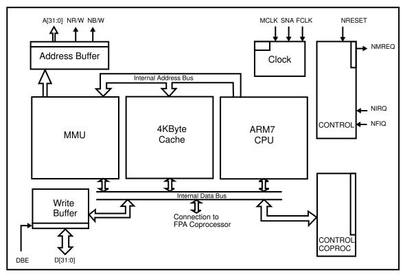
Figure 3-1: ARM processor block diagram
