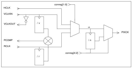
Figure 14-1: ARM7500FE internal subsystems for pixel clock generation
