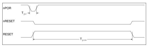
Figure 19-1: nPOR timing diagram
