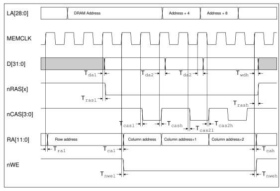
Figure 17-7: Fast page DRAM write timing (32-bit mode)
