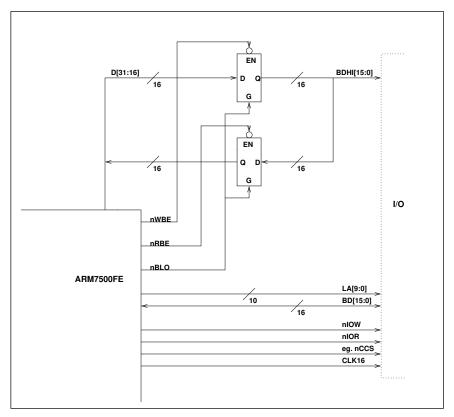
Figure D-1: 32-bit I/O interface
