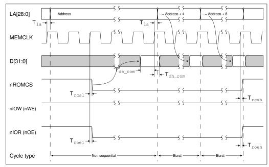
Figure 17-2: ROM read access timing—burst mode (32-bit)
