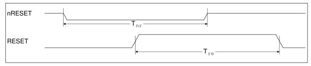
Figure 19-2: nRESET timing diagram
