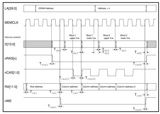
Figure 17-13: EDO DRAM write timing (16-bit mode)
