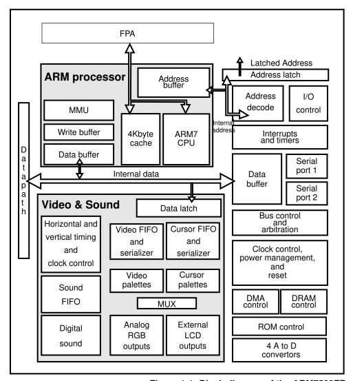
Figure 1-1: Block diagram of the ARM7500FE
