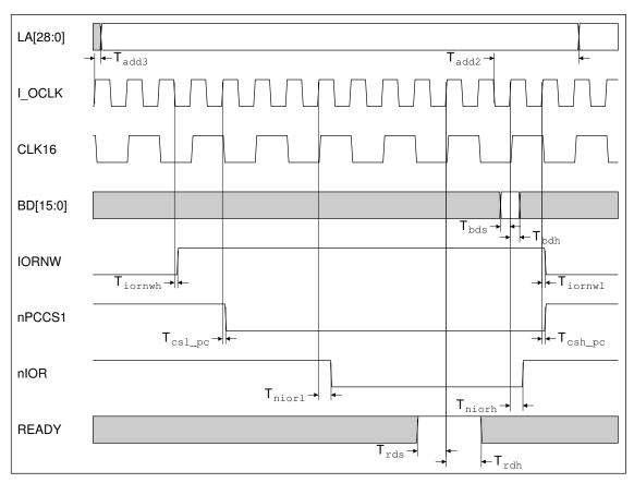
Figure 18-15: 16 MHz Type B read I/O cycle
