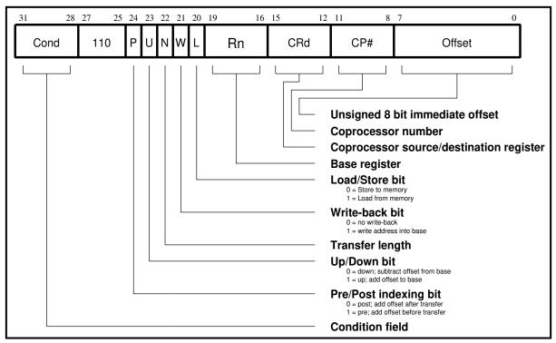
Figure 5-24: Coprocessor data transfer instructions
