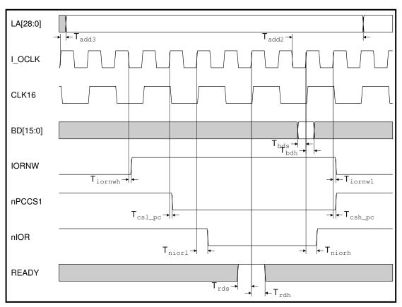
Figure 18-13: 16 MHz Type C read I/O cycle
