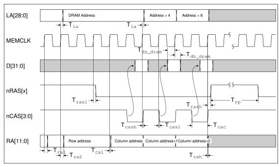
Figure 17-6: Fast page DRAM read timing (32-bit mode)
