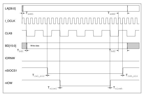
Figure 18-6: 'Medium' 8MHz Simple I/O write cycle timing
