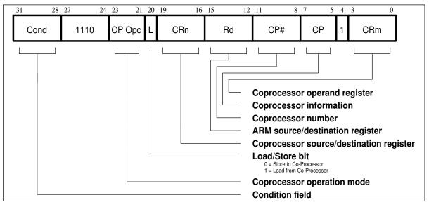
Figure 5-25: Coprocessor register transfer instructions
