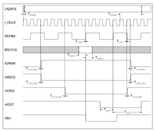
Figure 18-9: 8 MHz Module read I/O cycle
