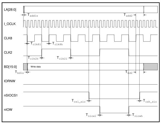
Figure 18-8: 'Sync' 8MHz Simple I/O write cycle timing
