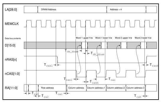
Figure 17-10: Fast page DRAM read timing (16-bit mode)
