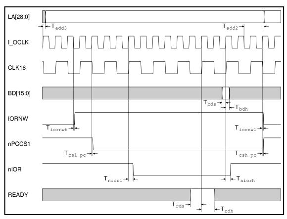
Figure 18-17: 16 MHz Type A read I/O cycle
