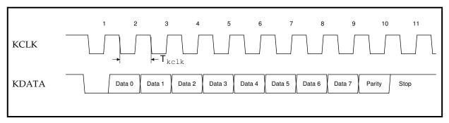
Figure 18-21: ARM7500FE Keyboard/mouse controller receive protocol
