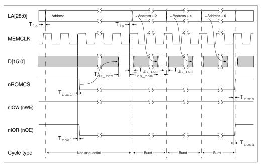
Figure 17-3: ROM read access timing with burst mode—16-bit mode
