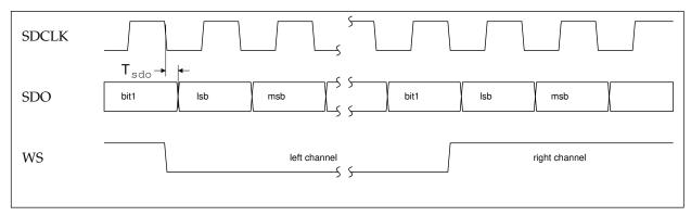
Figure 15-1: Serial sound output — normal format
