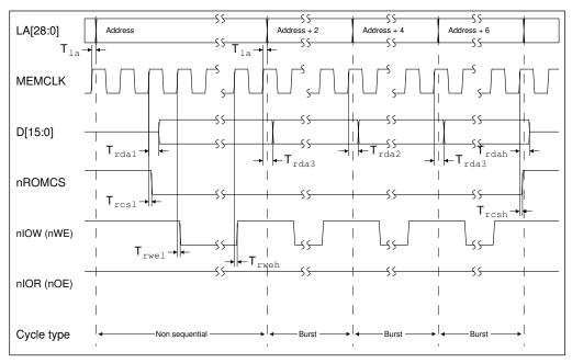
Figure 17-5: ROM write access with burst mode — (16-bit)
