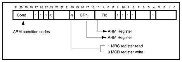
Figure 4-5: Format of Internal Coprocessor Instructions MRC and MCR
