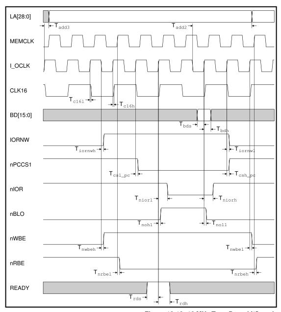
Figure 18-12: 16 MHz Type D read I/O cycle
