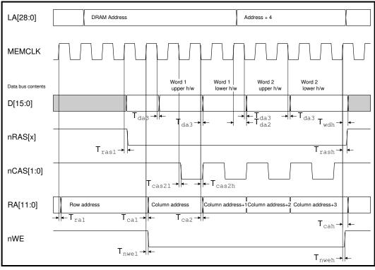
Figure 17-11: Fast page DRAM write timing (16-bit mode)
