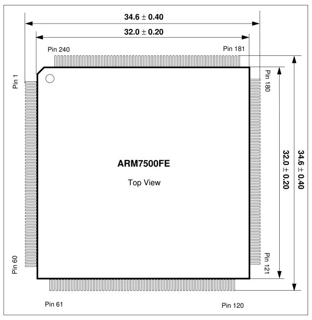
Figure 23-1: Pin diagram for the ARM7500FE
