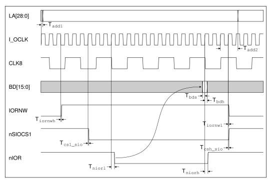
Figure 18-2: 'Medium' 8MHz Simple I/O read cycle timing
