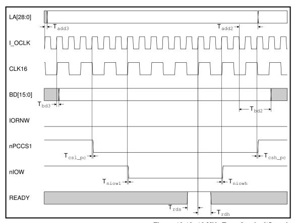
Figure 18-18: 16 MHz Type A write I/O cycle
