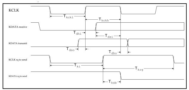
Figure 18-22: Keyboard/mouse interface timing
