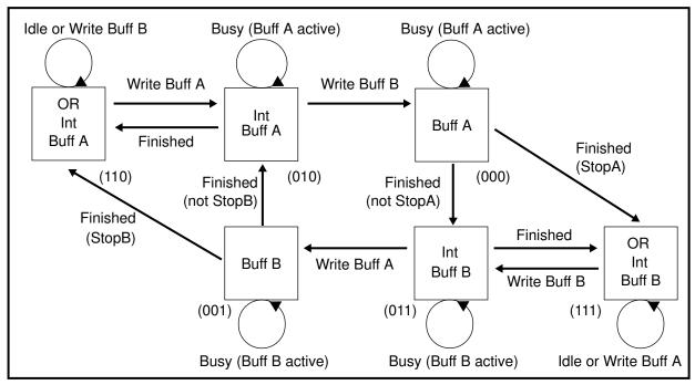
Figure 17-16: Hardware DMA state machine diagram
