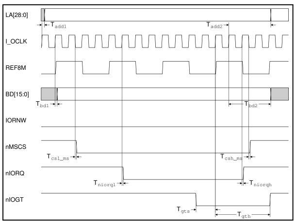
Figure 18-10: 8 MHz module write I/O cycle
