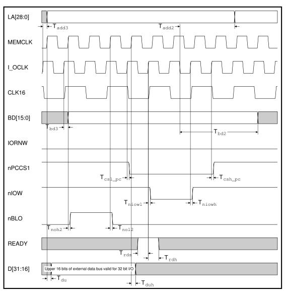
Figure 18-11: 16 MHz Type D write I/O cycle
