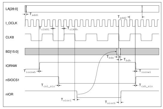
Figure 18-1: 'Fast' 8MHz Simple I/O read cycle timing
