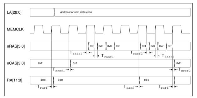
Figure 14-8: Refresh cycle timing
