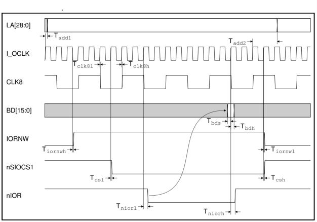
Figure 15-1: 'Fast' 8MHz Simple I/O read cycle timing
