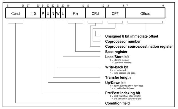
Figure 5-24: Coprocessor data transfer instructions
