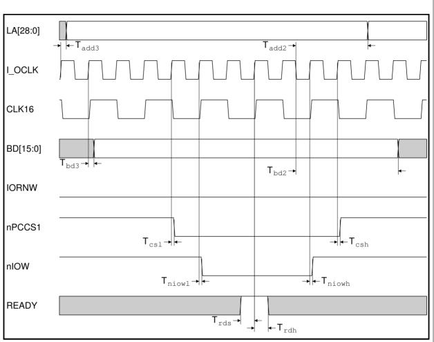
Figure 15-14: 16 MHz Type C write I/O cycle
