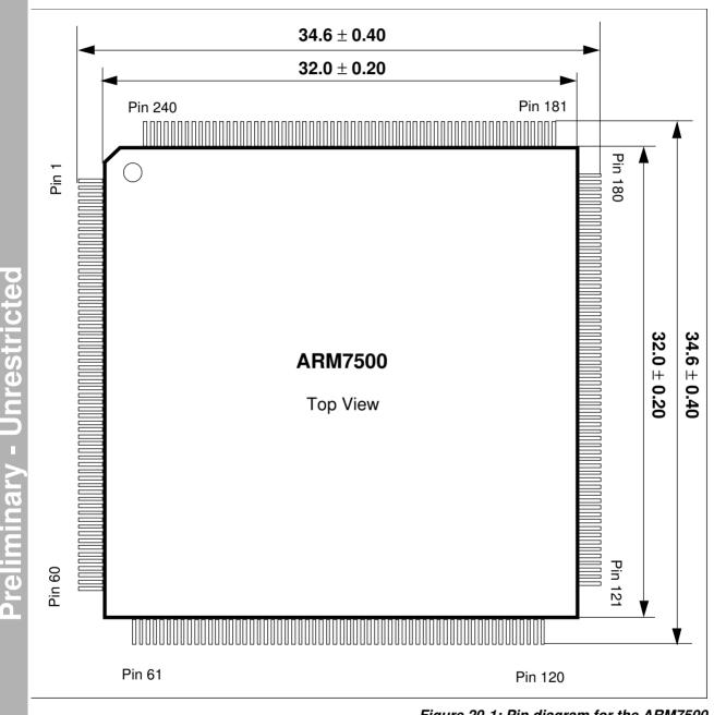
Figure 20-1: Pin diagram for the ARM7500
