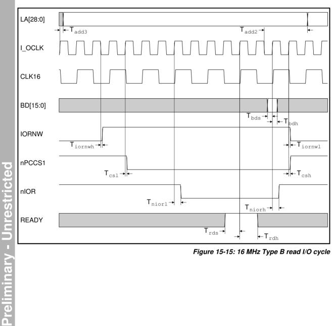
Figure 15-15: 16 MHz Type B read I/O cycle
