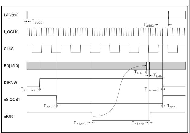
Figure 15-3: 'Slow' 8MHz Simple I/O read cycle timing
