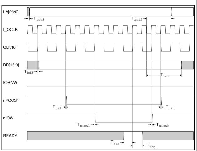
Figure 15-16: 16 MHz Type B write I/O cycle
