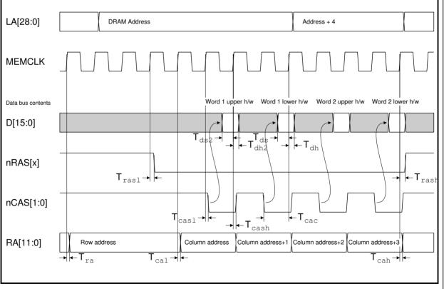
Figure 14-6: DRAM read timing (16-bit mode)
