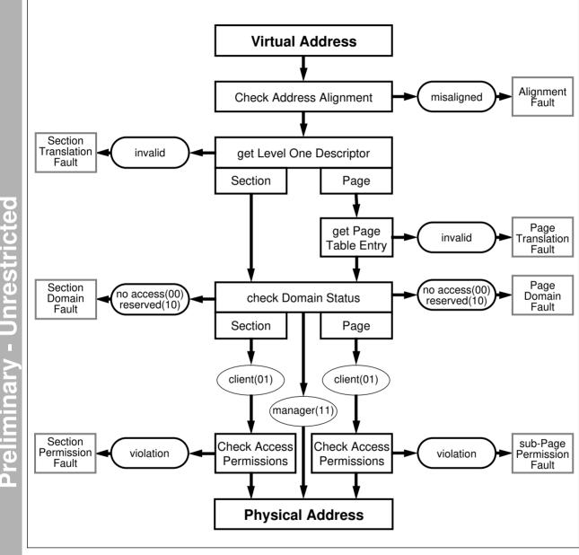
Figure 7-10: Sequence for checking faults
