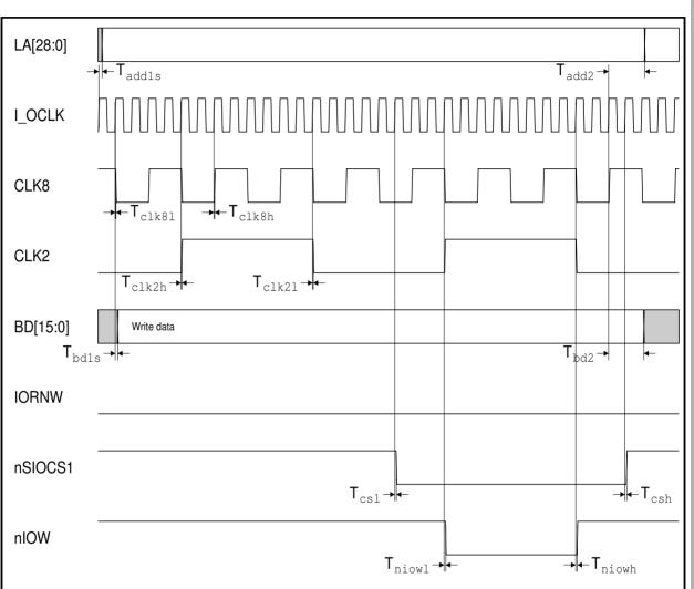
Figure 15-5: 'Fast' 8MHz Simple I/O write cycle timing
