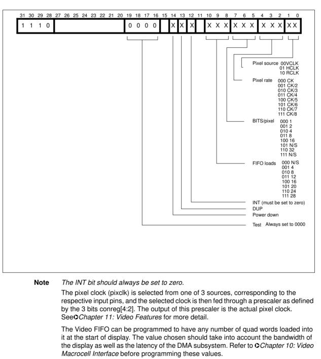
Setting the dup bit configures the display for dual-panel LCDs. This is described further in OChapter 11: Video Features.
