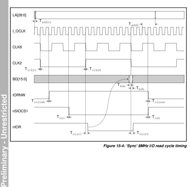
Figure 15-4: 'Sync' 8MHz I/O read cycle timing
