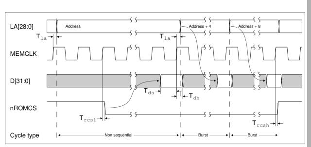
Figure 14-2: ROM access timing—burst mode (32-bit)
