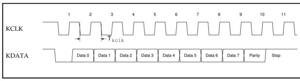
Figure 15-21: ARM7500 Keyboard/mouse controller receive protocol
