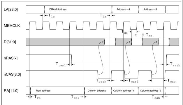
Figure 14-4: DRAM read timing (32-bit mode)
