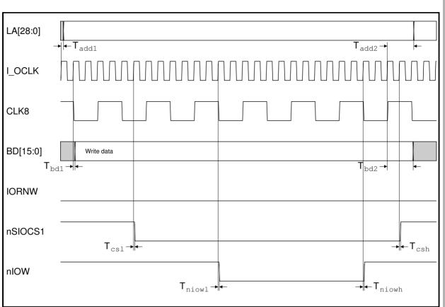
Figure 15-7: 'Slow' 8MHz Simple I/O write cycle timing
