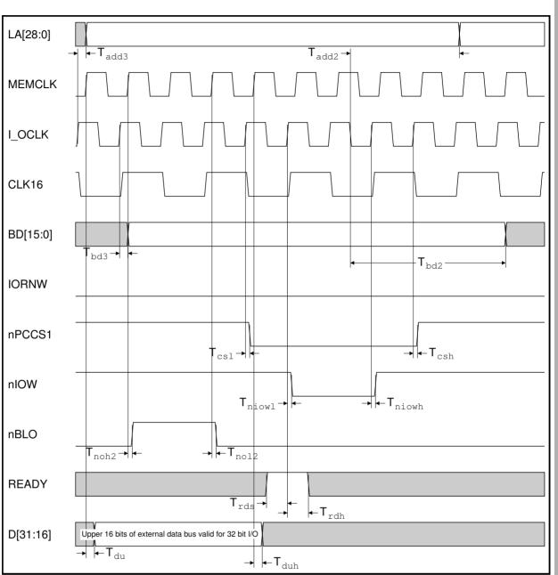
Figure 15-12: 16 MHz Type D write I/O cycle
