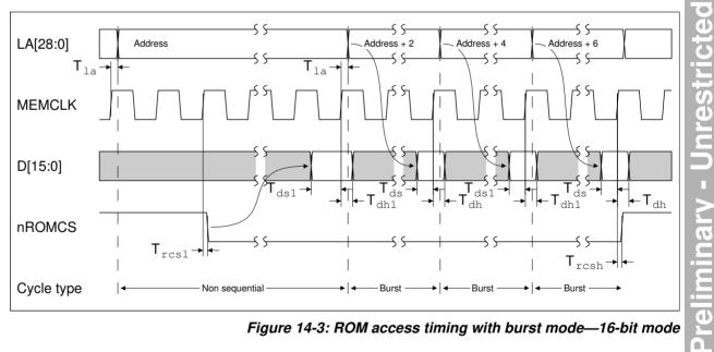
Figure 14-3: ROM access timing with burst mode—16-bit mode
