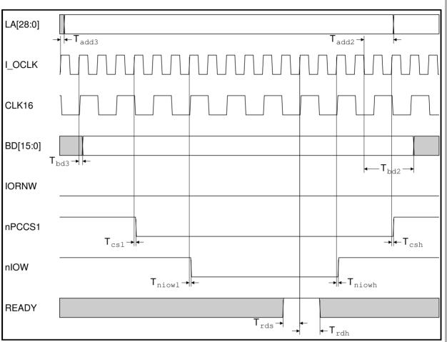
Figure 15-18: 16 MHz Type A write I/O cycle
