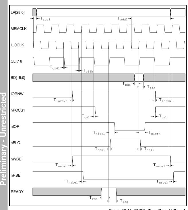
Figure 15-11: 16 MHz Type D read I/O cycle
