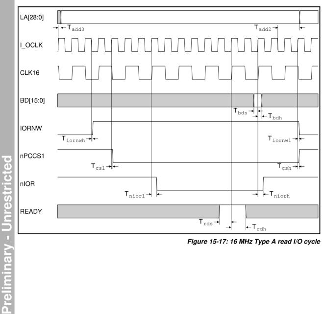
Figure 15-17: 16 MHz Type A read I/O cycle
