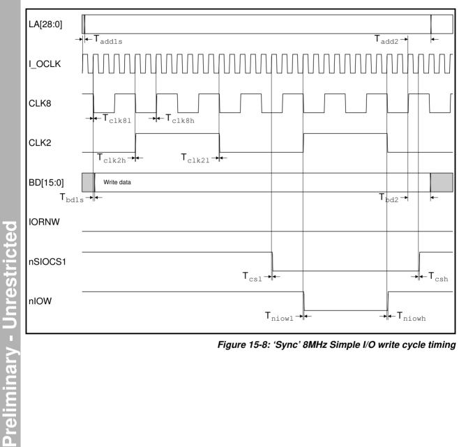
Figure 15-8: 'Sync' 8MHz Simple I/O write cycle timing
