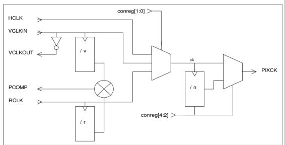
Figure 11-1: ARM 7500 internal subsystems for pixel clock generation
