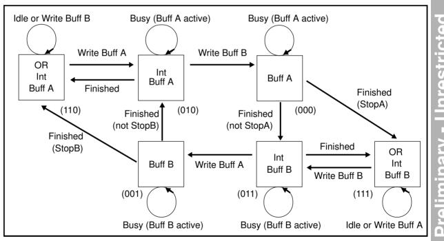
Figure 14-9: Hardware DMA state machine diagram
