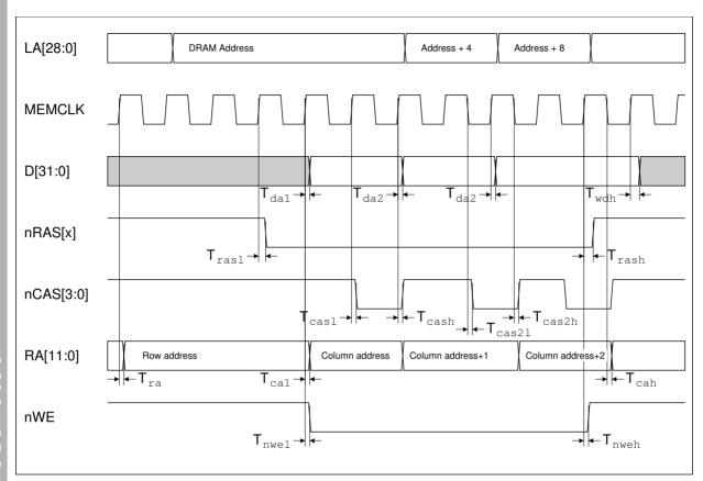
Figure 14-5: DRAM write timing (32-bit mode)
