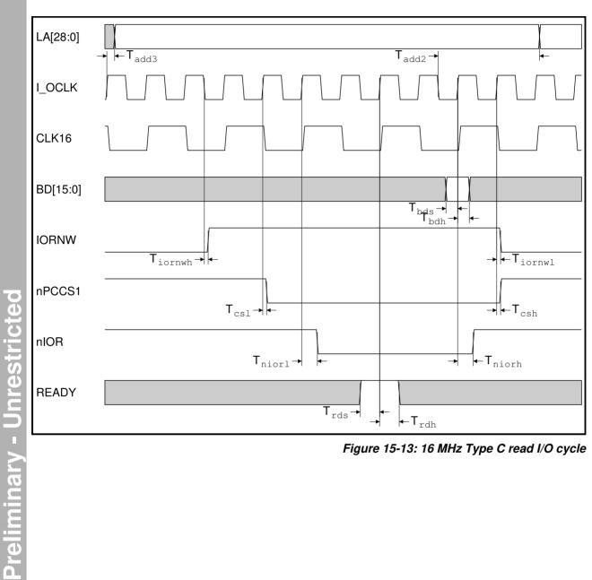
Figure 15-13: 16 MHz Type C read I/O cycle
