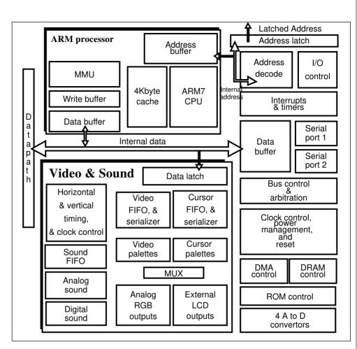
Figure 1-1: Block diagram of ARM7500
