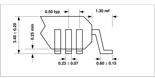
Figure 20-2: Side view of ARM7500 chip
