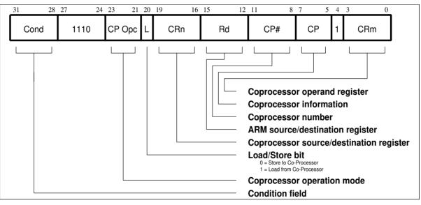
Figure 5-25: Coprocessor register transfer instructions
