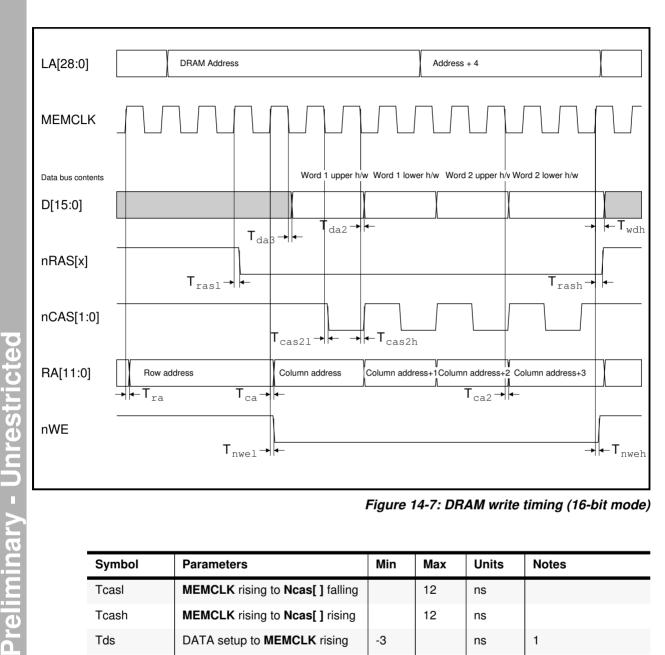
Figure 14-7: DRAM write timing (16-bit mode)
