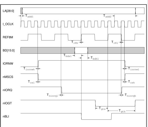
Figure 15-9: 8 MHz Module read I/O cycle
