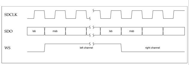
Figure 12-3: Serial sound interface—Japanese format
