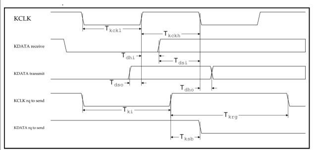
Figure 15-22: Keyboard/mouse interface timing
