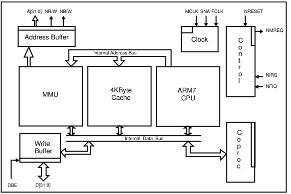
Figure 3-1: ARM processor block diagram
