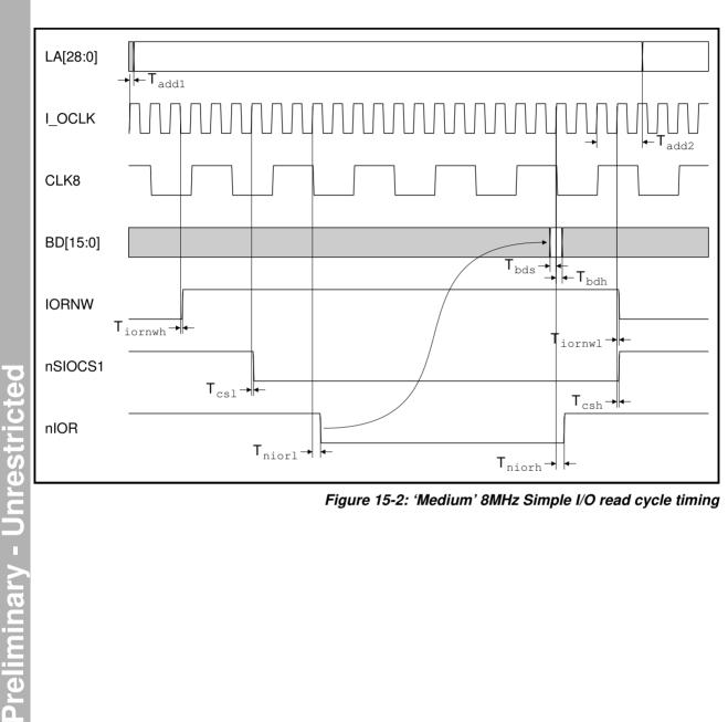
Figure 15-2: 'Medium' 8MHz Simple I/O read cycle timing
