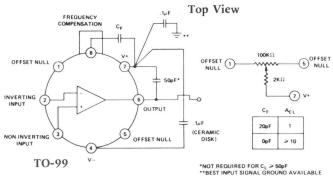
are supplied in the TO-99 package for operation over the 0 to  $+70^{\circ}$ C temperature range. The AD507S is specified for operation from  $-55^{\circ}$ C to  $+125^{\circ}$ C.
