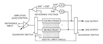
Diagram Showing the Principle of the DSC1605
