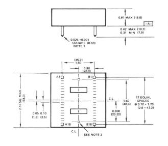
Figure 13. SMX1004 and SCL1006 (Note that Pins A1, A2, A3, A16, A17, A18, B1, B2, B3, B16, B17, and B18 are omitted on the SCL1006.)
