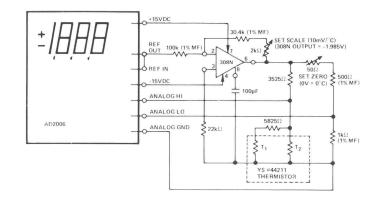
AD2006 Thermistor Temperature Measurement System
