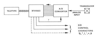
Figure 1. STX1003 Serial Transmitter (For details of this system, request SERDEX Note 1 "Interfacing the teletype with . . . ADC1100 A/D converter")
