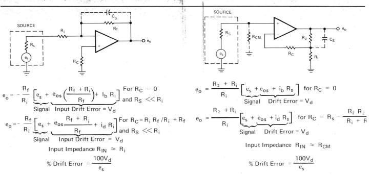
Figure 1A. Inverting Configuration
