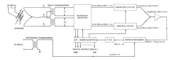
Block Schematic for "SDC" Series Converters
