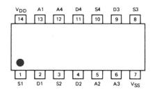
PACKAGE INFORMATION Suffix D – Ceramic DIP Suffix N – Plastic DIP Suffix H – TO-100 AD7519
