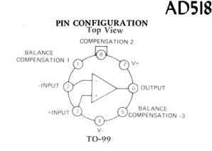
The high slew rate, fast settling time, ease of use, and low cost of the AD518 make it ideal for use with the D/A and A/D converters, as well as active filters, sample and hold circuits, and as a general purpose amplifier. The AD518 is supplied in the TO-99 package. The AD518J and AD518K are specified for operation over the 0 to  $+70^{\circ}$ C temperature range; the AD518S for operation from  $-55^{\circ}$ C to  $+125^{\circ}$ C.
