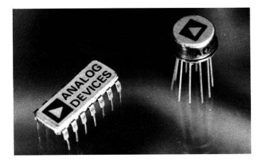
unity gain slew rate of  $50V/\mu$ sec, a typical bandwidth of 10MHz and laser-trimmed offset voltage down to 1mV max.
