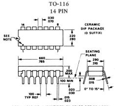
NOTE: LEAD NO. 1 IDENTIFIED BY COLOR DOT OR NOTCH MECHANICAL INDEX POINT OR NOTCH IN PIN.
