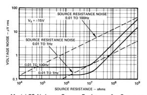
Model 52 Noise vs. Source Resistance for Constant Bandwidth
