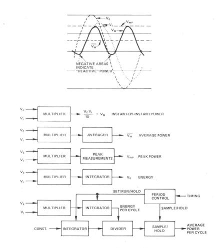
Figure 1. Multiplier Applications for Power and Energy Measurements
