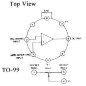
This circuit has excellent dynamic performance, with a typical slew rate of  $6V/\mu$ sec, and is supplied in the TO-99 package for operation from 0 to  $+70^{\circ}$ C and  $-55^{\circ}$ C to  $+125^{\circ}$ C.
