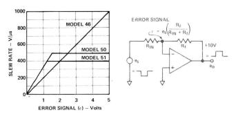
Figure 2. Slew Rate vs. Error Signal
