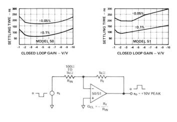
Figure 1. Settling Time vs. Gain (V/V)
