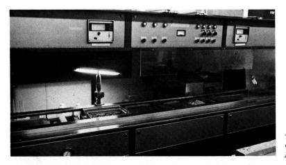
This automatic wave soldering machine complements other facets of our manufacturing facilities geared for volume with quality.
