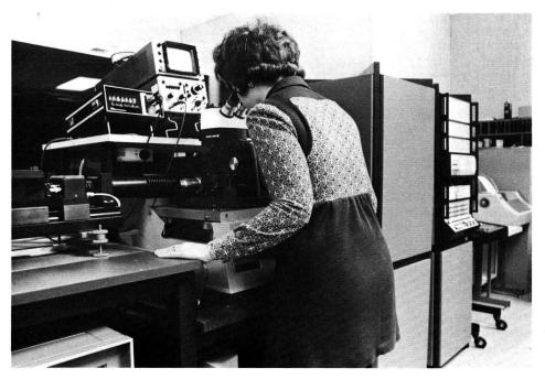
Our proprietary thin-film-on-silicon trimming process allows precise tailoring of integrated circuit element values prior to final encapsulation. Computerized laser trimming of our IC multipliers, op amps, and converters enhances their accuracy, but decreases their cost.
