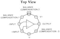
The high slew rate, wide bandwidth, and low input currents of the AD528 make it ideal for use in sample-hold circuits, A/D, D/A and sampled data systems, and high speed integrators. The AD528 is supplied in the TO-99 package. The AD528J and AD528K are specified for operation over the 0 to  $+70^{\circ}$ C temperature range; the AD528S for operation from -55 to  $+125^{\circ}$ C.
