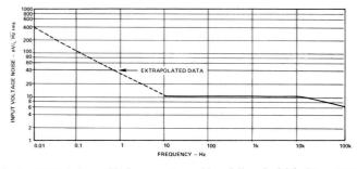
Model 606 Voltage Noise per Root Hz of Bandwidth (G = 1000)
