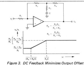
Figure 3. DC Feedback Minimizes Output Offset for AC Applications
