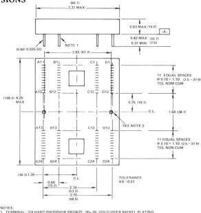
NUTES: 1. TERMINAL: 3/4 HARD PHOSPHOR BRONZE, 30µ IN. GOLD OVER NICKEL PLATING. 2. MOUNTING HOLES: THREADED TO ACCEPT A #6-32, THREAD DEPTH 0.375 MAX (9.53) FROM SUBFACE - A-
