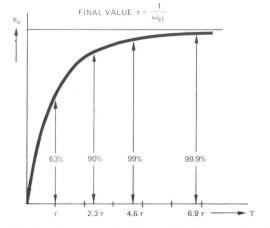
Figure 5. Step Response for Linear 6dB/Octave Amplifier
