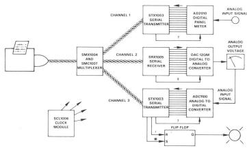
Figure 4. Self-Multiplexed Analog Output. Several D/A converters with registers are connected in parallel to one SRX1005. The %, !, or \* strobes the input register of the desired D/A converter. Figure 6. A Complex 3-channel Data Acquisition and Control System. To read the analog input signal, the operator would type #1? and wait for print-out of the data. To set the output voltage at mid-scale, he would type #2 = 500\$. Likewise,  $\#3^*$ would turn on the light
