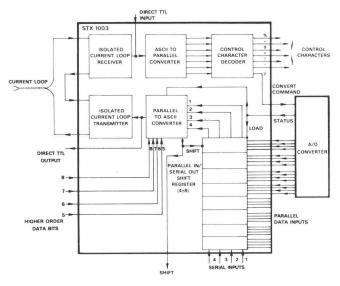
Figure 9. Block Diagram of the STX1003 Serial Transmitter
