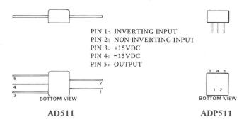
operation over the  $-25^{\circ}$ C to  $+85^{\circ}$ C temperature range. The AD511 is supplied in the end-lead mini-package; the ADP511 in the bottom-lead mini-package.
