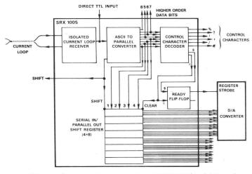
Figure 10. Block Diagram of the SRX1005 Serial Receiver
