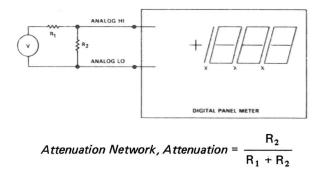
Resistors used in attenuator networks should be chosen for temperature coefficients at least twice as good as the DPM to avoid any additional temperature effects. In addition, keeping the source loading of the DPM below  $10k\Omega$  will minimize the effects of bias current changes due to temperature.
