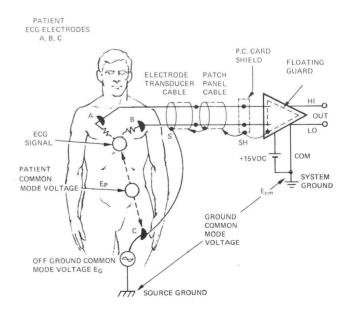
Figure 13. Patient-Amplifier Interconnection Diagram
