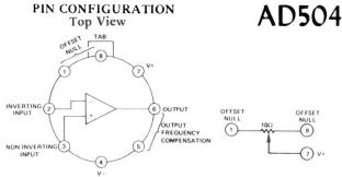
tected from short circuits to ground and/or either supply voltage, and is capable of driving 1000pF of load capacitance. The J, K, L, and M models are specified for operation over the 0 to +70°C temperature range, and are supplied in the TO-99 can package. The S version, in the same package, is specified for -55°C to +125°C operation.
