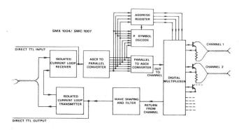
Figure 11. Block Diagram of a SMX1004/SMC1007 Multiplexer
