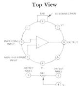
All versions of the AD514 are supplied in the hermeticallysealed, 8-pin, TO-99 package. The AD514J, K and L are specified for 0 to  $+70^{\circ}$ C applications, while the AD514S is offered for operation over the full military temperature range of -55 to  $+125^{\circ}$ C.
