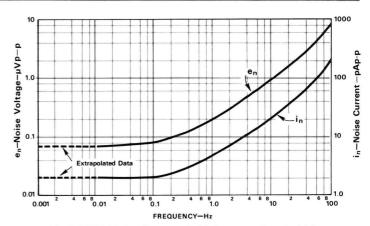
Model 261 Noise Current & Voltage vs. Bandwidth Measured from 0.01Hz
