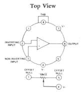
All versions of the AD540 are supplied in the hermeticallysealed, 8-pin, TO-99 package. The AD540J and AD540K are specified for 0 to +70°C applications, while the AD540S is offered for operation over the full military temperature range of -55 to  $+125^{\circ}$ C.
