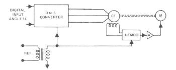
Servo Using D to S Converter
