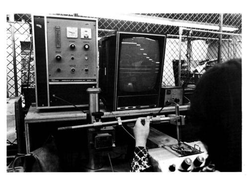
Active abrasive trimming trims the resistor networks in our modular converters while the units are under power and operating. The precision of this trimmer, which we designed, allows high performance units to be built at a rate required for budget pricing.
