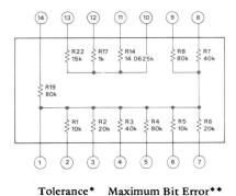
Max. Pwr. **Ratio Accuracy** Nominal REF. Dissipation L (U) R Value (Ohms) R (mW) 1/8LSB of 12 Bits 10k 1 20 ±0.3% Abs. 2 20k R1 10 0.015% 3 40k R1 0.03% 5 4 80k R1 2.5 0.05% 5 10k R1 20 0.10% 6 20k R1 10 0.2% 7 40k R1 5 0.4% 8 80k R1 2.5 0.8% 14 14.0625k R17 0.5 0.05% 17 1k 8 ±0.5% Abs 19 80k R1 2.5 0.20% 22 15k R17 0.5 0.50%
