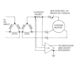
Figure 4. Motor Current Shunt Monitor
