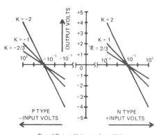
Plot of Output Voltage vs Input Voltage When Connected in Log Mode
