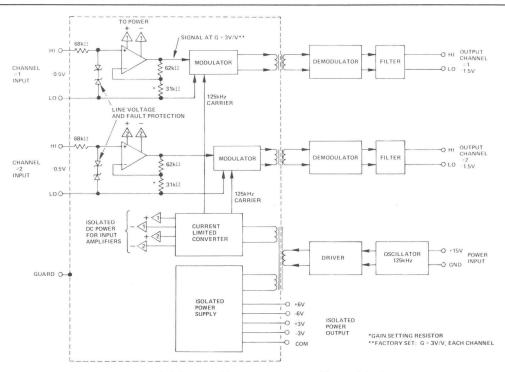
Figure 3. Block Diagram, Model 282J, Two Channel Isolator
