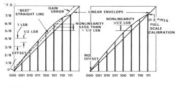
a. %LSB Nonlinearity Achieved By Arbitrary Location of "Best Straight Line". b. Nonlinearity Reference is Straight Line Through End Points. Nonlinearity >½LSB for Curve of a.
