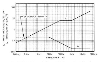
Model 230 Voltage & Current Noise per Root Hz of Bandwidth
