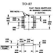
NOTE: LEAD NO. 1 IDENTIFIED BY COLOR DOT, MECHANICAL INDEX POINT OR NOTCH IN PIN.
