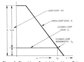
Figure 4. Closed Loop Bandwidth and Loop Gain
