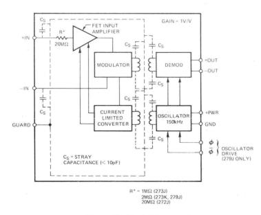
Figure 12. Block Diagram of Unity Gain Isolation Amplifiers
