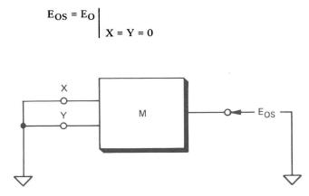
NOISE is specified and measured with both inputs at zero signal and zero impedance (i.e., shorted). For low frequency applications, filtering the output of the multiplier may improve small signal resolution significantly.
