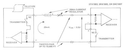
Figure 8. Each teletype serial character consists of one start bit, seven ASCII-coded data bits, a parity bit, and two stop bits. Prior to transmitting a character, all loop switches are closed and 20mA flows. A start bit, followed by the data bits, is transmitted by operating one of the transmitter switches. The receiver amplifiers detect the presence or absence of loop current.
