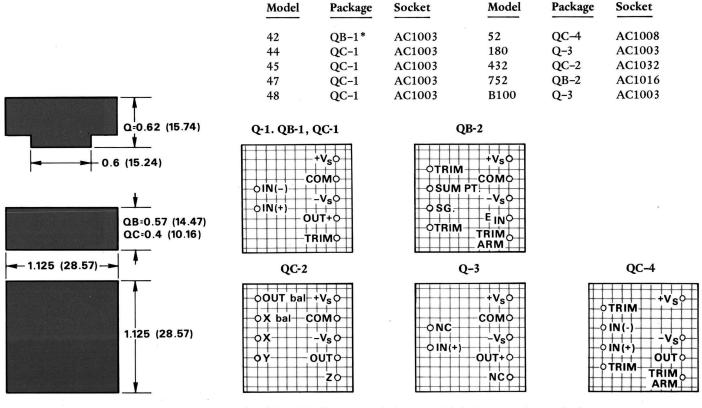
\*Model 42 (QB-1) common pin is not provided. No connection required.
