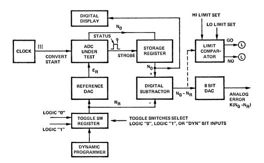
Figure 23. ADC test configuration.
