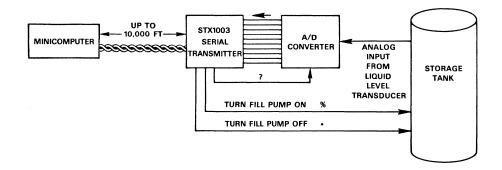
Figure 25. Application of the STX1003 Serial Transmitter.
