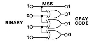
Figure 3. Binary to Gray code conversion using exclusive – or gates.
