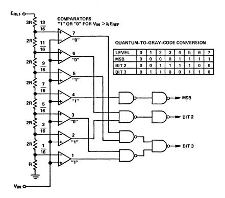
Figure 29. Parallel 3-bit A/D converter with Gray code output.
