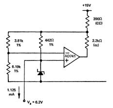
Figure 9. Constant-current excitation of precision reference Zener diode.
