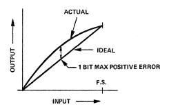
(a) Gain adjusted for zero full-scale error.
