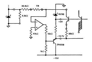
Figure 11. Reference circuit using inverting input.
