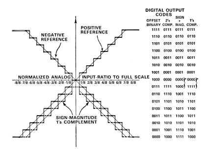
Figure 7. Ideal A/D conversion relationship for 4-bit (3-bit-plus-sign) offset binary, 2's complement, sign magnitude, 1's complement codes.
