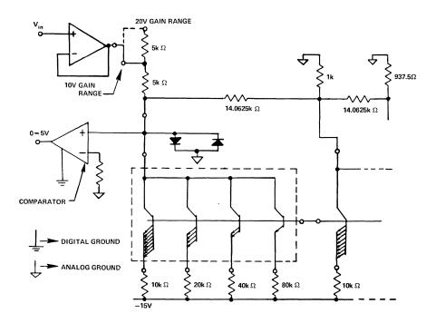
Figure 17. ADC using comparator in the current mode.
