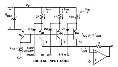
Figure 19. D/A converter using basic current switching technique.
