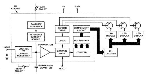
Figure 43. AD2026 block diagram.
