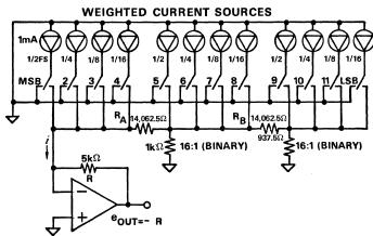
Figure 20. Block diagram of 12-bit current-switching D/A converter, showing weighted attenuation of quad output currents for binary coding. For BCD,  $R_A$  and  $R_B$  become 8,132.5 $\Omega$  and 8,437.5 $\Omega$ , and R becomes  $4k\Omega$ , and the interguad attenuations are 10:1.
