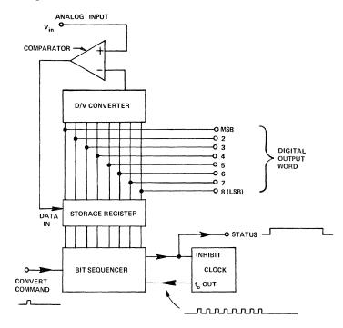
Figure 15. Block diagram of successive-approximations A/D converter.
