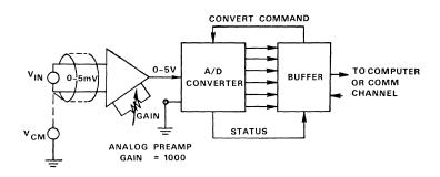
Figure 3. A/D Converter with preamplifier.
