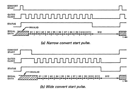
Figure 50. Effect of convert-start pulse-width on timing.
