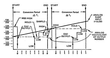
4b. Successive-approximations converter example of Figure 2, preceded by sample-hold. Digital output is within ½LSB of analog input at start of conversion, 124/256, and 127/256.
