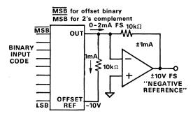
Figure 22. Bipolar connection of current-swtiching D/A converter for offset binary or 2's complement codes.
