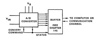
Figure 1. Simplest data-acquisition system configuration.
