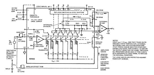
Figure 36. Functional schematic of the AD562.
