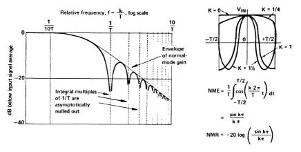
b. Worst-cast normal-mode response of dual-slope A/D converter.
