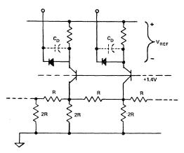
Figure 4. Diode switching in D/A converter.
