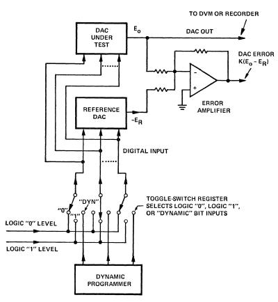
Figure 8. Basic DAC tester.
