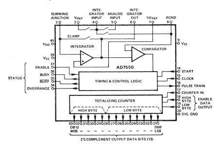
Figure 32. Block diagram of the AD7550 A/D converter.
