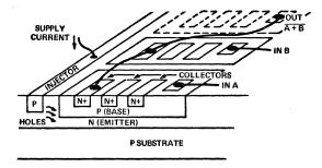
Figure 45b. Sectional view of I<sup>2</sup> L circuit.
