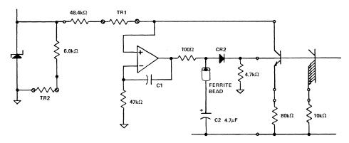
Figure 12. Reference cirucit with frequency shaping and anti-latchup circuit.
