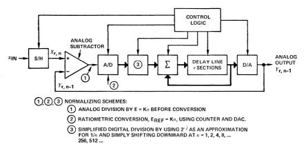
Figure 6. Waveform averaging by addition using normalized variables.
