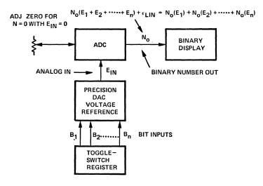
(b) A/D converter test.
