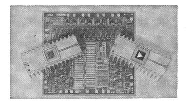
The AD7570 will accurately digitize signals having full-scale ranges from nearly  $\pm 25V$  down to levels limited only by the comparator's ability to detect submillivolt changes. This is a direct consequence of the use of a highly linear on-board multiplying D/A converter (close-ly related to the AD7520), which can accept a wide range of reference voltage. Normal operation is specified with 10V reference.
