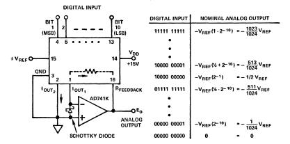
Figure 13. The AD7520 as a unipolar binary digital to voltage converter (2-quadrant multiplier).
