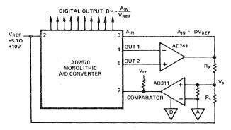
Figure 31. Direct resistance measurement. Digital output is equal to the ratio of  $R_x$  to  $R_s$ , independently of  $V_{REF}$ .
