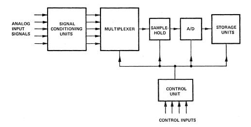
*Figure 5. Data-acquisition system with sample-hold and input pre-conditioning.*
