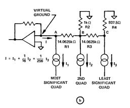
Figure 8a. Current attenuation to 1/16.
