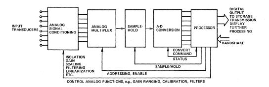
Figure 1. Data-acquisition function.
