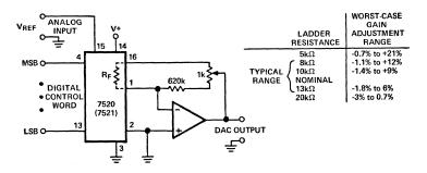
Figure 19. Single-control trim for gain calibration, allowing for a large range of absolute ladder-resistance variation.
