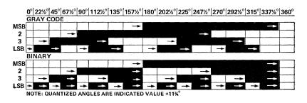
Figure 5. Gray vs. binary encoding.
