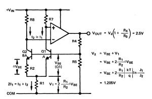
Figure 9. Basic bandgap-reference regulator circuit.
