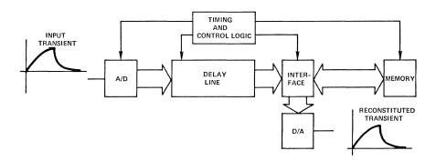
Figure 3. Transient recorder.
