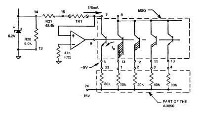
Figure 10. Reference circuit using non-inverting amplifier input.
