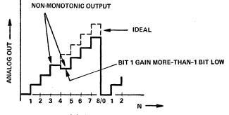
(c) Non-monotonicity. Figure 6. DAC differential linearity and monotonicity errors.
