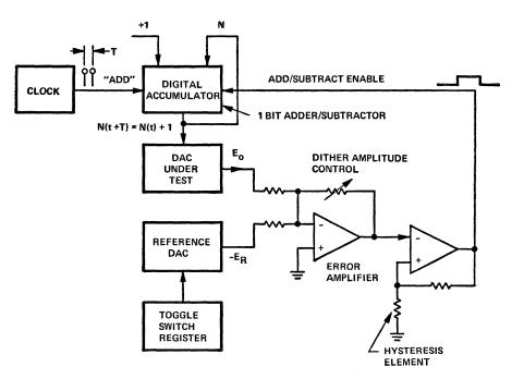
Figure 16. Closed-loop digital dither generation.
