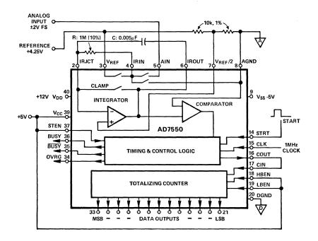
Figure 4. AD7550 connections for basic operation.
