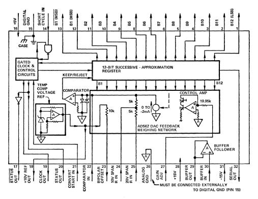
Figure 46. AD572 functional diagram & pinout.
