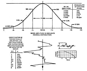
Figure 15. RMS vs. peak-to-peak amplitudes for gaussian noise.
