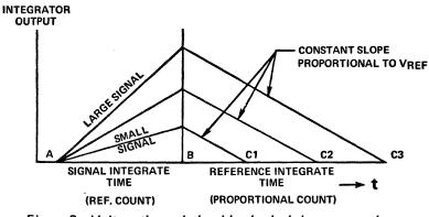
Figure 3. Voltage-time relationships in dual-slope conversion.
