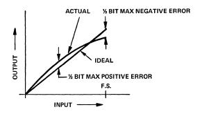
(b) Gain adjusted to minimize peak error. Figure 3. Effect of gain adjustment on linearity error for nonlinear DAC or ADC.
