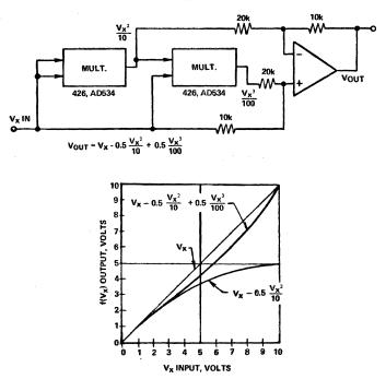
Figure 5c. Using multipliers for nonlinear functional realtionships (such as linearization).
