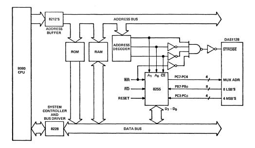
Figure 11. Interfacing a DAS1128 to an 8080 microprocessor.
