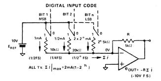
Figure 1. Elementary D/A converter circuit.
