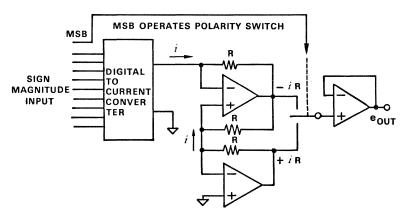
Figure 24. Sign-magnitude bipolar D/A conversion using unipolar DAC and switched outputs of operational amplifiers.
