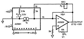
Figure 39. Connecting the AD561 for buffered 0V to +10V output. The adjustment pot may be replaced by a fixed  $25\Omega$  resistor for 10mV typical output error.
