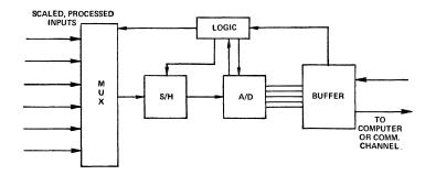
Figure 8. Multi-channel analog multiplexed interface.
