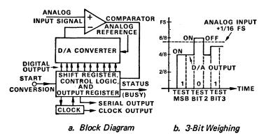
Figure 26. Successive-approximation A/D converter.
