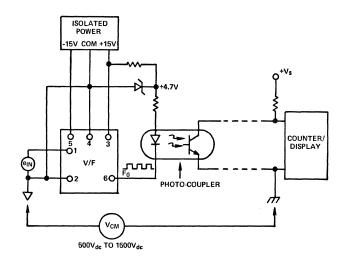
Figure 19. Optically-isolated A-D conversion.
