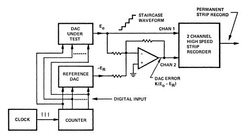
Figure 11. DAC dynamic test - COUNT mode.
