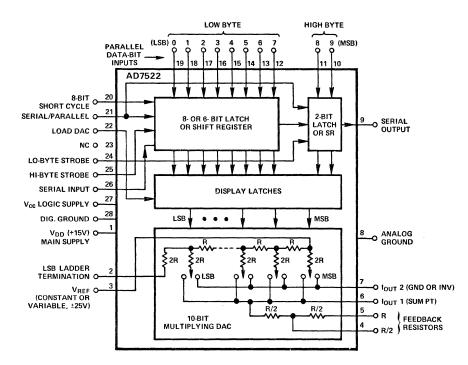
Figure 2. Functional diagram of the AD7522.
