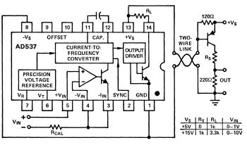
THE AD537 CAN BE USED FOR TRUE TWO-WIRE OPERATION, AS SHOWN HERE. THE FREQUENCY INFORMATION IS TRANSMITTED AS A CURRENT SIGNAL ON THE SUPPLY LINE TO THE DEVICE. THE SIGNAL IS CONVERTED TO A DTL/TL OR CMOS-COMPATIBLE SIGNAL BY THE SINGLE-TRANSISTOR-TERMINATION CIRCUIT SHOWN. THE EXCELLENT SUPPLY REJECTION, HIGH OUTPUT-DRIVE CAPABILITY AND SQUARE-WAVE OUTPUT FROM THE AD537 ARE ALL ADVANTAGEOUS IN THE APPLICATION.
