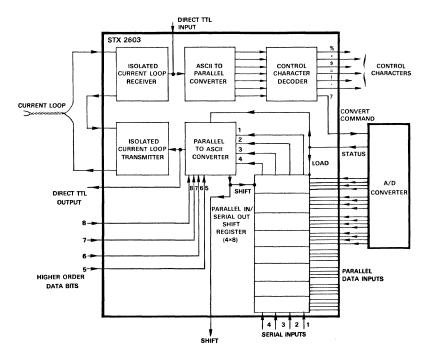
Figure 24. Block diagram of the STX2603 serial transmitter.
