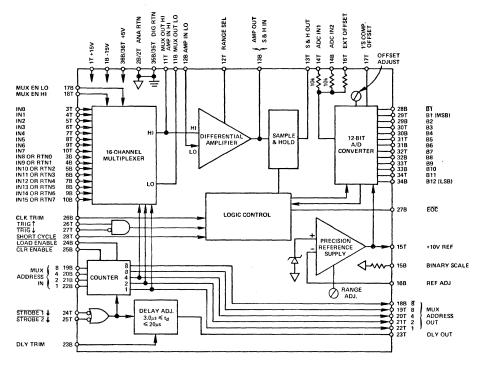
Figure 5. Block diagram of the DAS1128 data-acquisition subsystem.
