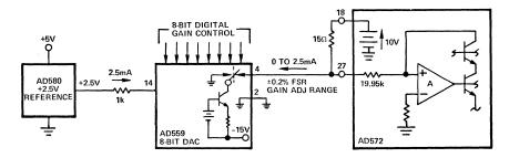
Figure 51. Digital gain control using 8-bit DAC.
