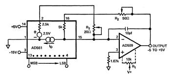
Figure 40. Connections for buffered  $\pm 5V$  output. Adjustment pots may be replaced by mid-range resistances with 10mV typical error.
