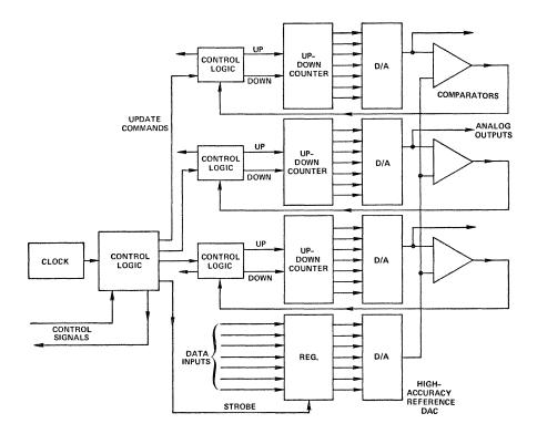
Figure 6b. Low-cost high-accuracy distribution.
