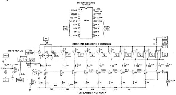
Figure 6. AD561 D/A converter: Schematic and connection diagrams.
