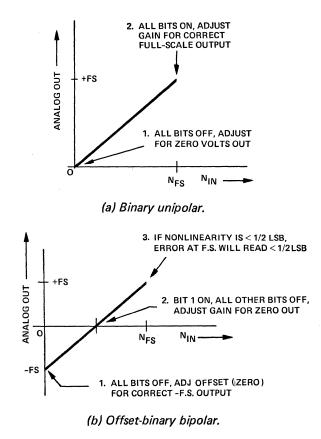
Figure 4. Typical DAC calibration procedure.
