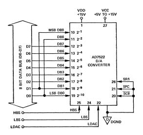
Figure 26. AD7522 - Connection for 2 byte operation.
