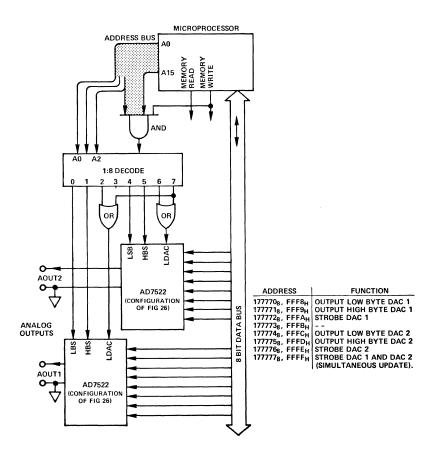
Figure 27. Interfacing multiple AD7522's to a microprocessor.
