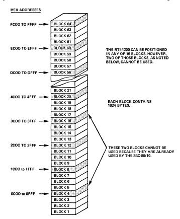
Figure 14. Positioning the RTI-1200 in the SBC-80/10's memory address space.
