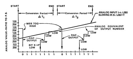
Figure 2. Successive-approximations converter error with fastchanging input (2%LSB per conversion interval). Note that output reading of 127/256 FS is the same for both intervals, though one starts at 124/256 and the other ends at 129/256. Error increases with ramp speed.
