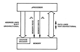
Figure 10. A microprocessor is a memory-controller.
