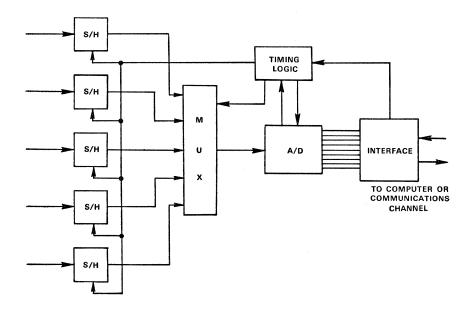
Figure 7. Multiplexed simultaneous sample system.
