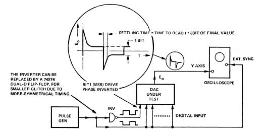
Figure 19. DAC major-carry settling-time measurement.
