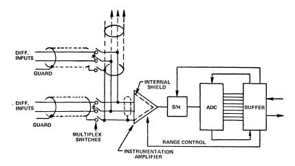
Figure 9. Low-level multiplexing.
