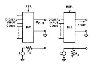
Figure 11. Digital-to-analog converters as voltage or current generators.
