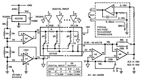
Figure 17. Single-supply 10-bit DAC circuit.
