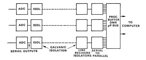
Figure 6b. Multi-channel conversion using remote A/D converters.
