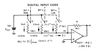
Figure 14. Simple D/A converter.
