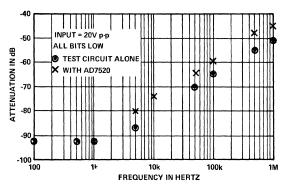
Figure 18. AD7520 feedthrough measurement.
