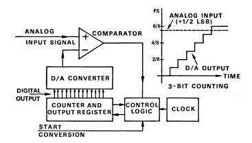
Figure 28. Counter-comparator A/D converter.
