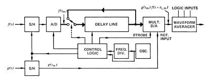
Figure 8. Real-time correlation using delay line.
