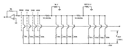
Figure 3. D/A converter using binary-weighted quad current sources.
