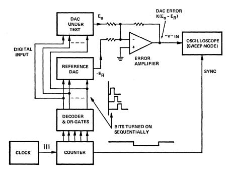
Figure 9. DAC dynamic test - BIT-SCAN mode.
