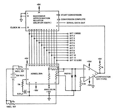
Figure 38. 12-bit successive approximation A/D converter.
