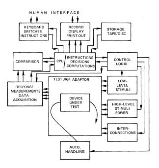
Figure 1. Test system ingredients in typical configuration.
