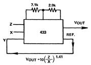
Figure 5d. Ratio of two voltages raised to arbitrary nonintegral power.
