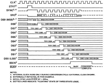
CROSS HATCHING INDICATES "DON'T CARE" STATE. SET AND RESET OF OUTPUT DATA BITS LAGS CLOCK POSITIVE EDGE BY  $\approx 200 ns.$
