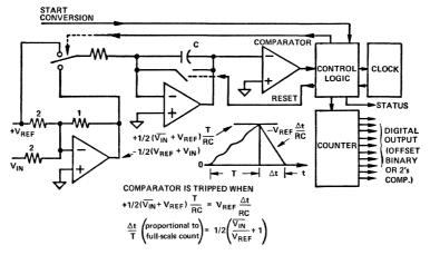
a. Dual-ramp A/D converter for bipolar input.
