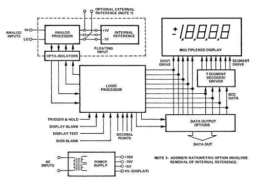
Figure 3. AD2008 block diagram
