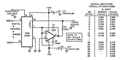
Figure 20. Inexpensive, high-performance gain control.
