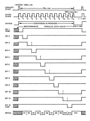
Figure 47. Timing diagram (binary code 110101011001)
