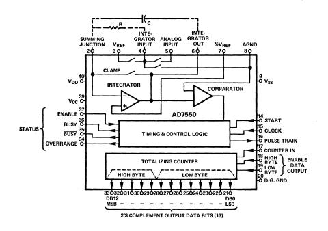
Figure 2. Block diagram of the AD7550 A/D converter.
