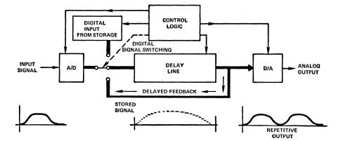
Figure 4. Recirculating delay line.
