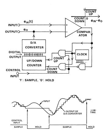
For slowly-varying analog signals, the tracking sample-hold is one of the lowest-cost ways to convert, since it eliminates the need for a sample-hold. However, its conversion time is variable, which introduces timing errors in sampled-data systems, since the most-recently acquired value may represent any value of signal during the interval between interrogations. Also, its response depends to a great extent on the amount and type of noise present.
