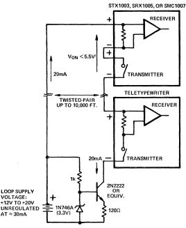
Figure 22. 20mA current loop data transmission.
