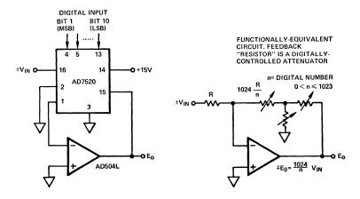
Figure 16. An analog-digital divider.
