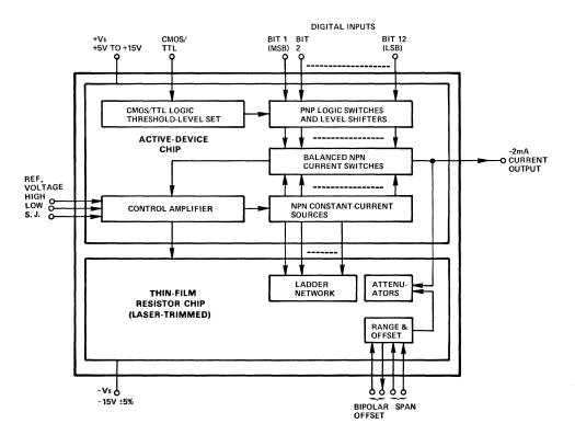
Figure 5. Functional block diagram of the AD562.
