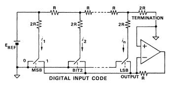
Figure 18. Inverted R-2R ladder in current-switching mode.
