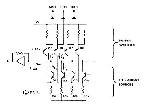
Figure 5. Buffered switches in D/A converter.
