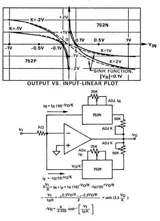
Figure 14. Bipolar signal compression using complementary logarithmic transconductors to synthesize sinh<sup>-1</sup> function.
