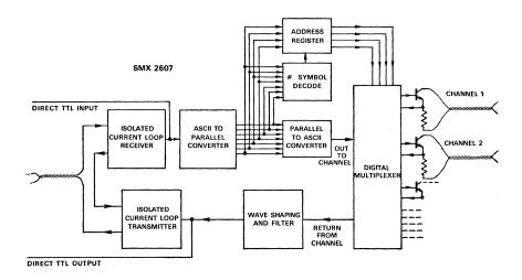
Figure 27. Block diagram of a SMX2607 multiplexer.
