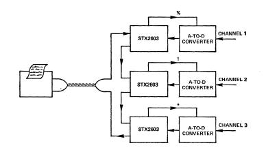
Figure 31. Many transmitters self-multiplexed on one series current loop. %, !, or \* interrogates the respective channels and transmits the data to the teletypewriter.
