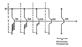
Figure 6. Binary-weighted current source transistors.
