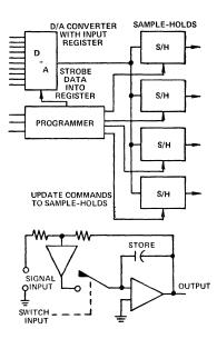
Figure 2. Sample-hold for each channel, with single fast, accurate D/A Converter. Multiplexing occurs by sampling each channel individually as its associated data appears on the input bus.
