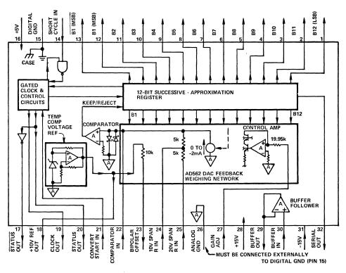
Figure 8. AD572 functional diagram & pinout.
