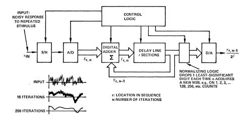
Figure 5. Waveform averaging by addition - basic scheme.
