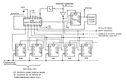
Figure 16. Logic diagram of successive-approximations ADC.
