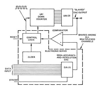
Figure 6a. Controlled-output DAC.
