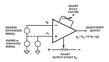
Figure 2. Differential instrumentation amplifier as a signal conditioner for data acquisition.
