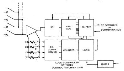
Figure 11. Switched-gain amplifier.
