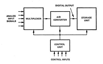
Figure 1. Data-acquisition system.
