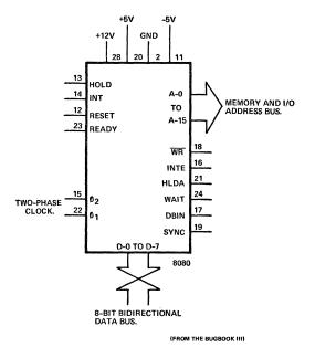
Figure 8. Functional diagram of connections to the 8080 microprocessor.
