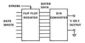
Figure 25. D/A converter with buffer register.
