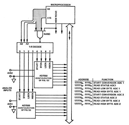
Figure 13. Interfacing multiple AD7550's to a microprocessor.
