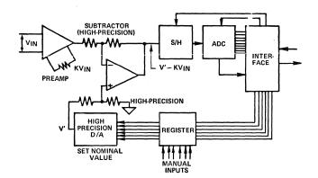
Figure 12. Use of high-resolution DAC to measure small deviations about a precisely-determined value.
