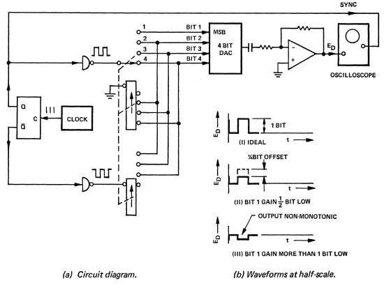
Figure 13. Simple DAC differential linearity tester.
