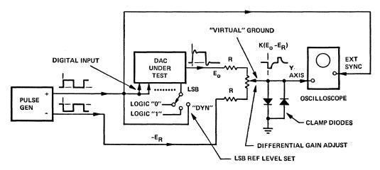
Figure 18. DAC zero and full-scale settling time measurement – virtual-ground method.
