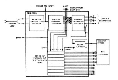
Figure 26. Block diagram of the SRX2605 serial receiver.
