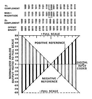
Figure 6. Ideal D/A conversion realtionship for 4-bit (3-bit-plus-sign) offset binary, 2's complement, sign-magnitude, 1's complement codes.
