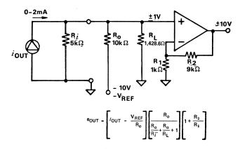
Figure 23. Non-inverting output from current-switching D/A converter.
