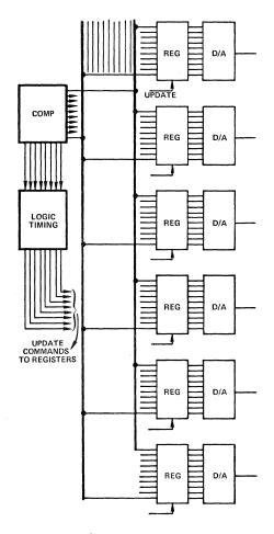
Figure 1. D/A Converter for each channel; parallel-word distribution.
