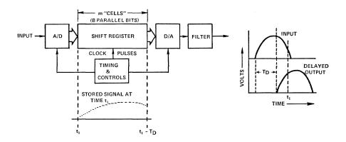
Figure 2. Parallel shift-register delay line.
