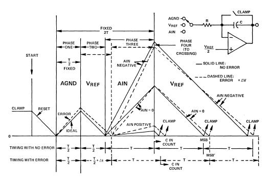
*Figure 34. Illustration of quad-slope principle: integrator output waveforms for positive, negative, and zero input – with and without error.*
