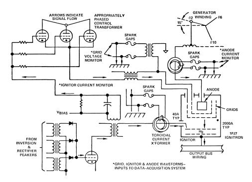
Figure 17a. Ignitron monitoring system.
