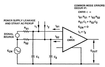
Figure 7. Common-mode and the difference signals due to line unbalance.
