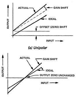
(b) Bipolar (offset binary) with offset and gain TC matched.
