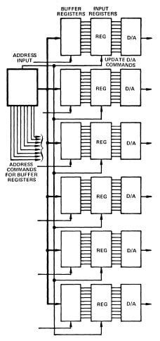
Figure 3. Simultaneous D/A updating.
