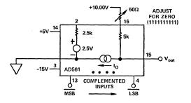
Figure 41. AD561 connected for unbuffered OV to +10V output, with  $5k\Omega$  output impedance. For this application, data inputs are negative true. Typical applications call for light load, e.g., with high-impedance devices or in null-seeking.
