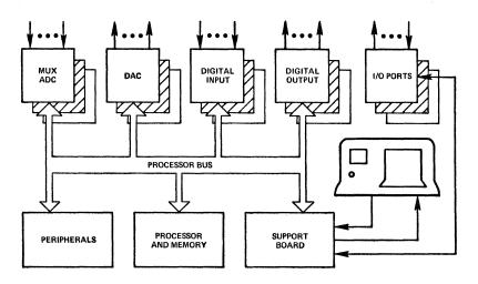
Figure 7. Block diagram of Macsym One system hardware.
