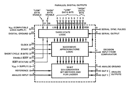
Figure 3. AD7570 10-bit A/D converter.
