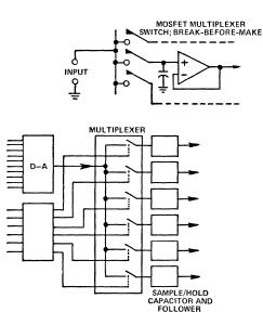
Figure 4. Multiplexing and sample-hold using multiplex switches.
