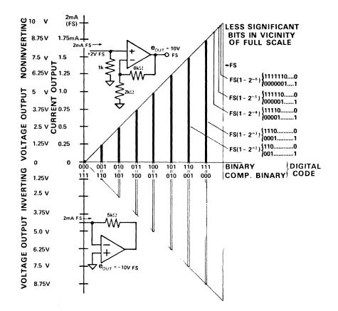
Figure 13. Ideal conversion relationships for 3 most-significant bits in positive reference unipolar D/I converter with noninverting and inverting amplifier connections, and binary vs. complementary binary codes.
