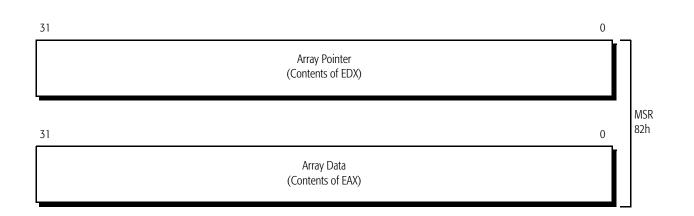
Figure 4-2. Array Access Register (AAR)
