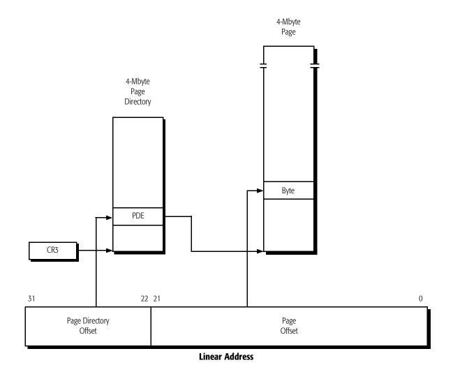
Figure 1-3. 4-Mbyte Paging Mechanism
