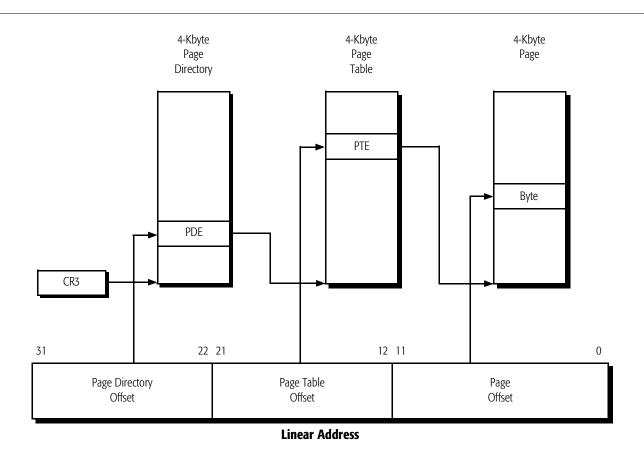
Figure 1-2. 4-Kbyte Paging Mechanism
