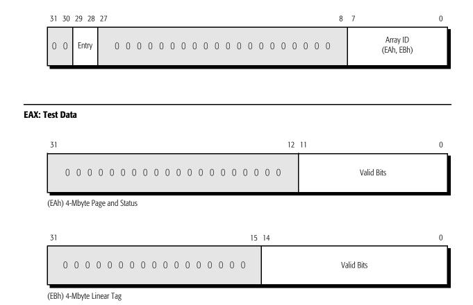
Figure 4-8. Test Formats: 4-Mbyte TLB
