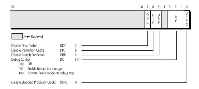
**Figure 4-1. Hardware Configuration Register (HWCR)**
