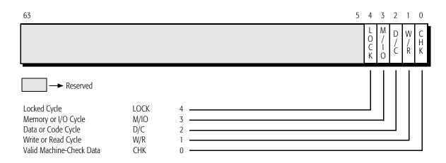
Figure 1-9. Machine-Check Type Register (MCTR)
