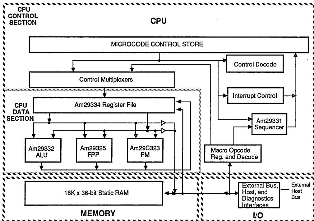
Figure 1-1. System Components
