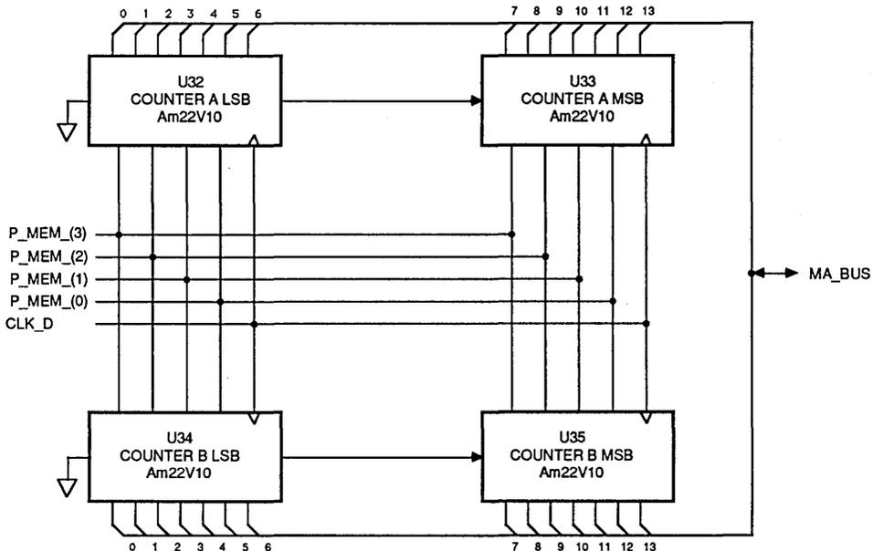
Figure 4-7. Memory Address Counters A and B
