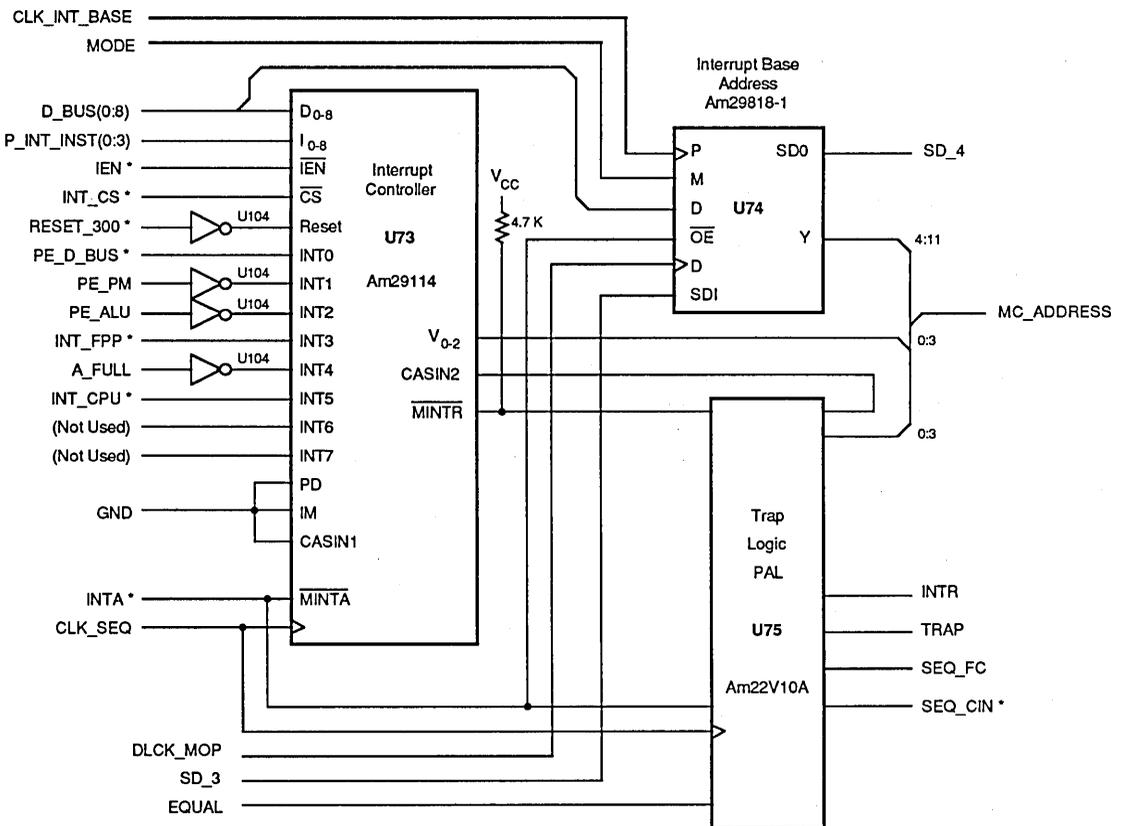
Figure 5-11. Interrupt and Trap Logic
