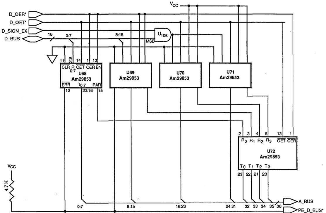
Figure 5-10. D Bus Transceiver
