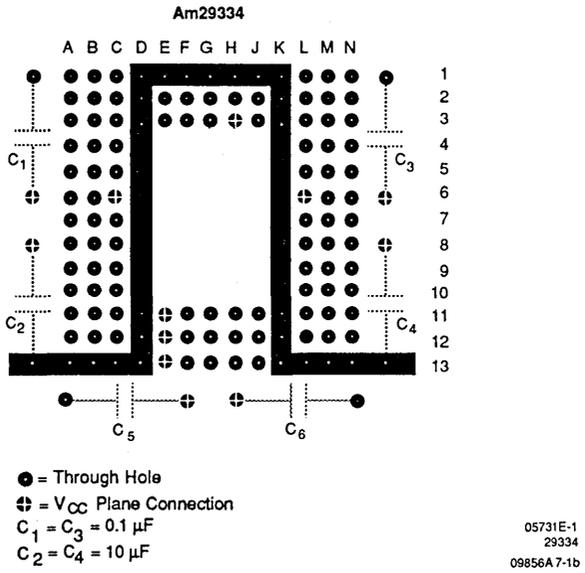
Figure 7-1b. Layout Recommendations for the V<sub>CC</sub> Plane
