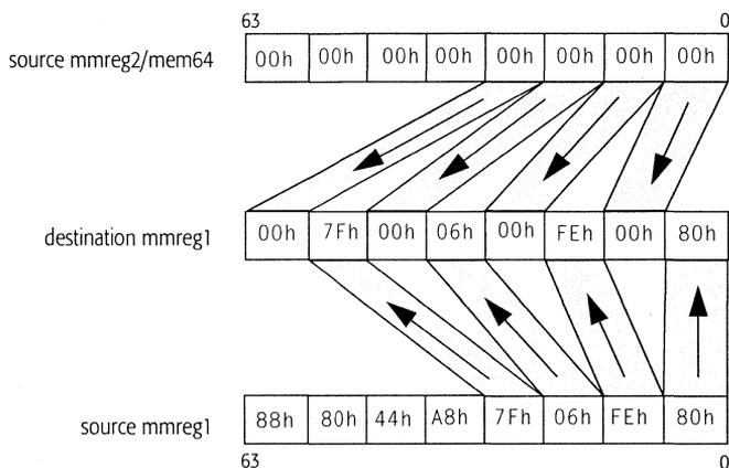
In the functional illustration of the PUNPCKLBW instruction, the 8-bit values from mmreg1 are stored in the low-order 8 bits of the 16-bit result. The mmreg2/mem64 source operand is set to all zero bits so it can provide zero fill in the high-order 8 bits of the 16-bit result. This is a method that can be used to expand unsigned 8-bit values into unsigned 16-bit operands for subsequent processing that requires higher precision.
