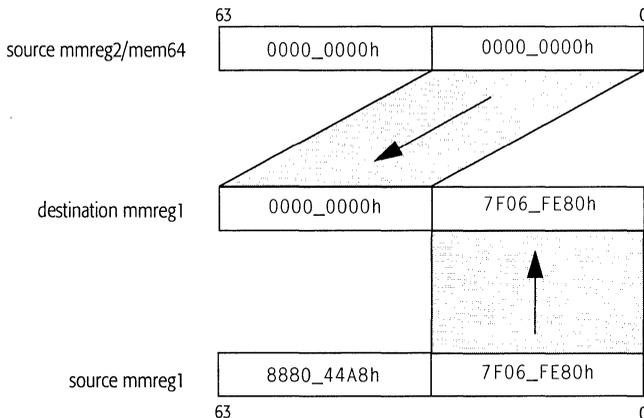
In the functional illustration of the PUNPCKLDQ instruction, the 32-bit value from mmreg1 is stored in the low-order 32 bits of the 64-bit result. The mmreg2/mem64 source operand is set to all zero bits so it can provide zero fill in the high-order 32 bits of the 64-bit result. This is a method that can be used to expand unsigned 32-bit values into unsigned 64-bit operands for subsequent processing that requires higher precision.
