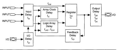
If the register is bypassed, the delay between the logic array and the output buffer is zero.
