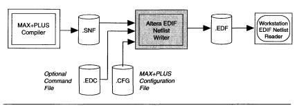
The EDIF output file may have one of two formats. The first format expresses all delays with special EDIF property constructs. The second expresses combinatorial delays with port-delay constructs and registered delays with path-delay constructs—a format that is especially useful for behavioral simulators. Figure 5 shows an example in both formats.
