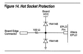
In some applications, boards are "hot-socketed" in the field. The circuitry shown in Figure 14 is recommended to ensure that latch-up-inducing levels are not applied to the EPLD under these conditions. Normally, this circuitry is required only if the EPLD has inputs tied directly to the edge connector. The diodes clamp the inputs at acceptable levels and the series resistor further limits the injection of current into the EPLD input and clamp diodes. This interface provides maximum protection.
