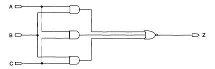
Step 2: Design an equivalent circuit with the MAX+PLUS Graphic Editor.
