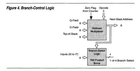
The address multiplexer provides the next-state address to the microcode memory. The next-state address can come from the Q-field, the D-field, or the top-of-stack. The selection is based on the instruction in the pipeline register and the condition of the zero flag from the counter.
