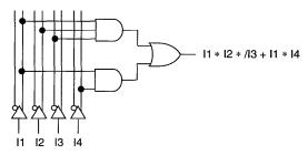
**Circuit C: Circuit B with 8-input AND gates in AND-array notation**
