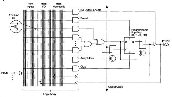
Figure 7. Detailed EPLD Macrocell Architecture
