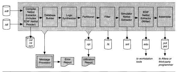
Compiler options simplify design processing and analysis. The user can specify up to two LMFs for the Compiler to use in processing EDIF Input Files (.edf), and can choose to create an EDIF Output File (.edo) for use with Valid Logic, Viewlogic, or other third-party simulation tools. Other options specify the degree of detail of the Report File (.rpt) that shows how EPLDs have been utilized and the target EPLD for the design.
