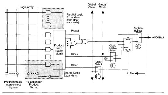
secondary inputs for either an additional XOR input or individual Clear, Preset, Clock, and Clock Enable logic functions for the flip-flops; or as logic expanders to assist the generation of complex logic functions.
