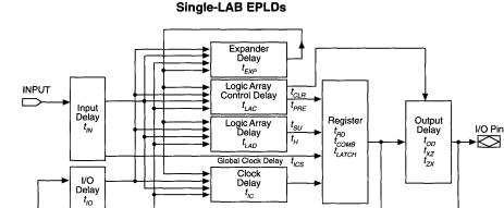
The timing models shown in Figure 6 can be used together with the internal timing parameters for a particular EPLD to derive timing information. External timing parameters are derived from a sum of internal parameters and represent pin-to-pin timing delays. Figure 7 shows the internal timing waveforms for these devices. Refer to *Application Brief* 75 for further information on MAX 5000 EPLD timing.
