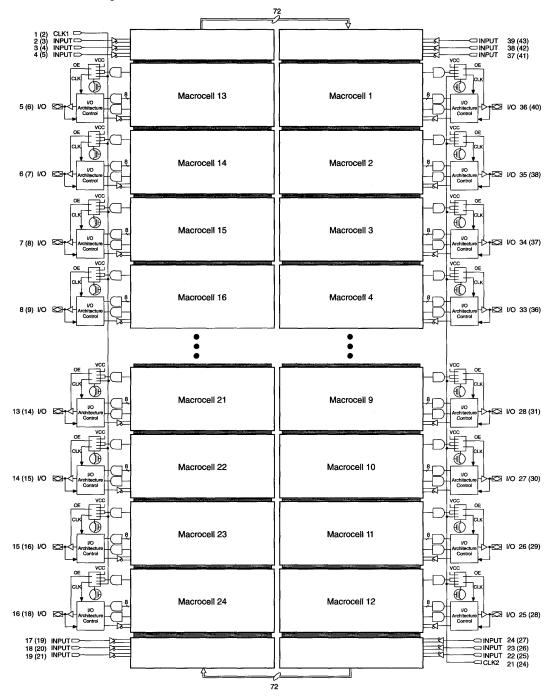
In the erased state, the true and complement of the AND-array inputs are connected to the product terms. An EPROM control cell is located at each intersection of an AND-array input and a product term. During the programming process, selected connections are opened, allowing any product term to be connected to the true or complement of an array input signal with the following results:
