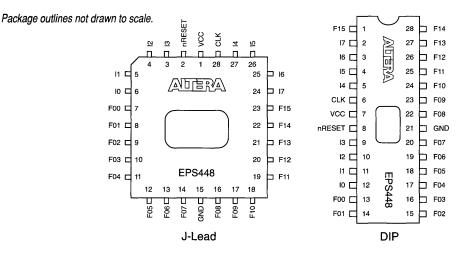
The on-chip EPROM of each EPS448 device (up to 448 words) is integrated with branch-control logic, a pipeline register, a stack, and a loop counter. This generic microcoded architecture can efficiently implement a broad range of high-performance controllers, from state machines to waveformgeneration applications.
