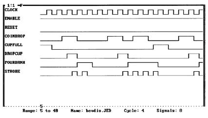
Figure 4. Virtual Logic Analyzer Output
