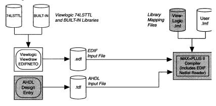
compiled. Symbols from the Valid Logic LSTTL library can be mapped to corresponding primitive and TTL functions in the MAX+PLUS II TTL MacroFunction Library with the Altera-provided Library Mapping File (.lmf) for Valid Logic users. Table 1 shows the primitive mappings and Table 3 shows the macrofunction mappings provided in this LMF.
