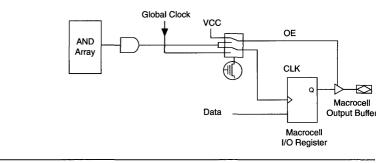
In Mode 0, the tri-state output buffer is controlled by a single product term If the output of the AND gate is high, the output buffer is enabled. If the output is low, the output buffer has a high-impedance value. In this mode the macrocell flip-flop is clocked by its global Clock input signal (CLK1 or CLK2). In the erased state, the OE/CLK Select multiplexer is configured to Mode 0.
