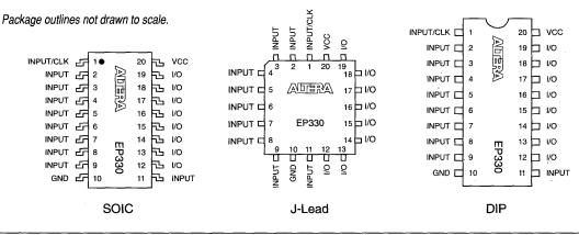
The EP330 EPLD can accommodate up to 18 inputs and 8 outputs. Each of the 8 macrocells contains a programmable-AND/fixed-OR structure that implements logic with up to 8 product terms. An additional product term in each macrocell controls Output Enable.
