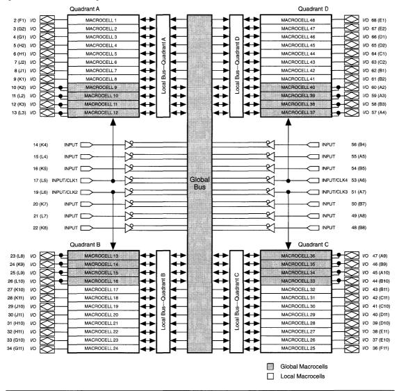
Array clock signals allow flip-flops to be configured for positive- or negativeedge-triggered operation. When global Clocks are used, the flip-flops are triggered by the positive edge, i.e., data transitions occur on the rising edge of the clock. 2
