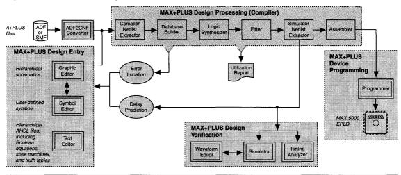
The PLDS-MAX Development System includes MAX+PLUS software, al hardware required to program MAX 5000 EPLDs, and device samples PLS-MAX is a software-only package. See "Package Contents" later in this data sheet for more information.
