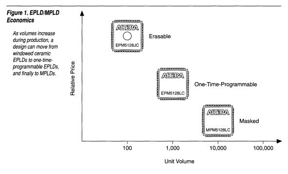
The EPLD-to-MPLD conversion is handled by Altera so that no redesign effort is required. Altera guarantees that the MPLD meets the worst-case AC and DC parameters of the original EPLD design. In addition, Altera automatically generates test vectors with over 95% fault coverage.
