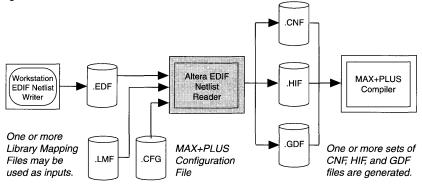
The Altera EDIF Netlist Reader can convert any EDIF 200 netlist with the following characteristics:
