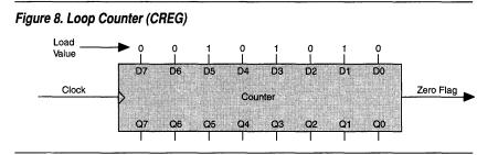
The CREG is loaded or decremented on the leading edge of the clock. It will not decrement once it reaches zero, thereby preventing roll-over. A zero flag indicates when the counter has reached zero. This flag is used with the LOOPNZ command to control program flow. (See "Instruction Set" later in this data sheet.) Single-instruction delay loops are easily constructed, and nested loops or delays of arbitrary length may be generated in combination with the stack.
