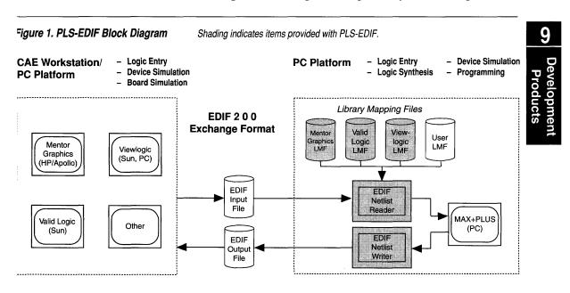
PLS-EDIF (Bidirectional EDIF Netlist Interface to MAX+PLUS Software) allows designers to enter and verify logic designs for Altera MAX 500C EPLDs with third-party CAE tools. The EDIF 2 0 0 netlist exchange format provides a two-way bridge between MAX+PLUS and third-party schematic capture and simulation tools. PLS-EDIF runs on an IBM PS/2, PC-AT, or compatible computer.
