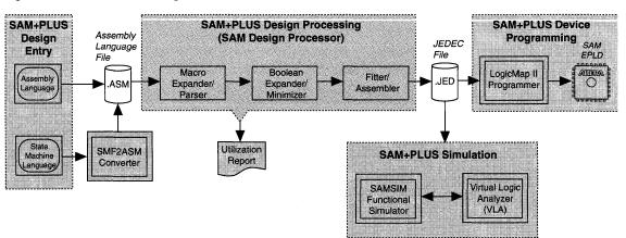
Figure 1. SAM+PLUS Block Diagram
