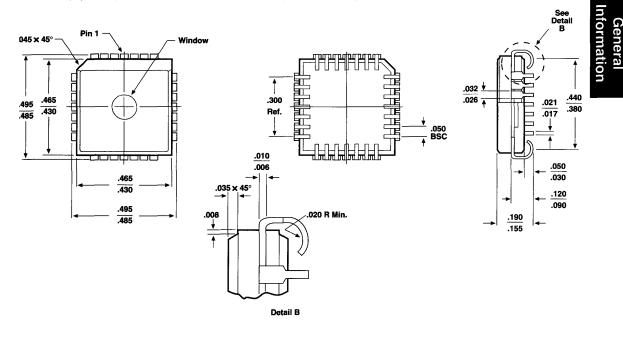
**!8-Pin Plastic J-Lead Chip Carrier (PLCC)**
