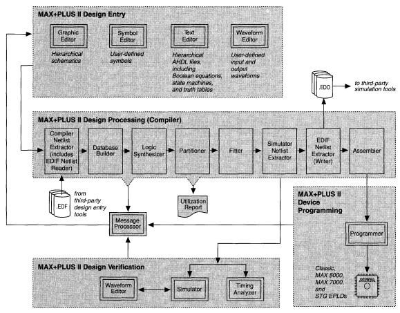
to create large system-level designs. The Partitioner lets the user specify speed-critical paths for optimum EPLD selection and design placement.
