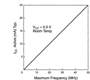
Figure 4. MP1810 I<sub>CC</sub> vs. Frequency
