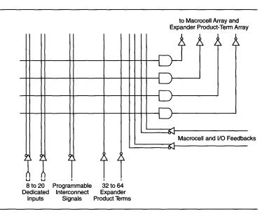
Expanders are fed by all signals in the LAB. One expander may feed all macrocells in the LAB or multiple product terms in the same macrocell. Since expanders also feed the secondary product terms of each macrocell, complex logic functions can be implemented without using additional macrocells. Expanders can also be cross-coupled to build additional flip-flops or latches.
