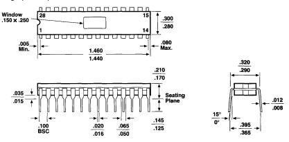
28-Pin Plastic Dual In-Line Package (PDIP)
