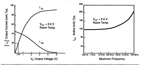
Figure 13. EPM5032 Output Drive Characteristics and  $I_{CC}$  vs. Frequency
