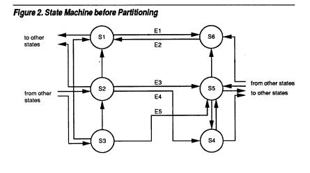
The states are connected by directional arrows, marked with the symbolic labels **E1** to **E5**, that show possible transitions to and from states. These labels represent arbitrarily complex or simple equations, which are normally functions of state machine inputs that allow the state machine to respond to external events.
