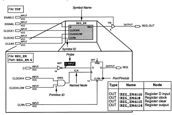
Figure 2. Node Names in a Hierarchical Design
