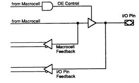
state machines or bus-oriented functions) are easily accommodated by this programmable I/O control block.
