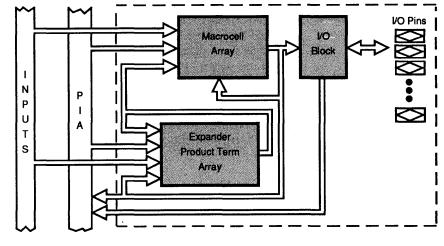
without the waste associated with fixed product-term architectures. Thus, PAL or PLA devices are easily integrated into MAX EPLDs. The outputs of the macrocells feed the decoupled I/O block, which consists of a group of programmable tri-state buffers and I/O pins. In the EPM5064, EPM5128, EPM5130, and EPM5192, multiple LABs are connected by a Programmable Interconnect Array (PIA).
