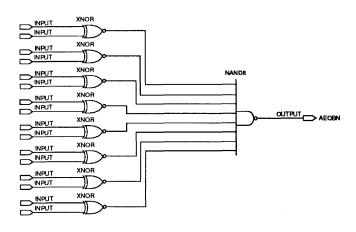
The best location for a **SOFT** buffer may not be obvious. Although the Compiler error message specifies an error location, the identified node name indicates the output of the complex expression, which is usually not the correct location for a **SOFT** buffer. To find the best location, the logic feeding the node must be analyzed to determine the cause of the expression's complexity.
