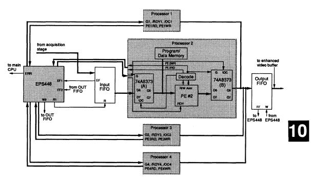
The EPS448 EPLD is also a highly integrated coefficient generator for a variety of DSP algorithms. In addition, the device's exact timing capabilities make it popular in the video output stages of the DSP imaging system.
