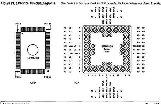
The EPM5130 EPLD is available in a windowed ceramic pin grid array (PGA) or 100-pin windowed ceramic or plastic one-time-programmable quad flat pack (QFP) package.
