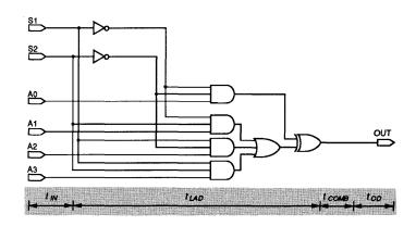
The propagation delay from input pin to I/O pin is the sum of the input delay, logic array delay, combinatorial buffer delay, and output delays:  $t_{IN} + t_{LAD} + t_{COMB} + t_{OD}$ . This worst-case delay is also known as  $t_{PD1}$  (from input pin to output pin) or as  $t_{PD2}$  (from I/O pin to output pin). The maximum  $t_{PD1}$  and  $t_{PD2}$  values are shown in the individual MAX EPLD data sheets, or may be determined with the following equations.
