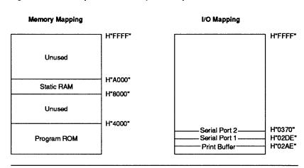
Figure 1. 16-Bit Microprocessor Memory and I/O Space
