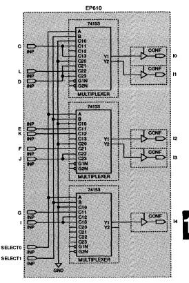
EPLD (**I5** to **I7**). The other nine inputs are routed through an EP610 EPLD and multiplexed down to the five remaining input pins (**I4** to **I0**). Two outputs from the EPS448 EPLD (**SELECT0** and **SELECT1**), which depend on the current state, feed the multiplexer select inputs on the EP610 and direct the correct set of system signals to the EPS448 inputs.
