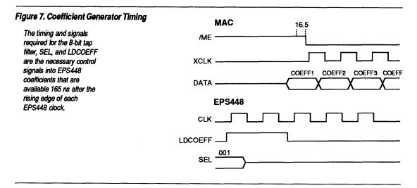
The EPS448 EPLD has 448 microcode addresses, each containing a 36-bit word that consists of 20 internal control bits and 16 output bits. As a result, the EPLD contains a  $448 \times 16$  PROM and a stack that can implement a 448-way branch in only 2 clock cycles. The EPS448 EPLD can thus store and quickly obtain access to coefficient tables of varying sizes to implement multiple algorithms.
