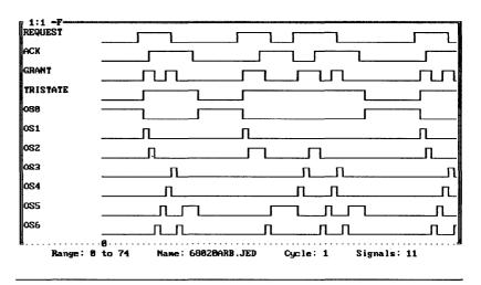
Figure 8. VLA Screen for Bus Arbiter Design
