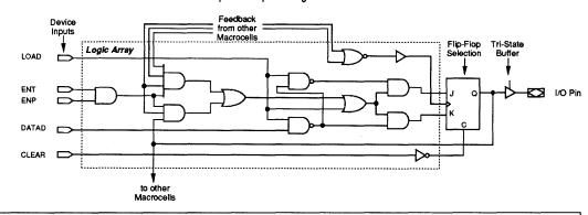
This figure shows a typical logic function implemented in a single macrocell. Each EP1800-series macrocell can accommodate up to 40 equivalent gates. EP1800-series EPLDs have 4 identical quadrants, each containing 12 macrocells. Internal bus structures in these EPLDs feed input signals into the macrocells. Macrocell outputs drive the external pins and internal buses.
