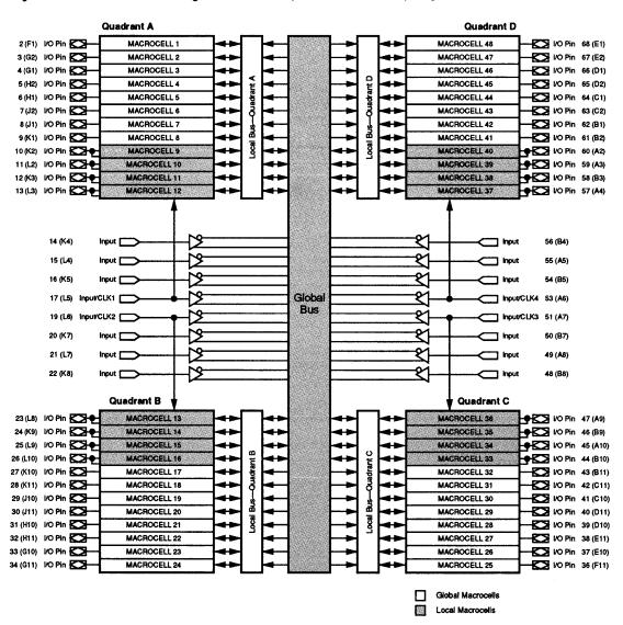
Figure 2. EP1800-Series Block Diagram Numbers in parentheses are for PGA packages.
