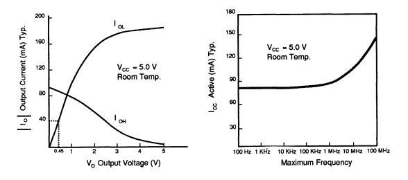
Figure 10. EPM5016 Output Drive Characteristics and I<sub>CC</sub> vs. Frequency
