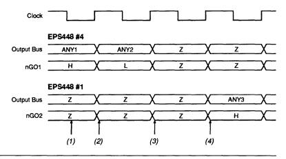
versa. During this clock period, the control lines (**nG01** to **nG04**) float unless they are pulled up by the resistors.
