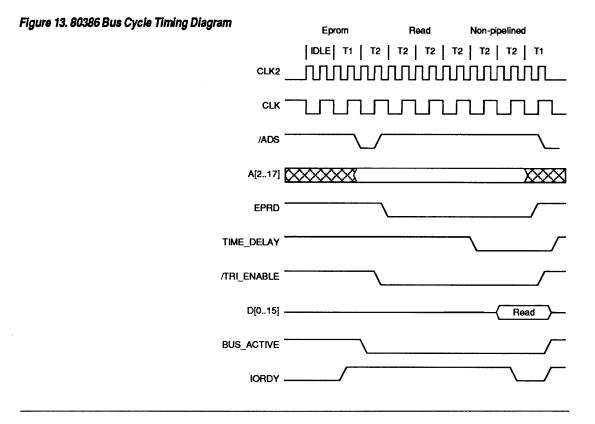
The EPROM output signals become valid 200 ns after an address is placed on the address signals. To activate the **/READY** signal, the number of wait states required must include the EPROM address-to-valid delay *plus* the latch clock-to-output delay *minus* one state machine cycle. Thus, the total delay required, in nanoseconds, is:
