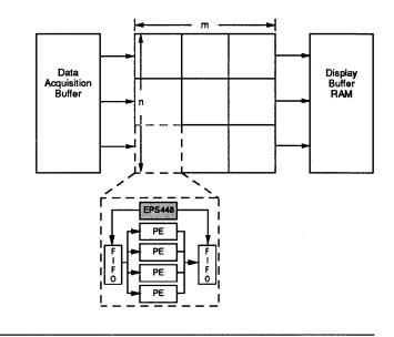
The need for processor element speed has led to advances in processors dedicated to DSP applications, such as the TMS320 family. Careful system data flow design is just as critical to system performance, particularly in a heavily pipelined system. Ideally, data should flow "automatically" through the system, without involving the PEs. By minimizing the housekeeping overhead on the processor elements, this method maximizes useful imaging cycles throughout the system.
