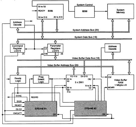
These activities are performed independently of the main microprocessor, freeing it up for other tasks. These other tasks fall into two general categories: controlling bus transfers between elements (registers, ALU, RAM, etc.) and sequencing 2901 ALU computations that generate the pixel addresses for drawing the circle.
