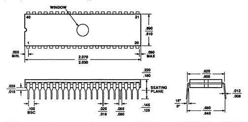
40-Pin Plastic Dual In-Line Package (PDIP)
