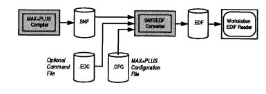
The EDIF output file may have one of two formats. The first format expresses all delays with special EDIF property constructs. The second expresses combinatorial delays with port-delay constructs and registered delays as path-delay constructs—a format that is especially useful for behavioral simulators. Both formats are shown in the example in Figure 5.
