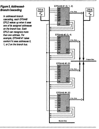
A single EPS448 EPLD can have several addresses assigned to it, with each address corresponding to a different starting location in its microcode. Thus, a single EPLD can contain more than one block of independent states. In such a case, each address on the branch bus corresponds to a block of states within an EPLD.
