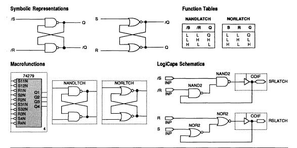
Figure 4. SR Latch Implemented in an Altera Design File
