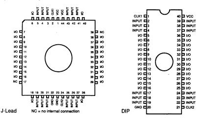
EP900-series EPLDs use sum-of-products logic that consists of a programmable-AND/fixed-OR structure. These EPLDs accommodate combinatorial and sequential logic functions with up to 36 inputs and 24 outputs.
