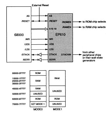
Figure 5 shows the logic schematic for the EP610. The design provides two chip-select signals, one for 256 Kbytes of DRAM (**RAMENL**) and the other for 64 Kbytes of ROM (**ROMENL**). The EP610 asserts **DTACK** one clock cycle after ROM is selected, providing the ROM with two wait states (**UAIT2**), two clock cycles after a RAM read (**UAIT4**), and three clock cycles after a RAM write (**UAIT6**).
