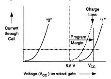
Figure 11 illustrates the concept of cell margin. As mentioned earlier, EPROM arrays depend on cell threshold shifts for correct operation. Zero and One I-V characteristics for the EPROM cell are shown. Program margin is a measure of the spread between the actual device threshold and the minimum required device threshold for correct operation.
