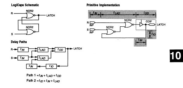
Figure 8. Cross-Coupled NOR Gates
