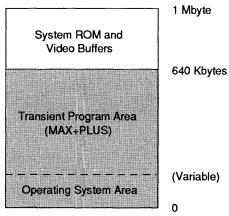
Memory ranging from 640 Kbytes up to 1 Mbyte is used for system ROM (device handlers) and expansion board buffers. DOS and programs that run under DOS (e.g., MAX+PLUS) occupy the lower 640 Kbytes of conventional memory. This area is further divided into an operating system area and a transient program area (TPA).
