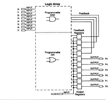
array. Each of the AND gates is fed by 8 to 12 input pins and feedback signals, plus their complements. The OR array allows logical ORing of any of the AND terms in the array. Typically, 8 to 12 programmed OR terms feed either feedback combinatorial buffers, feedback registers, or output pins.
