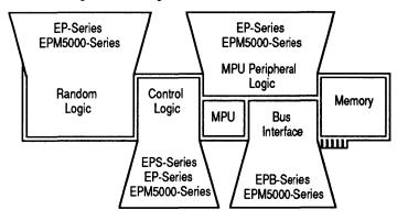
EPLDs can be used to integrate complete printed circuit boards of TTL, PAL, and FPGA devices into a single package. EPLDs are also valuable for prototyping high-density custom devices, which enables designers to test markets and evaluate systems before committing to expensive engineering development cycles and tooling charges. For most of today's applications, EPLDs not only ensure faster time-to-market, but also provide a lower total cost than custom ASIC solutions.
