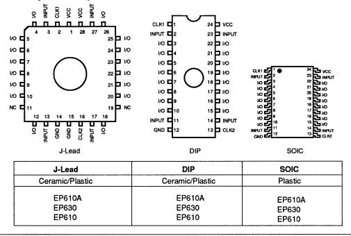
The CMOS EPROM technology in EP600-series EPLDs can reduce active power consumption to less than 40% of the power required by equivalent bipolar devices, without losing speed. This reduced power consumption makes the EP600-series EPLDs highly desirable for a wide range of applications. Moreover, these EPLDs are 100% generically testable and can be erased with UV light. Designs and design modifications can be implemented quickly, eliminating the need for post-programming testing.
