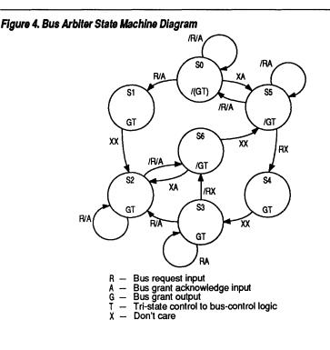
Three signal lines on a 68020 bus—**REQUEST**, **GRANT**, and **ACKNOWLEDGE**—define the handshake required to arbitrate bus exchanges between multiple bus masters. **S0** represents the "normal," active state of the processor; **S1** and **S2** correspond to the grant phase; **S5** and **S6** to the acknowledge phase; and **S3** and **S4** to the arbitration phase if requests are pending at the end of the current bus exchange.
