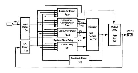
Figure 4 shows the timing model for multiple-LAB devices. Following is a list of these microparameters and examples of how to predict timing delays with equations that use them.
