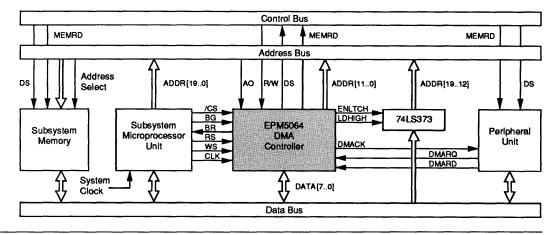
Figure 2 shows the timing associated with the DMA control signals. A custom-designed DMA controller in an EPM5064 can improve performance of the peripheral subsystem by providing faster data transfers than are possible with the MPU alone. Using a DMA controller also frees the MPU to perform other tasks.
