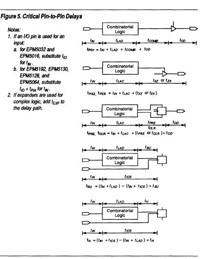
Critical pin-to-pin delay calculations are shown in Figure 6. The calculations used to derive these values from the microparameters listed in the MAX EPLD data sheets are shown for each path. These calculations assume that a dedicated input pin is used.
