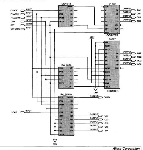
Integration of these 3 PALs plus the 2 discrete counters required 29 macrocells and 29 expanders. Less than 90% of the EPM5032 is used, so there is room left to implement additional logic.
