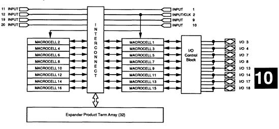
The macrocell array contains 16 macrocells (see Figure 2). Each macrocell has a programmable-AND/fixed-OR array and a configurable register that provides D, T, JK, SR, or flow-through latch operation with independent programmable clock options. Each macrocell also contains 3 product terms for logic implementation. If necessary, the expander product-term array can supply up to 32 additional product terms. Each expander product term can be used and shared by any of the macrocells.
