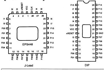
The EPS448 EPLD is available in 28-pin, 300-mil windowed ceramic dual in-line packages (DIPs) and in 28-pin ceramic J-lead chip carriers (JLCCs). One-timeprogrammable plastic J-lead (PLCC) versions of the EPS448 EPLD are also available for volume production. See Figure 1.
