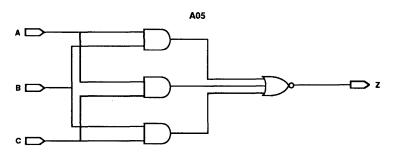
Step 2: Design an equivalent circuit with the MAX+PLUS Graphic Editor.
