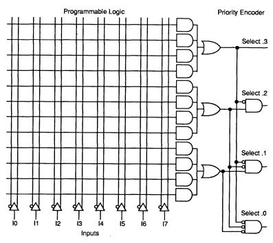
The EPS448 EPLD is designed so that the number of available product terms is always sufficient for a design. Prioritization provides an effective product-term count of more than 12 per location. A tradeoff between the number of product terms and the number of possible branches can be made simply by placing identical state information in 2 locations, as shown in Figure 6.
