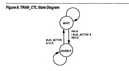
The AHDL file describing **TRAN\_CTL**, which is a single-bit state machine called **tran\_en**, is shown in Figure 9. When a non-pipelined bus cycle is executed with the statement **na & !bus\_active**, the 80386 control signals are read by **tran\_en** to determine whether the transceiver needs to be enabled. The enable is released when the bus cycle is completed with the statement **bus\_active & clk**.
