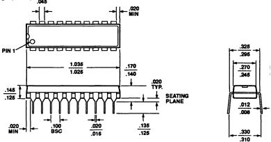
20-Pin Plastic J-Lead Chip Carrier (PLCC)
