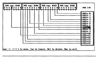
Address decode chip-select ranges may be entered in either I/O, memory, or binary format (see Figure 2).
