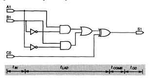
where S1 is the output of macrocell 21 (\_MC021), which contains combinatorial logic. The combinatorial logic, MCELL(\_EQ026 \$ C0), represents the XOR of the intermediate equation (\_EQ026) and the carry-in (C0). In turn, \_EQ026 represents logic equivalent to the XOR of inputs, B1 and A1. See Figure 8.
