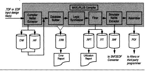
The Compiler offers several options to customize the processing and analysis of a design. The user can set the degree of detail of the Report File as well as the maximum number of errors to be detected before processing halts. The user can also choose whether to extract a netlist containing postsynthesis timing information.
