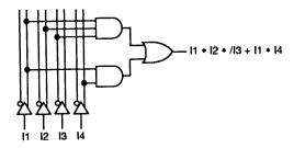
The  $2 \times 8$  AND-array of circuit III can produce any Boolean function of four variables (provided only two product terms are required) when expressed in sum-of-products form. Any Boolean expression—no matter how complex—can be written in sum-of-products form. Outputs of the two AND gates in Figure 5 are called product terms (or p-terms).
