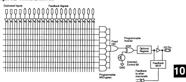
When modelling EPLD timing, the concept of "gate delay" is not a useful measure. The EPLD logic array contains *n*-input AND gates called product terms (n is the number of connections). Depending on the logic implemented, a single product term may represent one to several gate equivalents.
