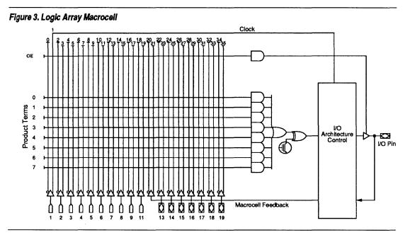
The EP330 block diagram is shown in Figure 4. The internal architecture of this device has a sum-of-products (AND/OR) structure. Inputs to the programmable-AND array come from the true and complement signals of the dedicated input pins, and the true and complement forms of the 8 feedback signals that come from the I/O architecture control blocks. The 36-input AND array has 72 product terms distributed equally among the 8 macrocells. Each product term represents a 36-input AND gate.
