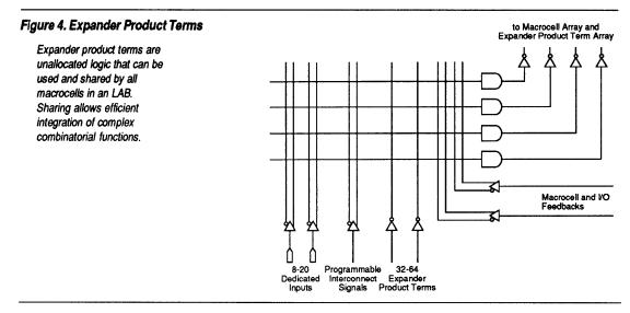
Expanders are fed by all signals in the LAB. One expander may feed all macrocells in the LAB or multiple product terms in the same macrocell. Since expanders also feed the secondary product terms of each macrocell, complex logic functions can be implemented without using another macrocell. Expanders can be cross-coupled to build additional flip-flops or latches.
