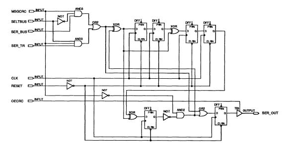
Integration is simplified with MAX+PLUS. Each of the three source files is compiled separately with the MAX+PLUS Compiler, and the automatically generated symbols that represent each module are entered with the MAX+PLUS Graphic Editor. Appropriate connections are made between the symbols to complete the design, and the final schematic is then submitted to the MAX+PLUS Compiler (see Figure 13). The PLS105A, PLS157, and PLS167A designs all fit into one EPM5032 (see Figure 14).
