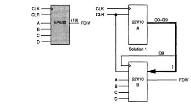
The logic design for the EP630 EPLD is entered, compiled, verified, and programmed with the Altera Programmable Logic User System (A+PLUS). Design entry is simple with LogiCaps schematic capture. LogiCaps provides access to over 100 Altera-supplied TTL macrofunctions (see Figure 2), which speed up design entry for designs such as this programmable frequency divider, allowing the designer to enter and connect the appropriate TTL macrofunctions. The Altera Design Processor provides
