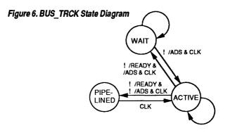
The AHDL description of **BUS\_TRCK** is shown in Figure 7. **BUS\_TRCK** has two output signals: **bus\_active** and **pipe\_active**, of which only **bus\_active** is used in the top level of the design. The **bus\_active** signal
