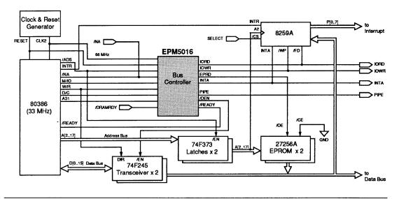
The 80386 halts processing to allow wait states to be added into the bus cycle when the signal **/READY** is high. (The slash (/) indicates an active-low signal.) The EPM5016 bus controller tracks each bus cycle operation and causes **/READY** to go high when wait states are needed. For example, read operations from 200-ns EPROM memory in 33-MHz systems require 14 wait states.
