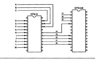
With input encoding, an EP610 EPLD compresses 13 system inputs (A to M) down to 5 inputs to the EPS448 EPLD (10 to 14). Three input pins (15 to 17) are still available for general-purpose use.
