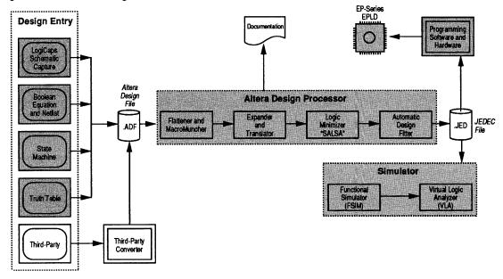
hardware is not included in PLS-SUPREME. Refer to the *PLCAD-SUPREME* or *PL-ASAP* data sheets for more information about products that include hardware.) PLS-SUPREME software runs on an IBM PS/2, PC/AT, or compatible computer and offers the most comprehensive support available for Altera's classic EPLDs.
