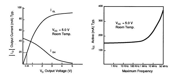
Figure 19. EPM5128 Output Drive Characteristics and I<sub>CC</sub> vs. Frequency
