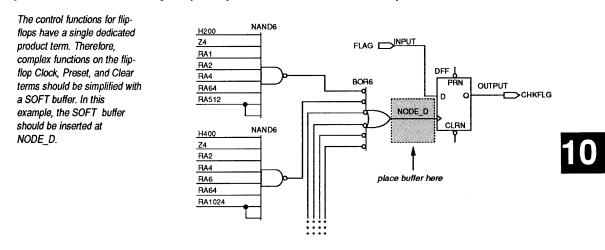
The following suggestions for placing **SOFT** buffers should be used to prevent and resolve compilation problems. Not only can fitting problems be avoided if these suggestions are followed, but often a more efficient fit will result, allowing additional logic to be integrated into the target EPLD. The following four steps should be taken in order:
