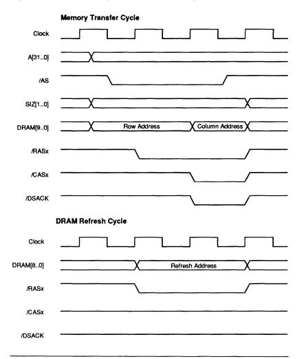
Figure 4. Memory Transfer Cycle and DRAM Refresh Cycle
