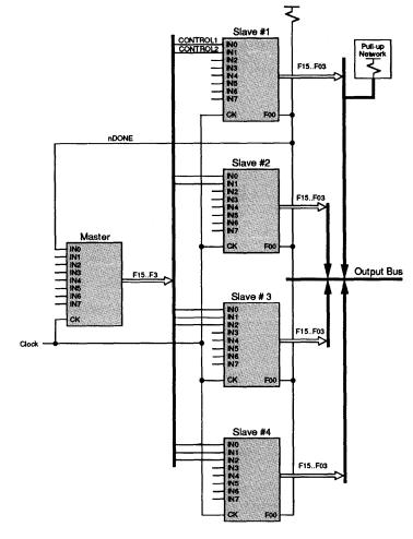
Figure 10 shows the timing associated with the master/slave configuration. Slave #1 originally has control of the output bus. It signifies that it is done by pulling **nDONE** low. The Master responds by initiating the Slave #2 machine, which then takes over the output bus. (The output bus is undefined for a single clock cycle.)
