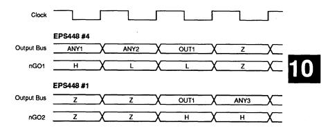
Each of the EPS448 EPLDs must have its own design file (with the extension .**ASM** or .**SMF**). A segment of the code used in EPS448 #1 is shown in Figure 4. While the machine is inactive, it remains in **IDLE** with the outputs disabled. When it receives an active-low **nGO1** signal from pin **1NO**, it jumps to the label **START**, takes control of the output bus, and holds **nGO2** to **nGO3** high, preventing the other EPLDs from competing for control of the output bus.
