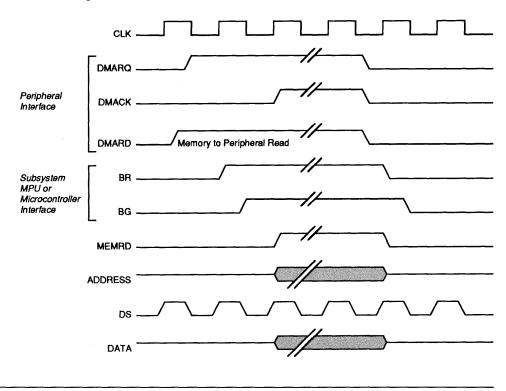
To start the DMA process, the MPU must first select and initialize the DMA controller; then it must write the starting and ending addresses and the control information to the controller. The control data indicates whether the transfer addresses should be incremented or decremented.
