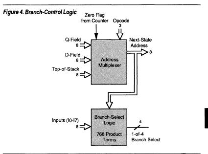
The address multiplexer provides the next-state address to the microcode memory. The next-state address can come from the Q-field, the D-field, or the top-of-stack. The selection is based on the instruction in the pipeline register and the condition of the zero flag from the counter.
