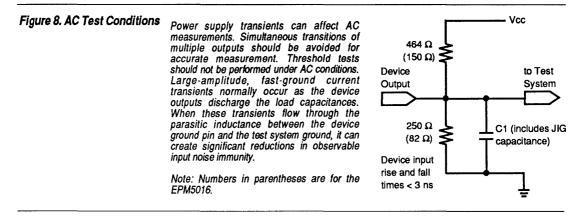
Test programs may be used and then erased during early stages of the production flow. This facility to use application-independent, general-purpose tests is called generic testing and is unique among user-configurable logic devices. EPLDs also contain on-board logic test circuitry to allow verification of function and AC specifications once they are packaged in windowless packages.
