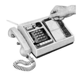
Fig. 8-Removal of 1B Cartridge
