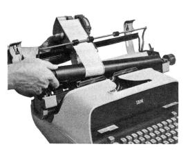
Fig. 9—Placing 1B Cartridge in Typewriter
