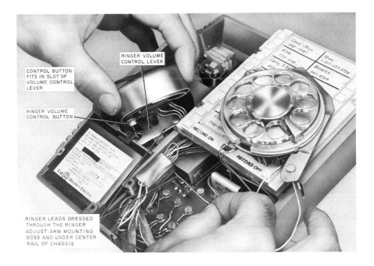
Fig. 8—Ringer Being Installed in 960A01M Chassis With Dial Rotated Onto Memory and Shield Removed
