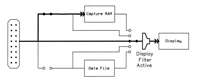
Figure 7-2 Connection Diagram – Display Filters Activated
