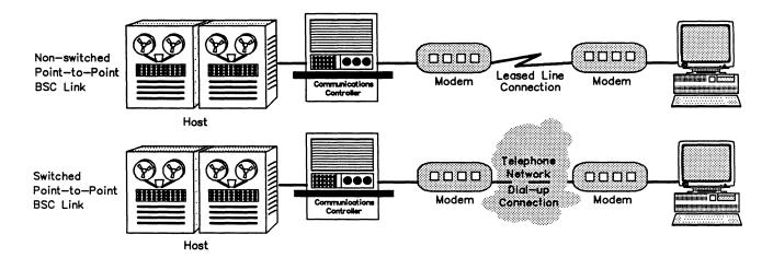
Figure A-1 Point-to-Point Configuration
