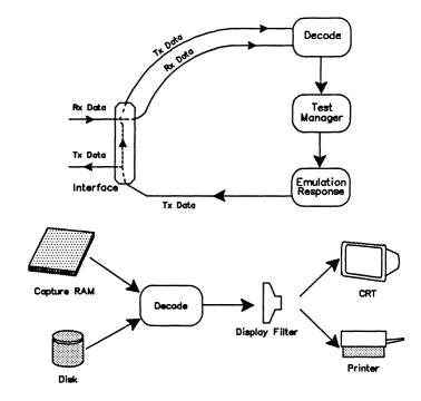
Figure 10-2 BSC Emulation Data Flow Diagram – Offline Processing
