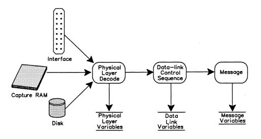
Figure 8-1 BSC Data Flow Diagram - Decode
