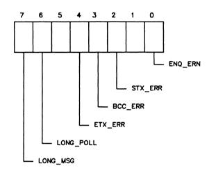
Figure 11-1 ERROR-GEN Bit Position
