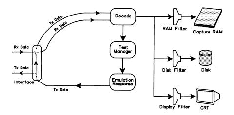
Figure 10-1 BSC Emulation Data Flow Diagram - Live Data
