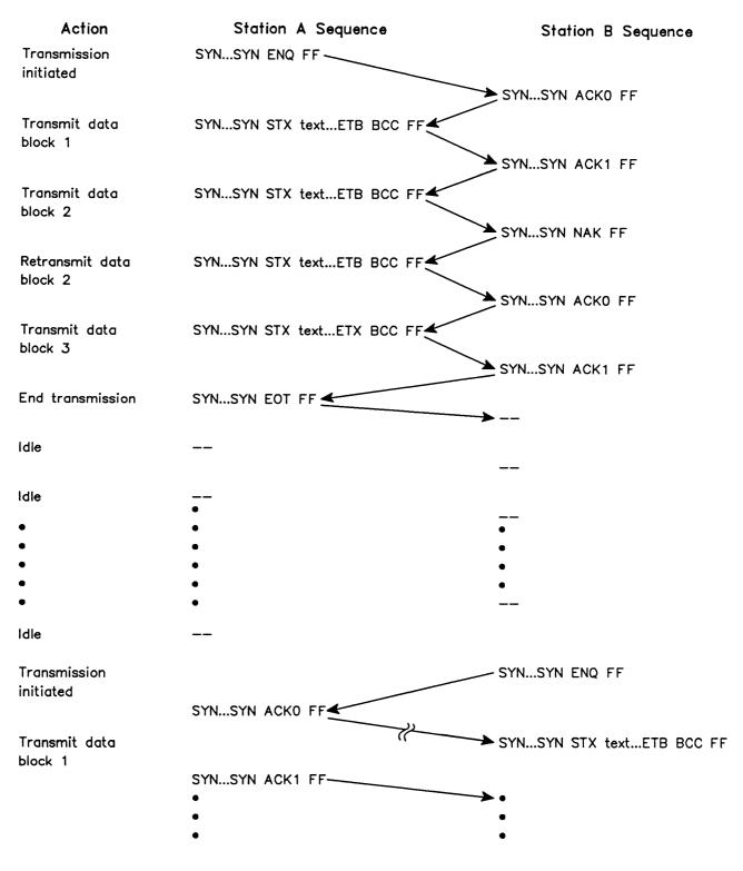
Figure A-3 Point-to-Point Setup and Transmission
