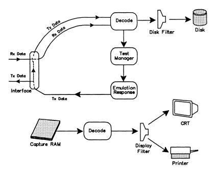
Figure 10-3 BSC Emulation Data Flow Diagram - Freeze Mode
