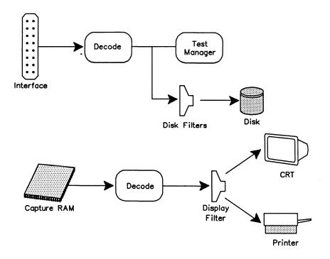
Figure 3-3 BSC Monitor Data Flow Diagram - Freeze Mode
