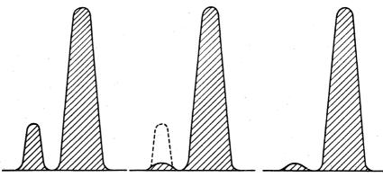
With Selective Switch in XTAL Sharp position identify the weaker amplitude—Tune Receiver to the weaker. Adjust phasing control carefully until this weaker amplitude is reduced to a minimum. Retune Receiver to the stronger amplitude and then adjust pitch control until you get note most pleasing to copy.
