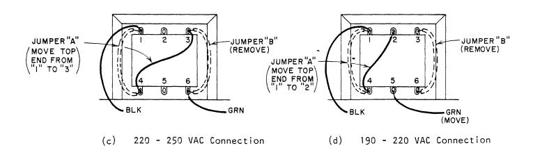
Figure 11. Power Transformer Voltage Tap Connections
