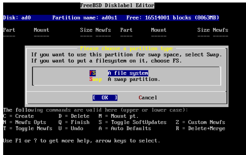
Figure 2-22. Choisir le type de la partition racine
