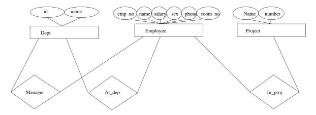
Figure 1.1: Company Entity-Relation Diagram
